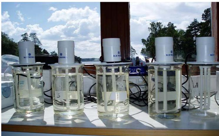
**Figure 11.** The jar test equipment.
