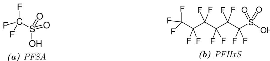
**Figure 4:** Structural formulas of two PFSAs.
