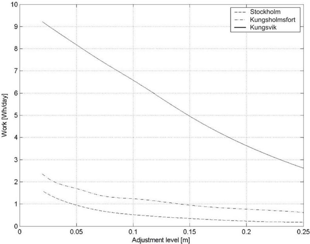
**Figure 7.2** The graph shows how the power need of the regulation system for the buoy varies depending on the predetermined limit of adjustment for the three locations; Stockholm, Kungsholmsfort and Kungsvik. The work per day is the average work derived from the total work over one calendar year.
