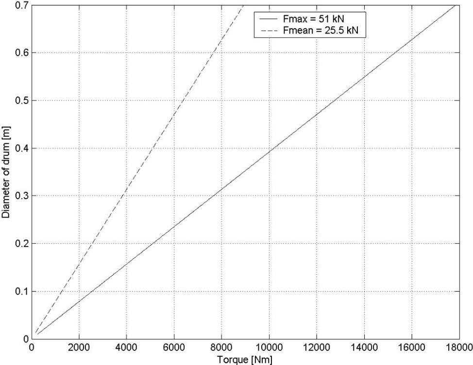
**Figure 7.3** The influence of the drum diameter on the torque exerted on the drum axle.  $F_{max}$  and  $F_{mean}$  are both calculated from 5.1.1-3
