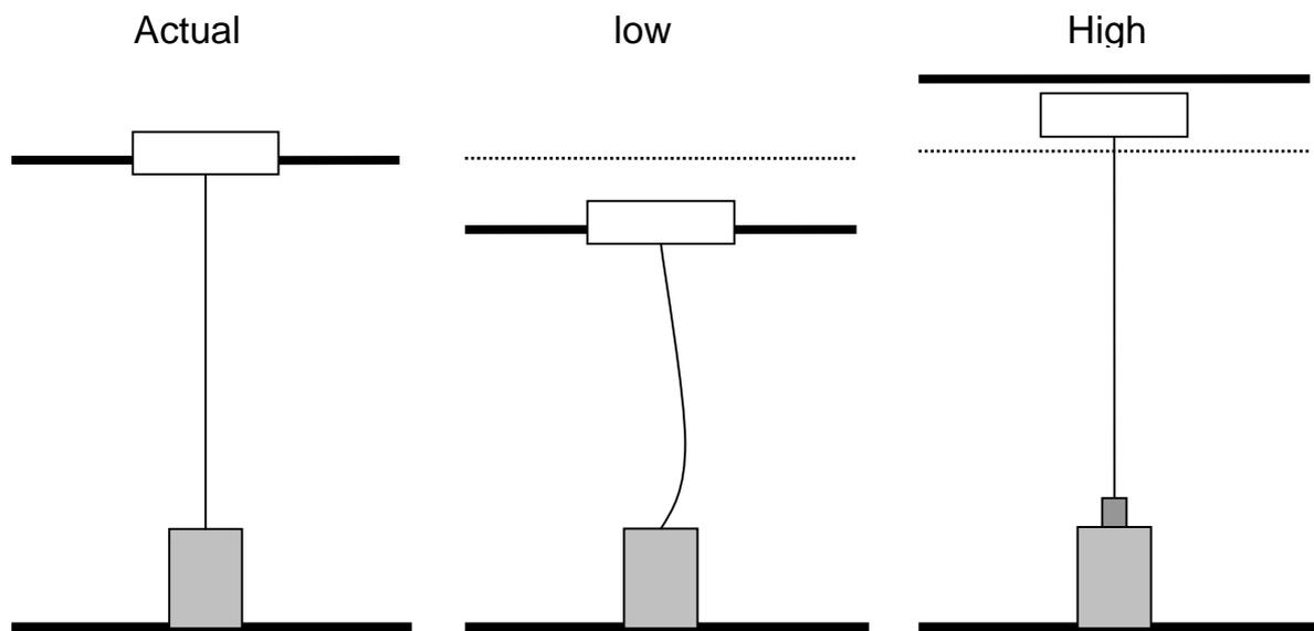
**Figure 1.2** A simple illustration of the problems due to water level change. When water levels fall below normal levels the line goes slack and there occurs a poorer energy conversion. Energy conversion is also lessened when water levels rise too high pulling the alternator to its maximum position and thereby inhibiting normal movement of the alternator.
