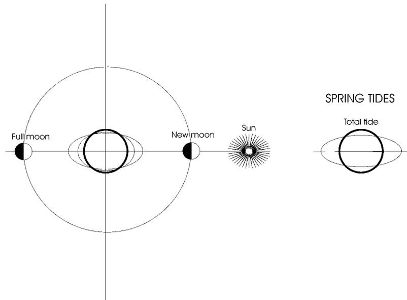
**Figure 2.4a** Example of the occurrence of spring tides (figure is not at scale).
