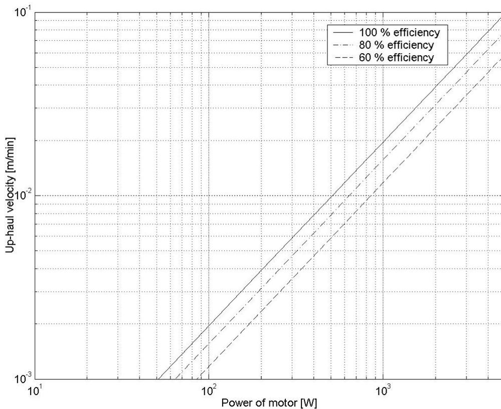
**Figure 7.6** Description of the up-haul velocities influence on the choice of motor at different efficiencies.
