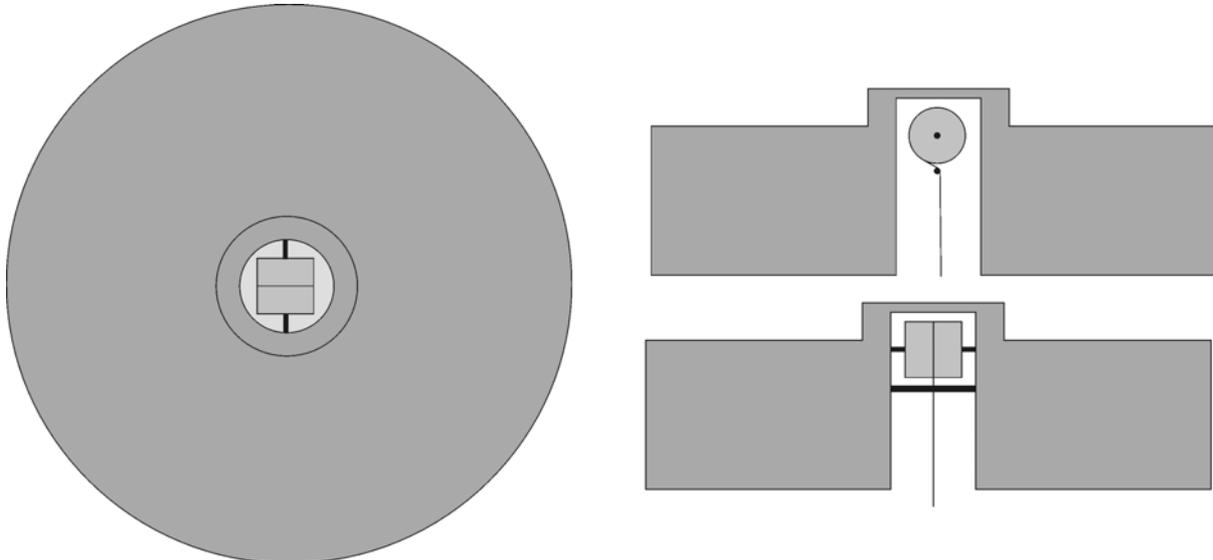
**Figure 5.8** A hollow buoy with a raised head and guide wheel. The raised head increases the distance between the drum and the water surface. This is to decrease the chances of wetting and biofouling of the moving parts. Clockwise from left: view of the buoy from above, view from the side and view from the front.
