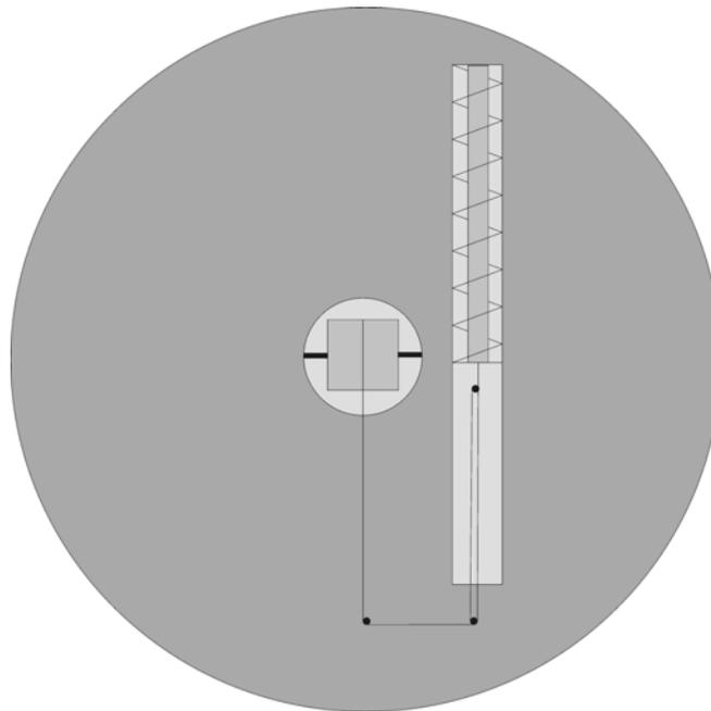
**Figure 5.2** A hollow buoy with horizontal spring and pulley-tack system. The darker tube inside of the spring is the dampener. (Top view).
