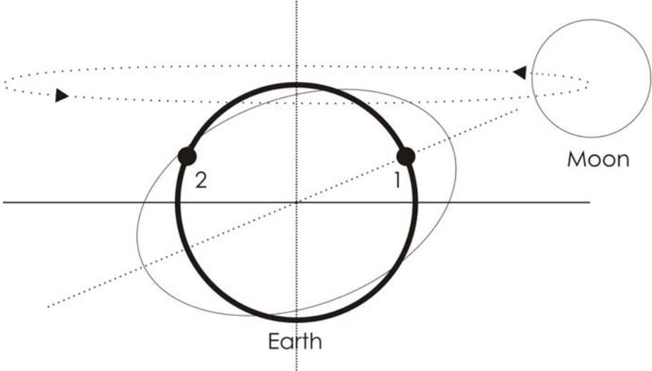
**Figure 2.2** Example of the basis of diurnal tides. Areas that are close to the points are subjected to one accentuated tidal maximum and minimum per day. (Figure is not at scale).
