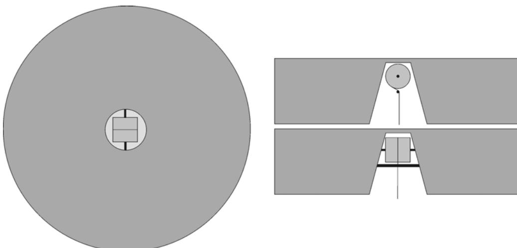
**Figure 5.7** A buoy with cone shaped hollow and guide wheel. The cone shape is to lessen the chances of damage to the line. Clockwise from left: view of the buoy from above, view from the side and view from the front.
