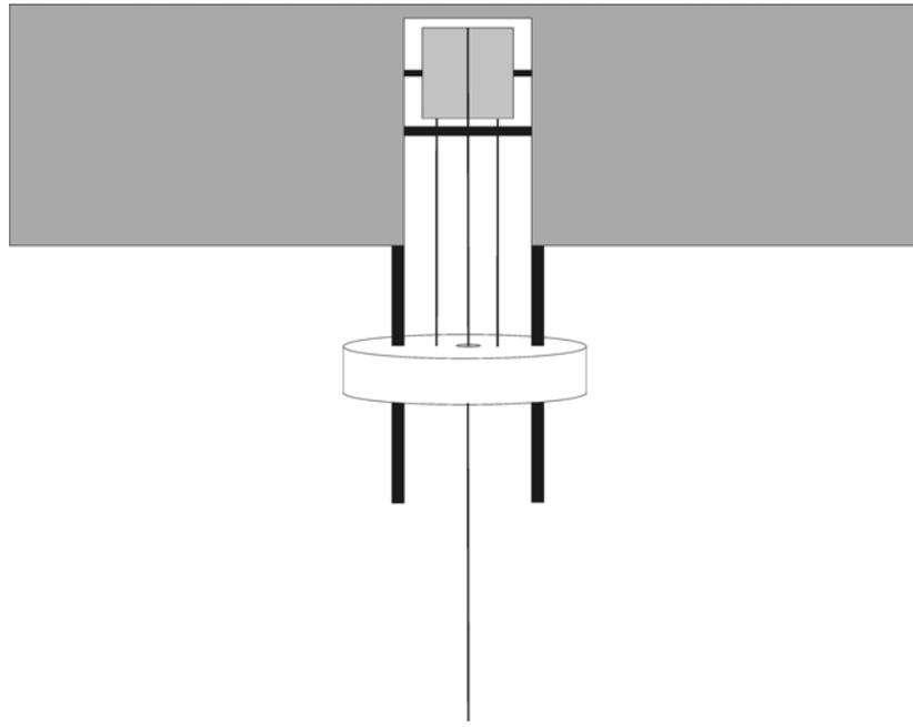
**Figure 5.4** *A hollow buoy with guide wheel and railed counterbalance. (Side view).*
