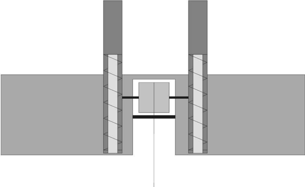
**Figure 5.1** A hollow buoy with guide wheel and dual vertical springs. The light grey inside the springs represent the dampeners. (Side view).
