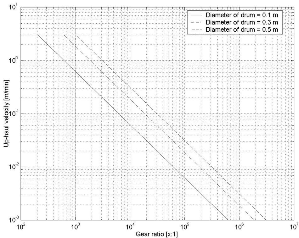
**Figure 7.5** The variation of the gear ratio on up-haul velocity at different drum diameters. This is with a motor working at 2000 rpm.
