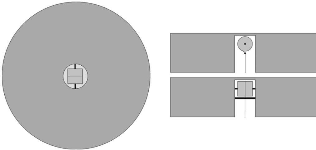
**Figure 5.6** A hollow buoy with guide wheel. Here the drum is centred in the buoy allowing for a smaller diameter of the inner hollow. A guide wheel is added to steer the line into a central position. Clockwise from left: view of the buoy from above, view from the side and view from the front.
