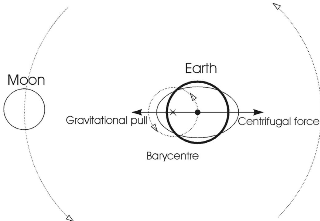
**Figure 2.1** *Illustration of the tidal generating forces on Earth. The gravitational pull of the two celestial bodies is balanced by the inertia or centrifugal force. The 'x' marks the location of the barycentre. Both the Earth and Moon rotate around this point. (Figure is not at scale).*
