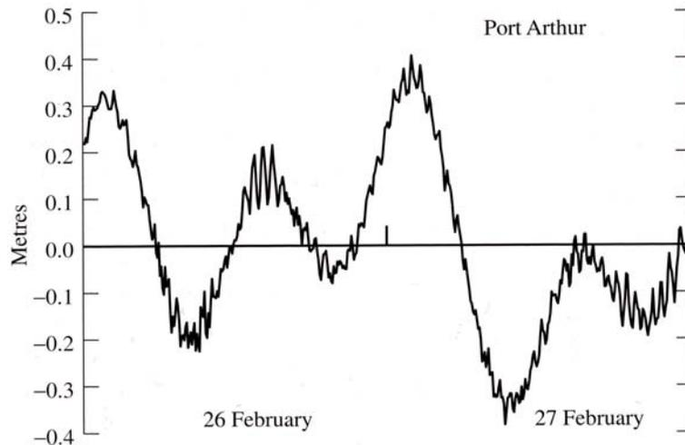
**Figure 2.6** *Seiches with a time interval of twenty minutes are superpositioned on top of the mixed tide at Port Arthur, Tasmania, Australia [11].*
