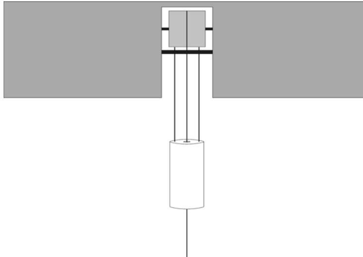
**Figure 5.3** *Hollow buoy with guide wheel and guided counterbalance. (Side view).*
