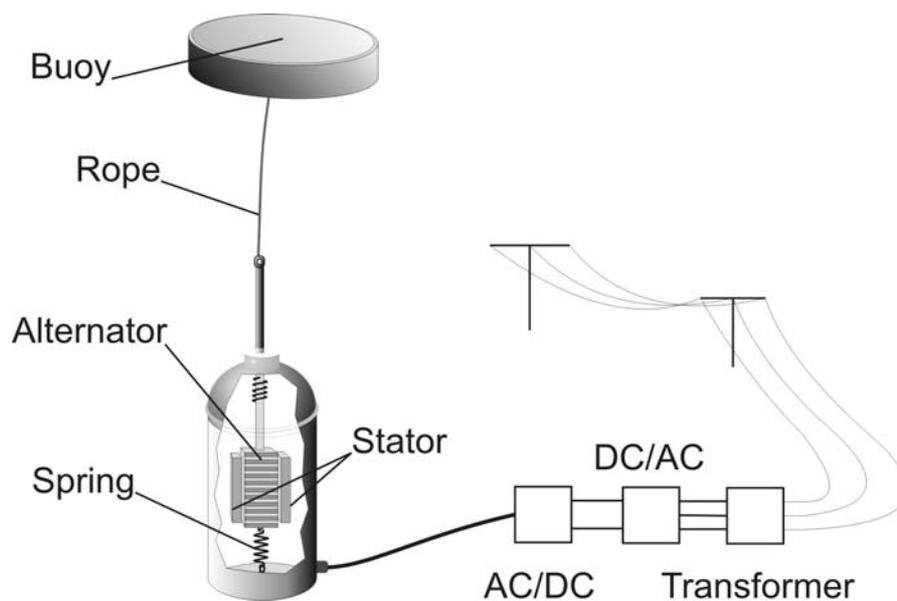
**Figure 1.1** A schematic illustration of the linear generator and its connection to the grid, from ref. [5].
