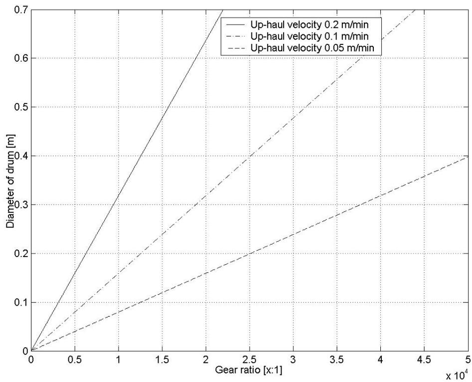
**Figure 7.4** *The influence of the drum diameter on the gear ratio of the electrical system.*
