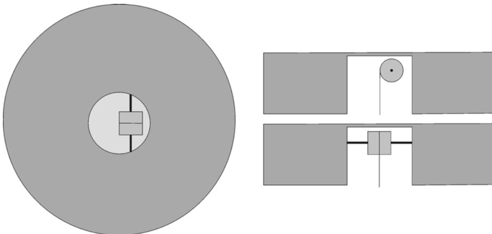
**Figure 5.5** A hollow buoy with large opening. The drum is placed asymmetrically inside the buoy to allow for the line to be centred. Clockwise from left: view of the buoy from above, view from the side and view from the front.
