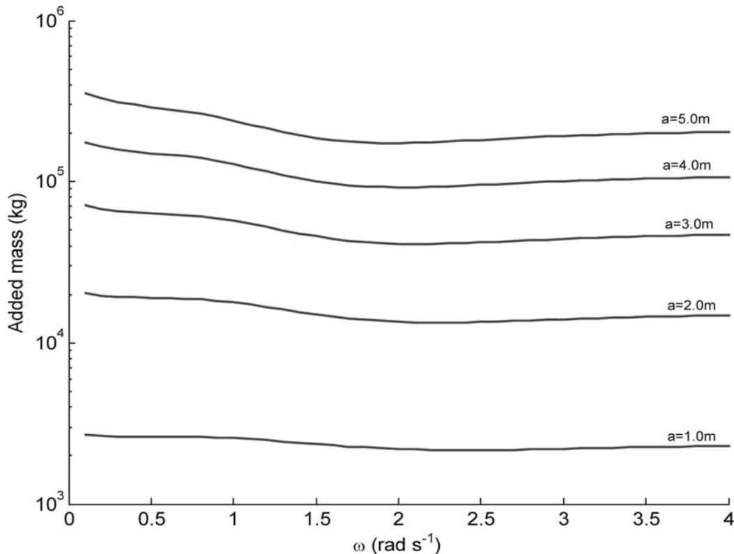
**Figure 6.1** Change in added mass with radius of buoy ( $a$ ) and angular wave frequency. Added mass increases with increasing radius. Draft (amount of buoy under the water line) is 1.5 m and the water depth is 23 m. Courtesy of supervisor Mikael Eriksson, previously unpublished)
