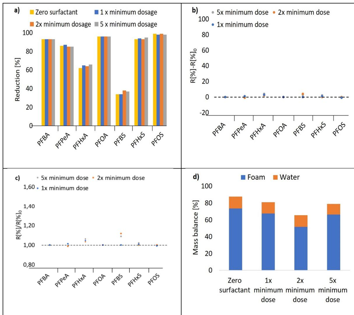
Figure 15 : a). Reduction of  $\sum_{11}$ PFASs with different doses of YES b). Difference in reduction between experimental runs containing surfactant and the reference of no surfactant. c). Change in reduction of PFASs expressed as a factor between the runs containing YES and the reference with zero addition d). Mass balance for each experiment
