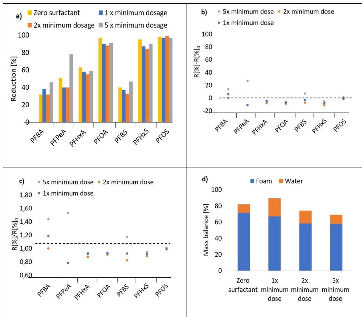
Figure 14 : a). Reduction of  $\sum_{11}$ PFASs with different doses of LAS b). Difference in reduction between experimental runs containing surfactant and the reference of no surfactant. c). Change in reduction of PFASs expressed as a factor between the runs containing LAS and the reference with zero addition d). Mass balance for each experiment.
