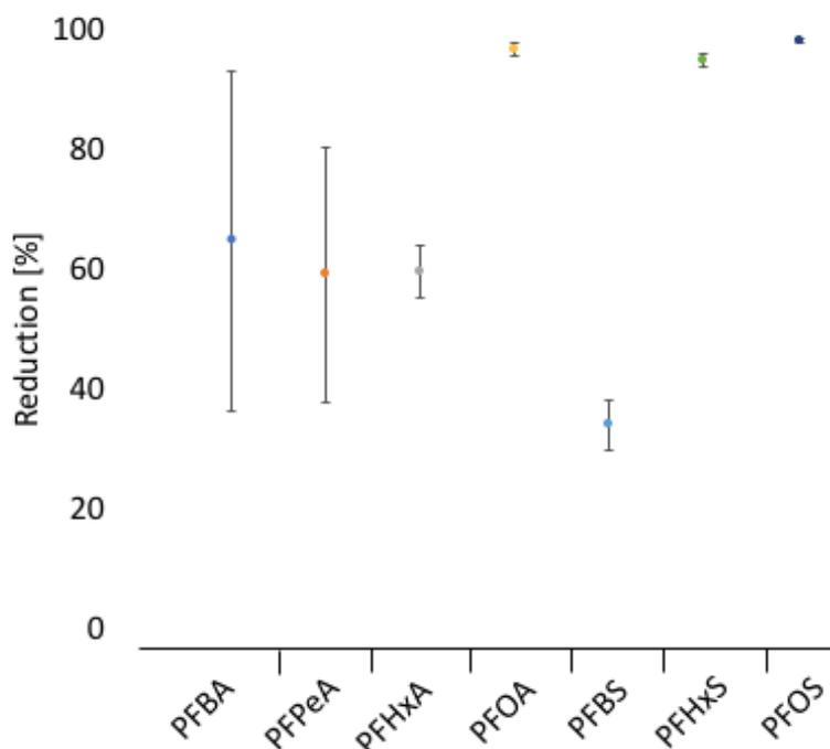
Figure 10: Average reduction and standard deviations for individual PFASs in the experimental runs with no addition of surfactants.
