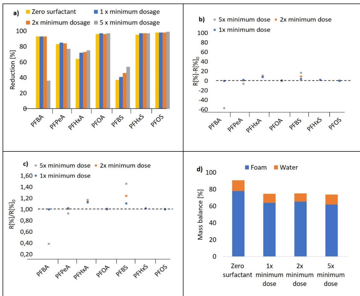
Figure 13 : a). Reduction of  $\sum_{11}$ PFASs with different doses of Simulsol S 10 b). Difference in reduction between experimental runs containing surfactant and the reference of no surfactant. c). Change in reduction of PFASs expressed as a factor between the runs containing Simulsol S 10 and the reference with zero addition d). Mass balance for each experiment.
