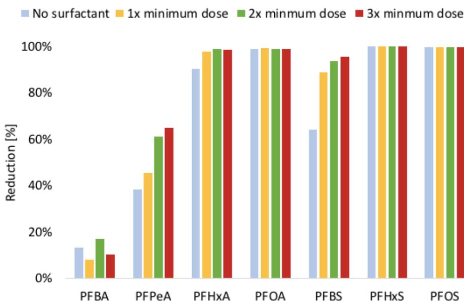
Figure 20: Average reduction for individual PFASs in the experimental runs with different doses of surfactant.
