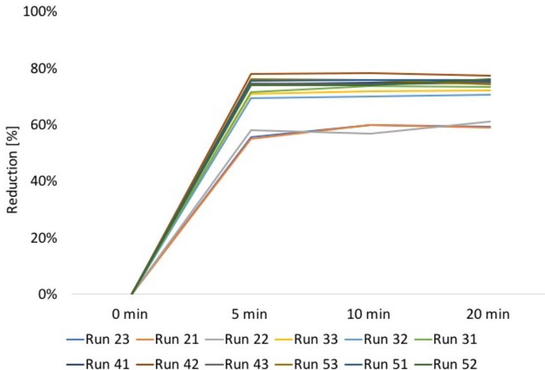
Figure 18: Average reduction of  $\sum$ short-chained PFASs at different time steps for each experimental run. Run 21-23 (Zero surfactant), run 31-33 (1x minimum dose), run 41-43 (2x minimum dose) and run 51-53 (3x minimum dose)
