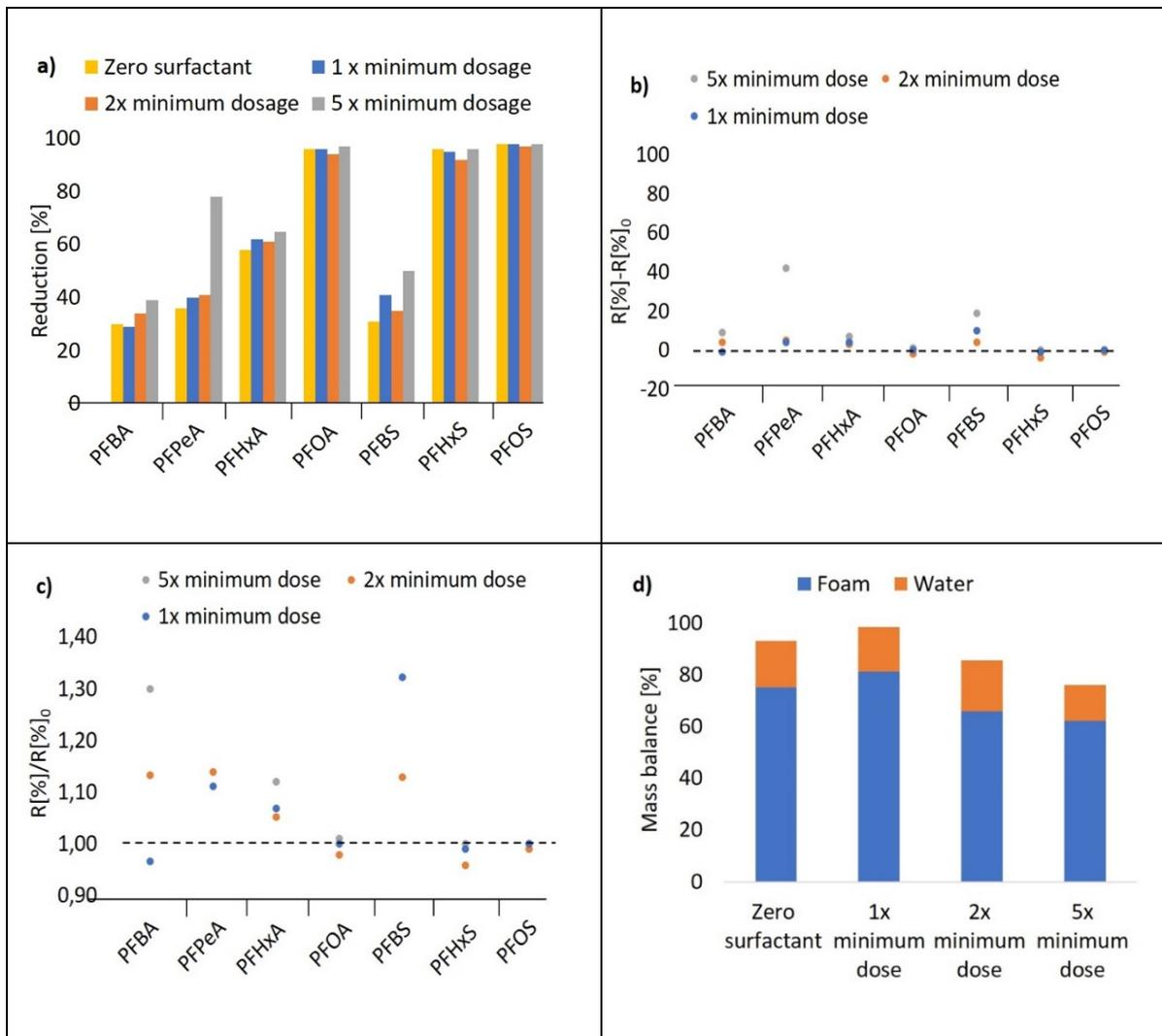
Figure 12 : a). Reduction of  $\sum_{11}$ PFASs with different doses of Marlinat 282/42 b). Difference in reduction between experimental runs containing surfactant and the reference of no surfactant. c). Change in reduction of PFASs expressed as a factor between the runs containing Marlinat 282/42 and the reference with zero addition d). Mass balance for each experiment.
