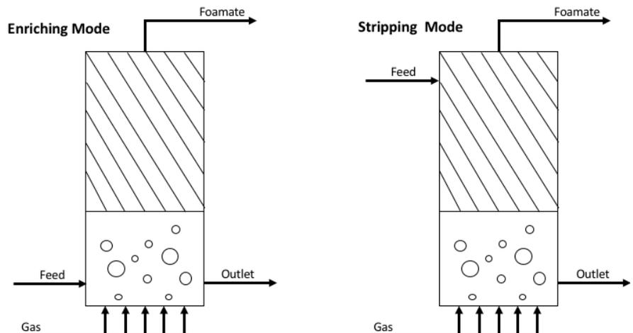
Figure 5: Two different continuous modes of foam fractionation operation, stripping mode and enriching mode. Adapted from Buckley et.al 2021.
