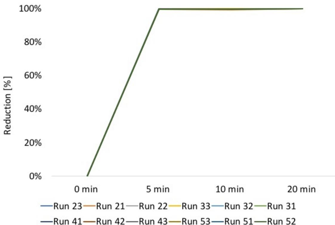
Figure 19: Average reduction of  $\Sigma$ long-chained PFASs at different time steps for each experimental run. Runs 21-23 (Zero surfactant), 31-33 (1x minimum dose), 41,43 (2x minimum dose) and 51-53 (3x minimum dose).
