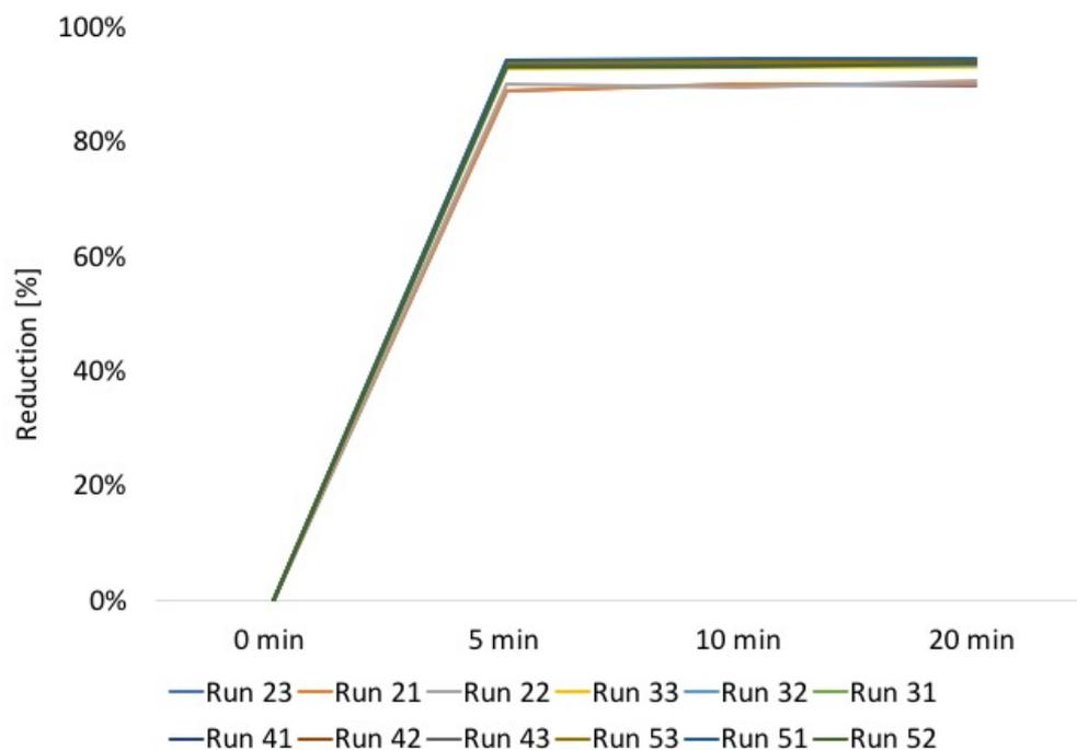
Figure 17: Reduction of  $\sum_{11}$ PFASs for all executed experimental runs at different time steps. Run 21-23 (Zero surfactant), run 31-33 (1x minimum dose), run 41-43 (2x minimum dose) and 51-53 (3x minimum dose).
