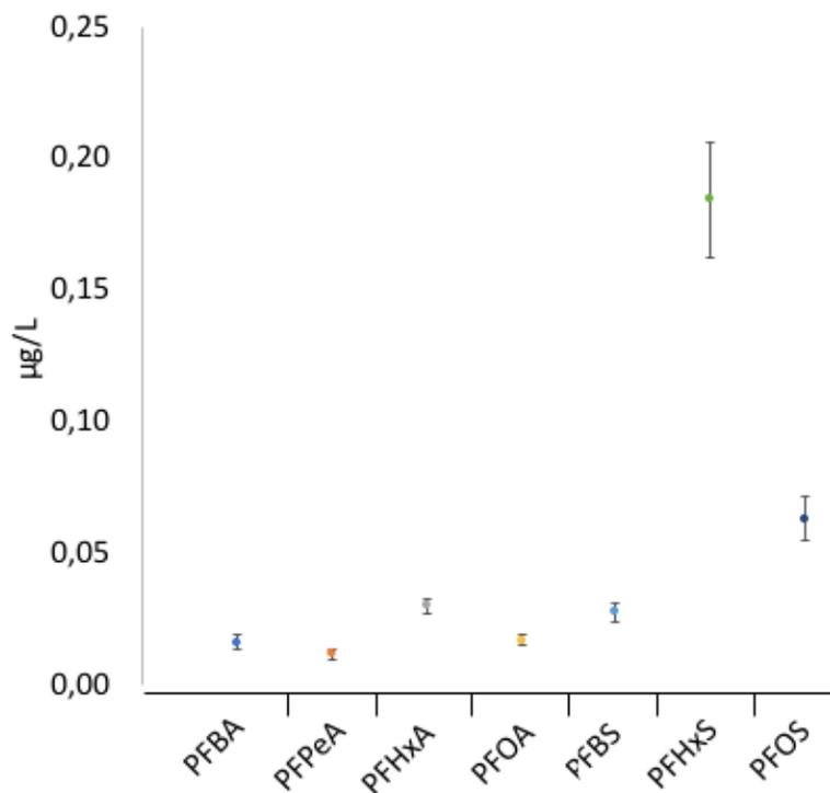
Figure 16: Average concentration for individual PFASs and their standard deviations detected in the NF concentrate.
