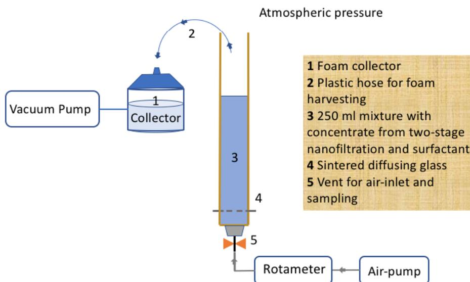
Figure 7: Foam fractionation setup for the laboratory experiments
