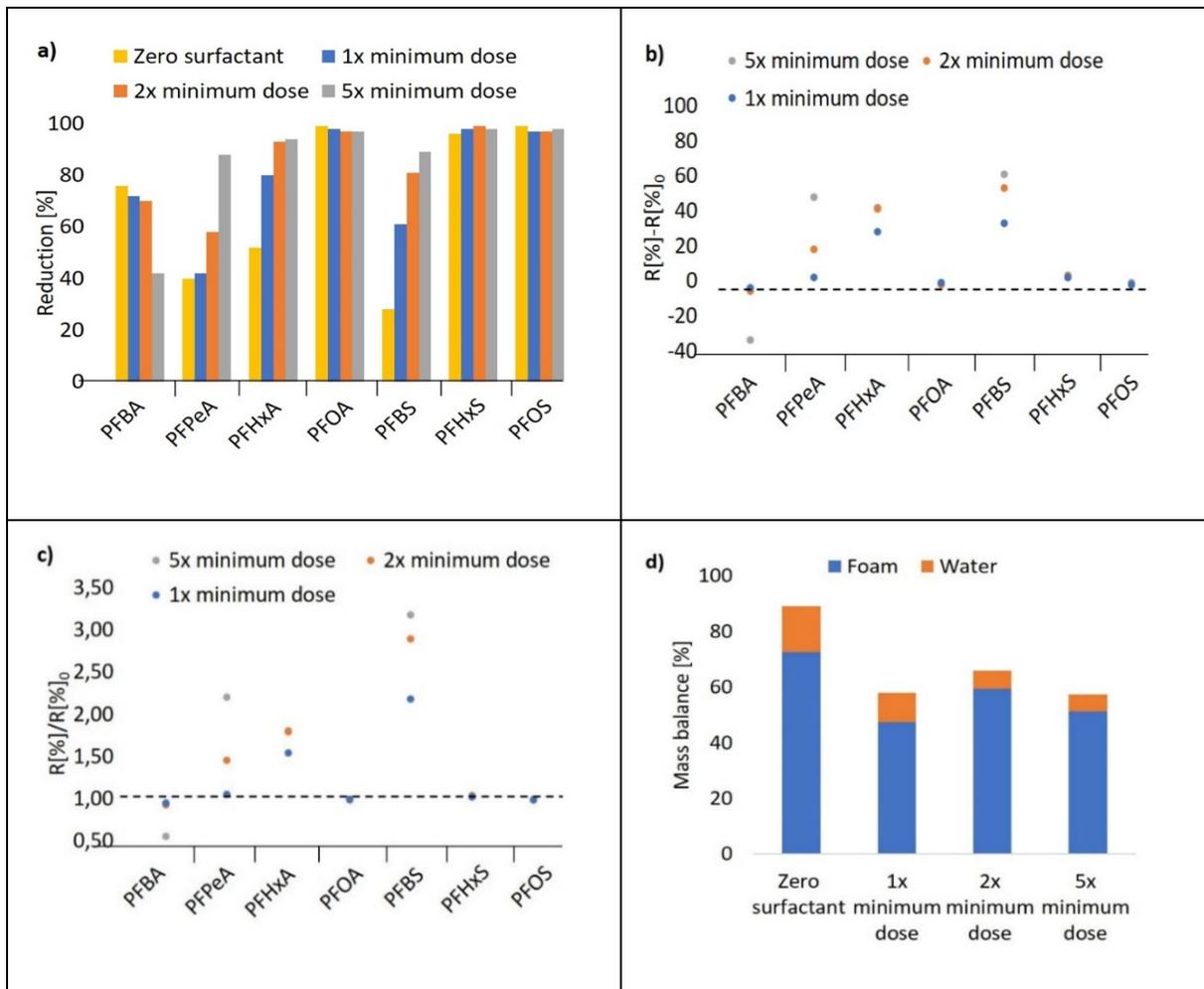
Figure 11: a). Reduction of  $\Sigma_{11}$ PFASs with different doses of Montaline C 40 b). Difference in reduction between experimental runs containing surfactant and the reference of no surfactant. c). Change in reduction of PFASs expressed as a factor between the runs containing Montaline C 40 and the reference with zero addition d). Mass balance for each experiment.
