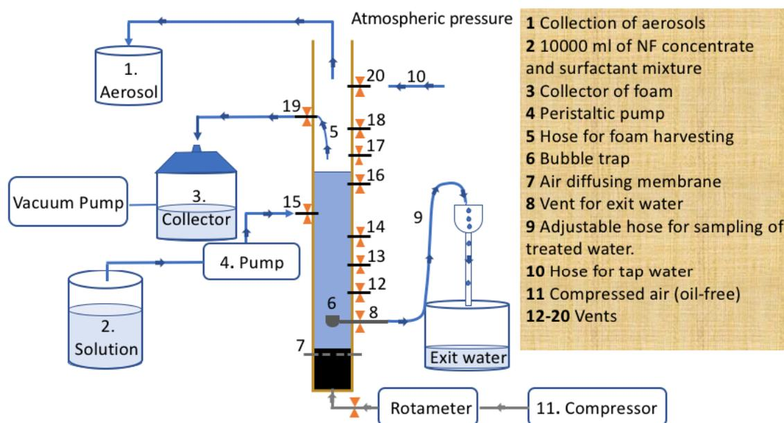
Figure 8: Experimental setup of the Pilot scale
