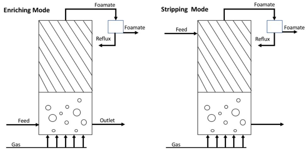
Figure 6: Two different continuous modes of foam fractionation with reflux. Enriching mode and stripping mode. Adapted from Buckley et.al 2021.
