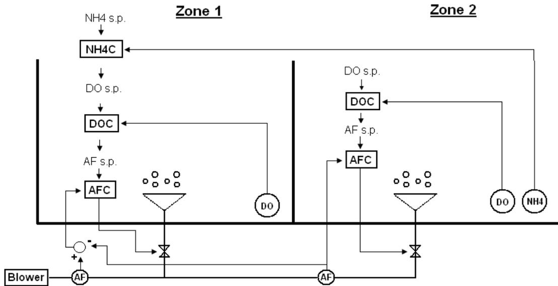
**Figure 16** Visualisation of the overall control in Sternö WWTP. NH4C is ammonium feedback control, DOC is DO control and AFC is airflow control. The circles with NH4, DO and AF represent measurement of ammonium, DO and airflow.
