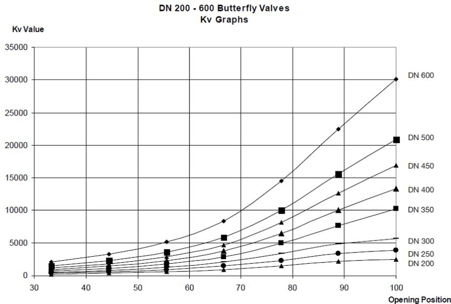
**Figure 6** Valve characteristics of butterfly valves. From AVK, 2011.
