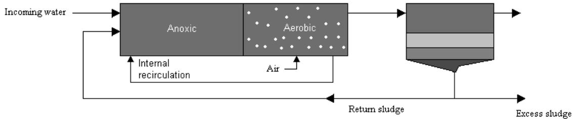
**Figure 3** Activated sludge process with pre-denitrification.
