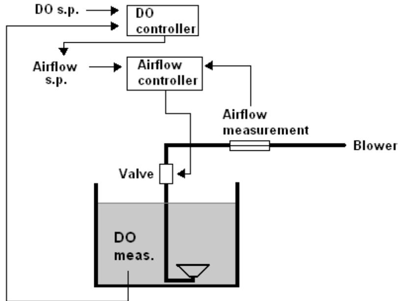
**Figure 10** DO cascade control. In the figure, s.p. is set-point.
