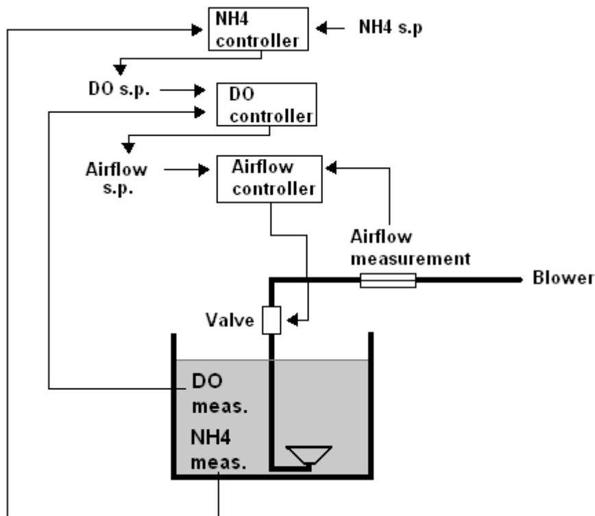
**Figure 11** Ammonium control. In the figure, s.p. is set-point.
