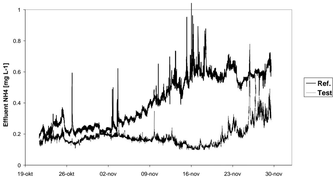
**Figure 24** Effluent ammonium concentration in each treatment line.
