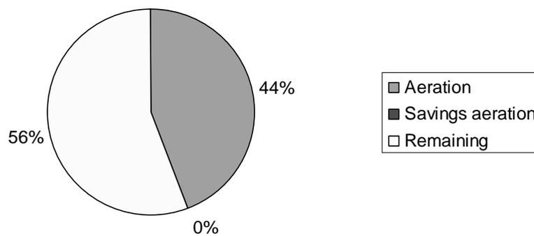
**Figure 26** Total energy consumption of Sternö WWTP in October 2011 without upgraded aeration system in the test line.
