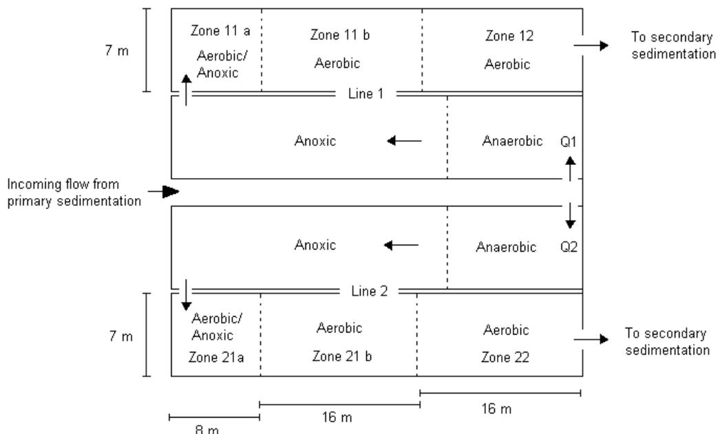
**Figure 15** Flowchart of the biological treatment in Sternö WWTP.
