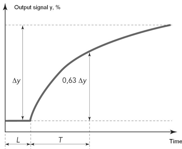
**Figure 13** An example of a step response test.
