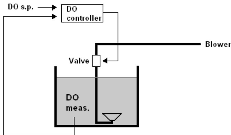
**Figure 9** Basic DO control. In the figure, s.p. is set-point.
