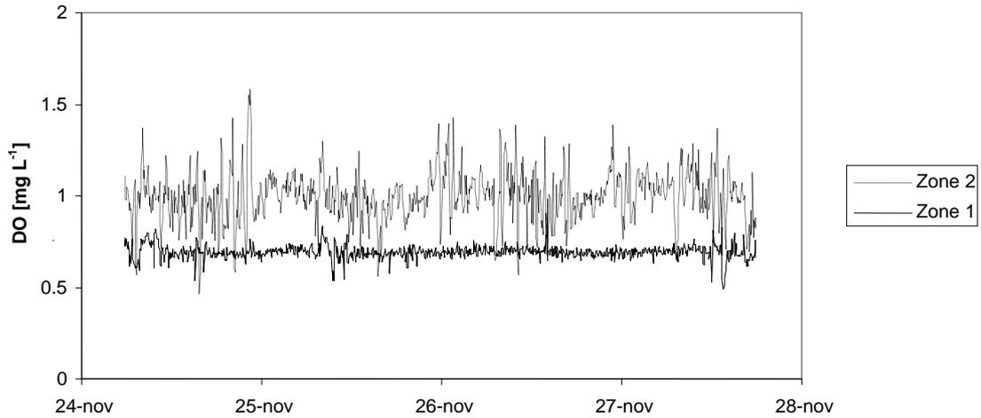
**Figure 20** DO concentrations in the test line for zone 1 and zone 2.
