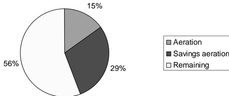
**Figure 28** Total energy consumption of Sternö WWTP in October 2011 if both the test line and the reference line would have had upgraded aeration system.
