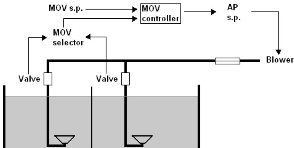
**Figure 12** Visualisation of MOV logic. s.p. is set-point and AP is air pressure.
