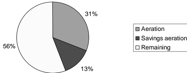
**Figure 27** Total energy consumption of Sternö WWTP in October 2011 with upgraded aeration system in the test line.
