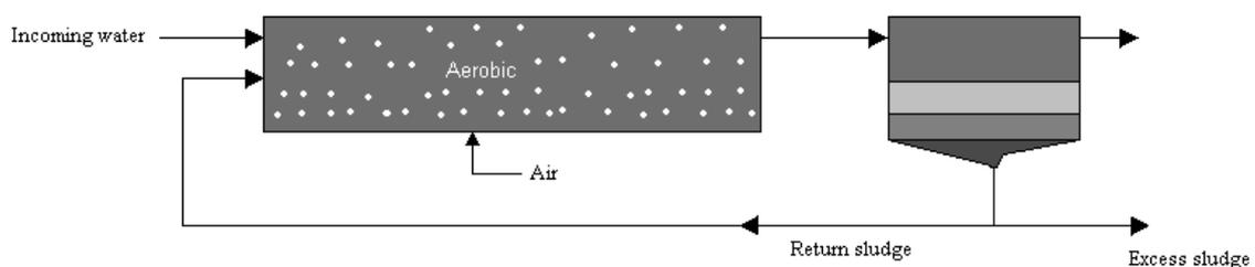
**Figure 2** A simple version of an activated sludge process.
