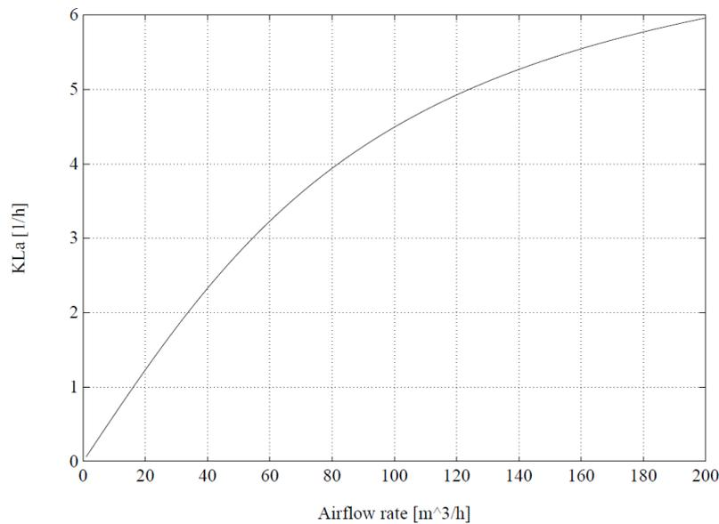
**Figure 4** Typical shape of the oxygen transfer function ( $K_L a(u)$ ) as a function of the airflow rate. From Lindberg, 1997.
