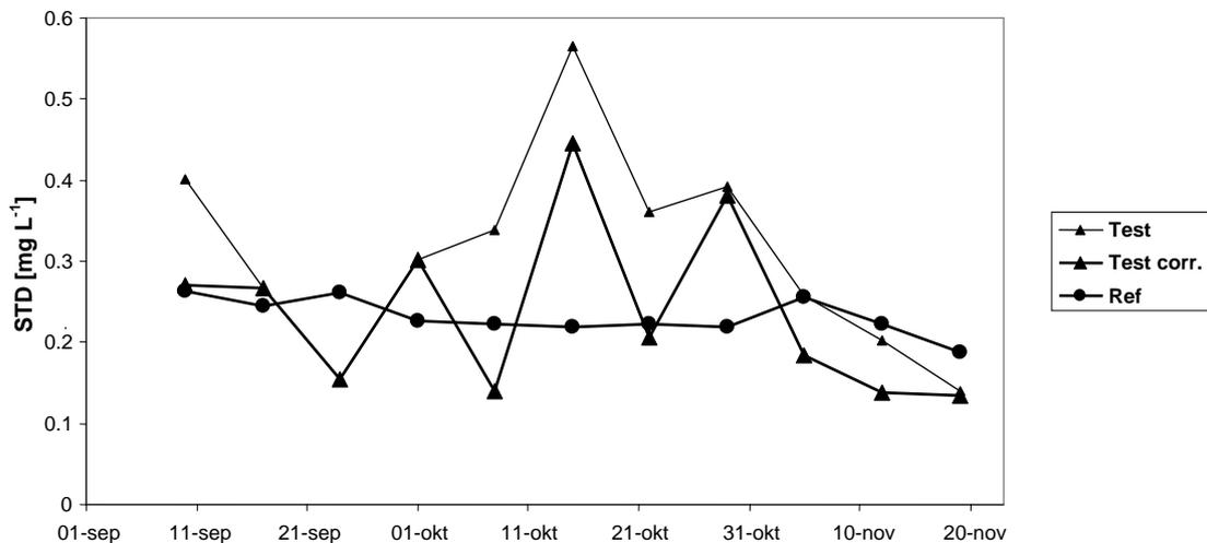
**Figure 23** DO standard deviation for zone 2 for the test line, the reference line and corrected values for the test line.
