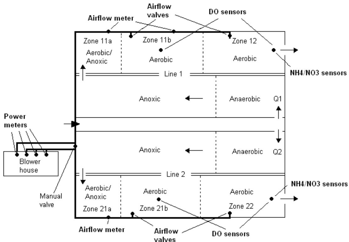
**Figure 17** Position of on-line measurements in the biological treatment of Sternö WWTP.
