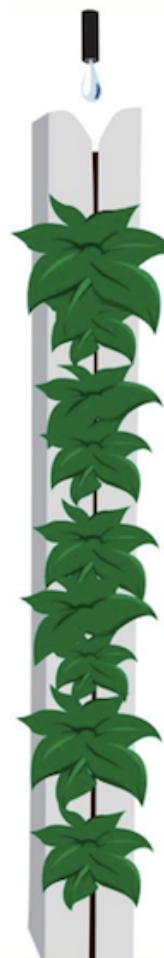
Figure 9 Schematic overview of the irrigation process. Water drips from a pipe at the top of the growing wall, down through the wicking strip and plugs with crops. Water is collected at the bottom (not showing). Retrieved from www.ZipGrow.com .
