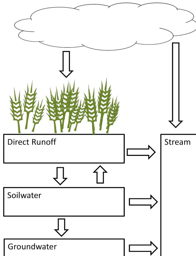
Figure 3. An example of interactions between three buckets (Direct Runoff, Soilwater and Groundwater) and the stream (Futter et al., 2013)
