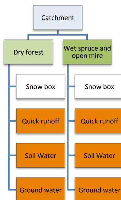
**Figure 4. The model structure used when modelling the hydrology in the catchments Aneboda, Gårdsjön, Kindla and Krycklan**
