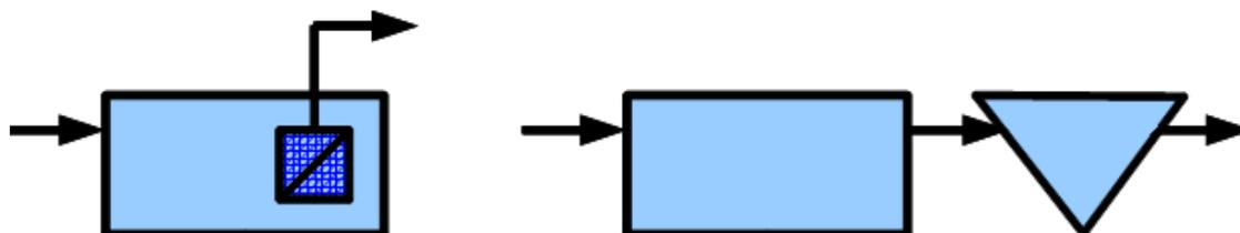
Figure 6. From the left: MBR system consisting of biotreatment (large rectangle) and membranes (small square), and CAS system consisting of biotreatment (large rectangle) and sedimentation (triangle). Arrows represent treated water flow.
