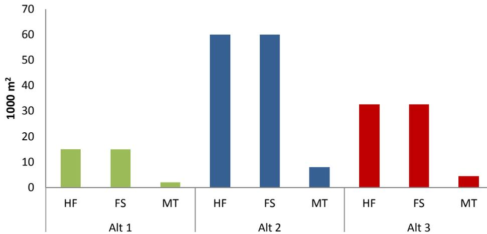
Figure 27. Required membrane area for alternative 1, 2 and 3, using HF, FS or MT membranes.
