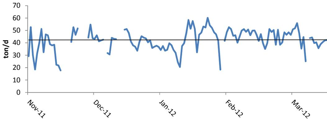
Figure 26. COD transport fluctuations at the inlet of the aerated lagoon at Korsnäs wastewater treatment.
