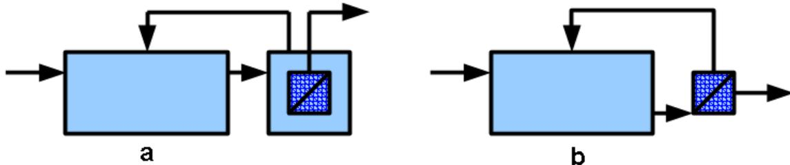
Figure 19. MBR configurations for application at Korsnäs: a) sMBR with separate compartment for membrane modules (HF and FS). b) rMBR (MT).
