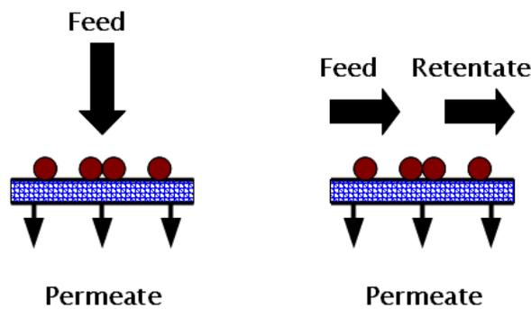
Figure 8. Feed, permeate and retentate directions for dead-end flow and crossflow.
