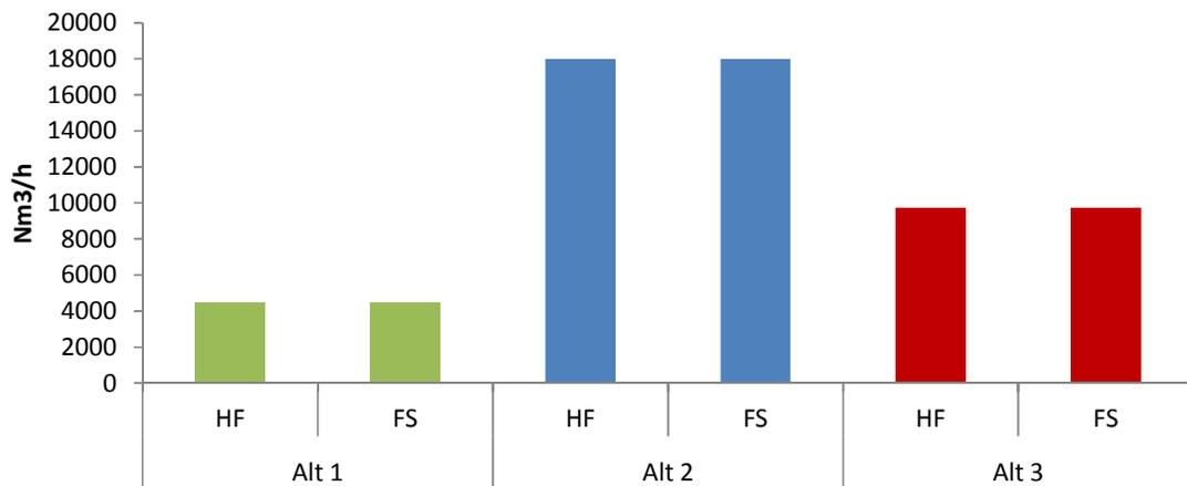
Figure 33. Aeration demand for membrane tanks for alternative 1, 2 & 3, using sMBR configuration.
