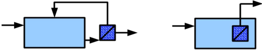
Figure 10. rMBR configuration with membrane unit placed externally, and sMBR configuration with membrane unit placed internally.
