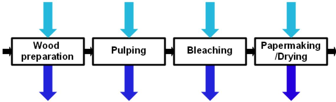
Figure 3. A schematic overview of the water flows in the process of making pulp and paper. Black arrows represent the direction of the process, while the light blue and dark blue arrows represent fresh water and waste water respectively.
