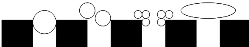
Figure 9. Pore clogging from the left: complete blocking, intermediate blocking standard blocking and cake layer.
