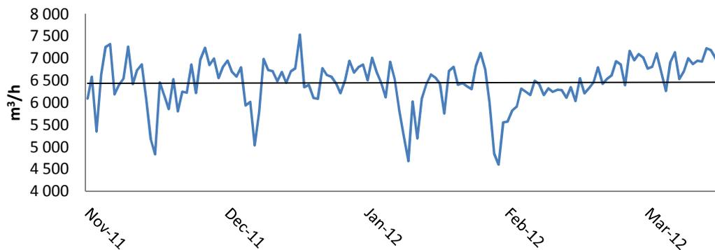
Figure 25. Flow fluctuations at the outlet of Korsnäs wastewater treatment.
