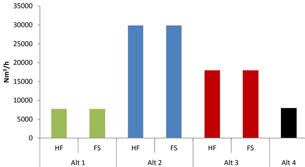
Figure 35. Total aeration demand for membrane and biotreatment tanks for alternative 1, 2, 3 & 4.
