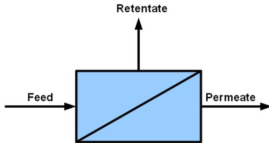
Figure 7. Feed entering a filtration unit, resulting in retentate and permeate.
