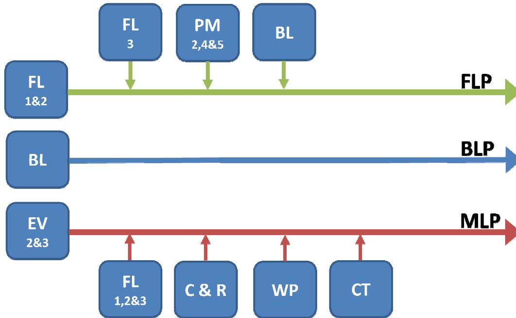
Figure 16. The three main pipes in the process wastewater transport at the Korsnäs pulp and paper mill; the fiber line pipe (FLP) containing wastewater from the fiber lines (FL), paper machines (PM) and bleaching effluent (BL); the bleaching pipe (BLP) containing wastewater from the bleach treatment (BL); miscellaneous pipe (MLP) containing wastewater from the evaporation (EV), the fiber lines (FL), causticizing and resin (C & R), wood preparation (WP) and the collection tank (CT).
