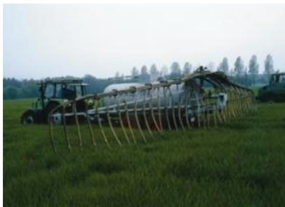
Figure 22. Tankwagon with trailing hoses (Source: Johansson et al.(not dated), with permission).
