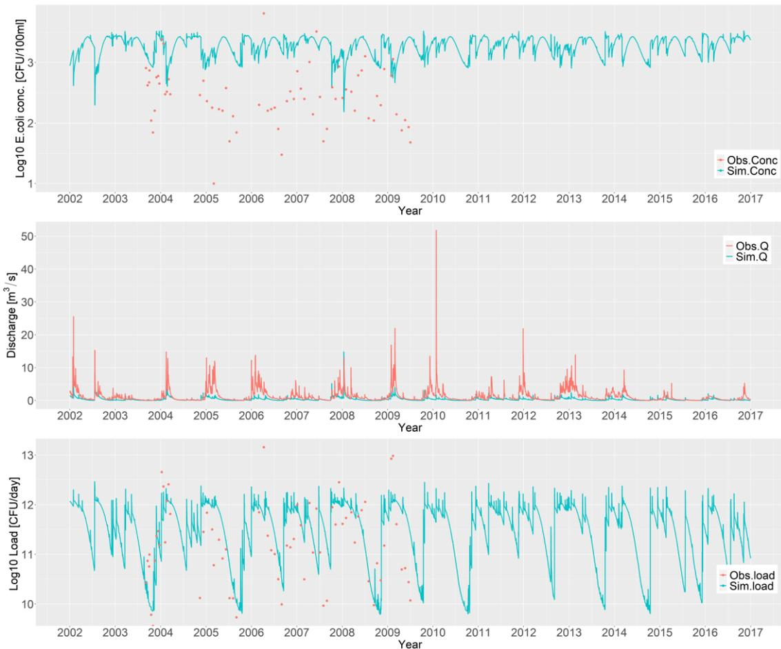
Figure 11. Time series of *E. coli* concentration, discharge, and *E. coli* load in a sub-catchment with no contribution from upstream areas with 100 % of the load from human rural sources.
