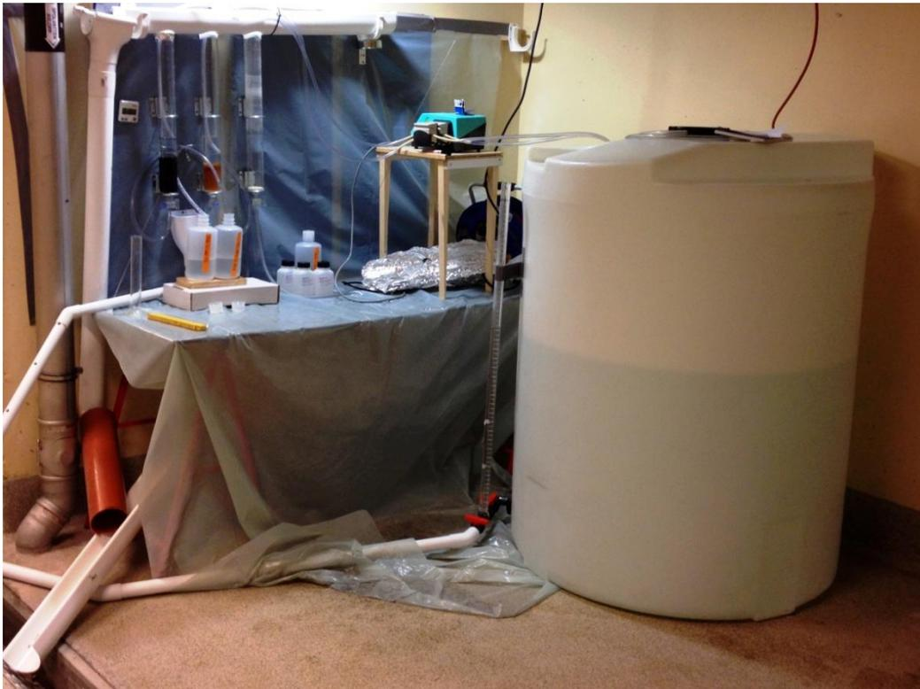
Figure F. The column experiments performed at Bäcklösa DWTP.
