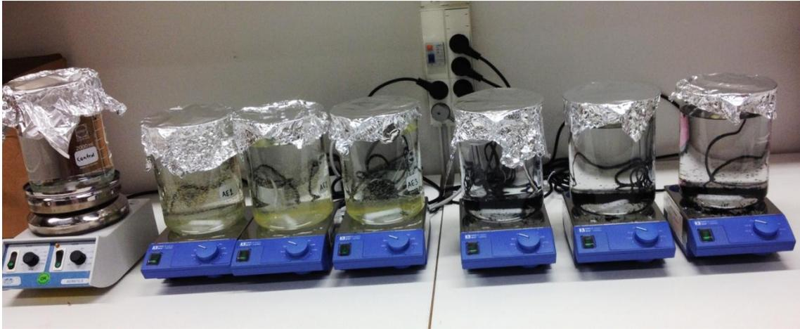
Figure E. The setup of the batch experiments. The first beaker contains the positive control without any treatment techniques. The three thereafter are treated with AE and the last three with GAC
