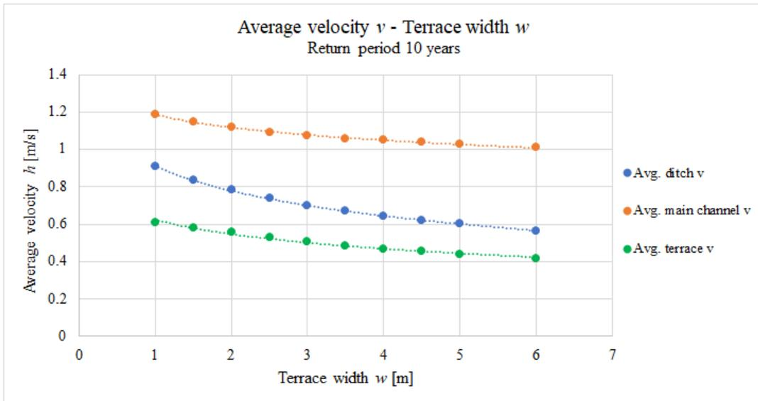
Figure D.2: Average velocity over terrace width in the theoretical two-stage ditch with return period of 10 years used.
