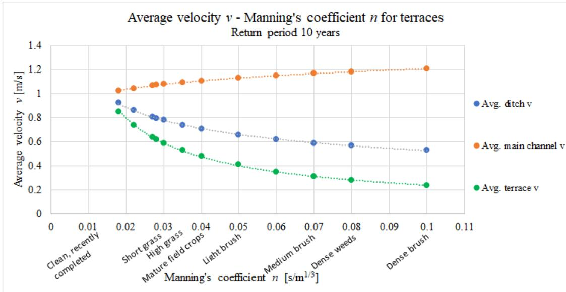
Figure F.2: Average velocity over Manning's coefficient varied on terraces with a 10 year return period. Used was the theoretical two-stage ditch.
