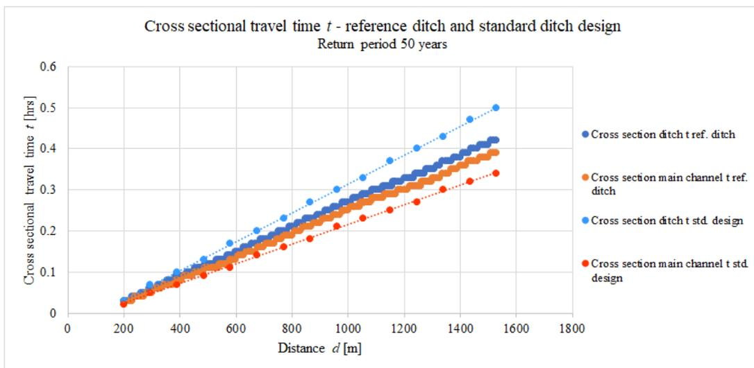
Figure H.3: Cross sectional travel time over distance of ditch with a return period of 50 years. Reference two-stage ditch and theoretical two-stage ditch of standard design are presented.
