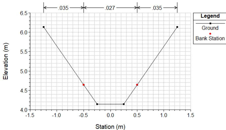
Figure 6: Schematic view of cross section design for a theoretical trapezoidal ditch modeled in HEC-RAS during climate change scenario study. Cross section showed as elevation above sea level over width by station. Manning’s coefficient are defined as  $n_1 = 0.035 \text{ s m}^{-1/3}$  for bank slopes and  $n_2 = 0.027 \text{ s m}^{-1/3}$  for the main channel.
