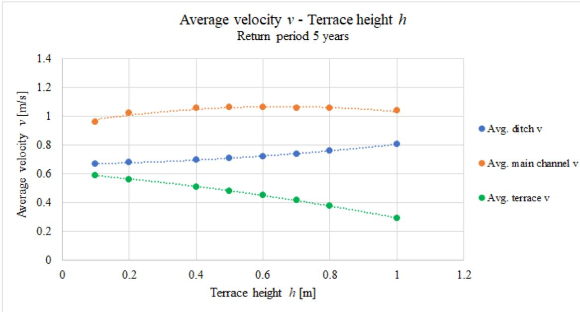
Figure 8: Average velocity  $v$  over terrace height  $h$  for return period 5 years in the theoretical two-stage ditch. Blue line represents average ditch velocity  $v$ , orange line is average velocity  $v$  in main channel, green line is average velocity  $v$  on terraces. Manning's coefficients were defined to  $n_1 = 0.035 \text{ s m}^{-1/3}$  on terraces and  $n_2 = 0.027 \text{ s m}^{-1/3}$  in the main channel.
