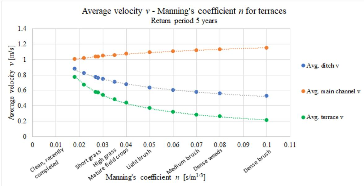
Figure 14: Average velocity  $v$  over Manning's coefficient  $n$  varied on terraces, in the theoretical two-stage ditch during a 5 year return period. Manning's coefficient in the main channel was  $n_2 = 0.027 \text{ s m}^{-1/3}$ . Explanations are included on axis for values of Manning's coefficient  $n$ . Blue line represents average ditch velocity  $v$ , orange line represents average main channel velocity  $v$ , green line represents average terrace velocity  $v$ .
