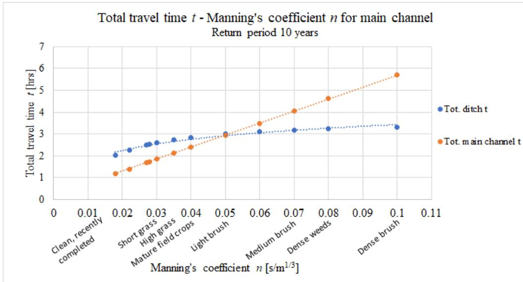
Figure G.1: Total travel time over Manning's coefficient varied in the main channel for a 10 year return period. Simulated was the theoretical two-stage ditch.
