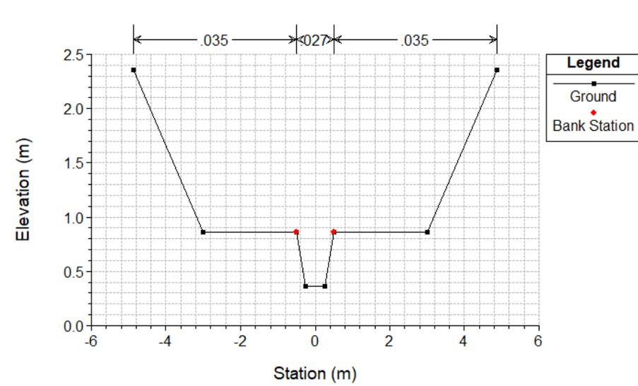
Figure 5: Schematic view of cross section design for a theoretical two-stage ditch modeled in HEC-RAS during climate change scenario study. Cross section showed as elevation above sea level over width by station. Manning’s coefficient are defined as  $n_1 = 0.035 \text{ s m}^{-1/3}$  for terraces and  $n_2 = 0.027 \text{ s m}^{-1/3}$  for the main channel.
