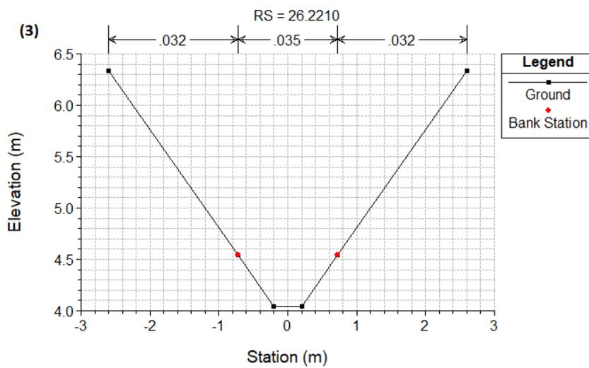
Figure 23: Cross section (3) showing a trapezoidal ditch shape at river station 26.2210 in the reference two-stage ditch. Defines the cross section shape occurring at (3) in Figure 20. Elevation above sea level over width by station. Values defining vegetation are observed values  $n_3 = 0.032 \text{ s m}^{-1/3}$  on bank slopes, and  $n_4 = 0.035 \text{ s m}^{-1/3}$  in the main channel.
