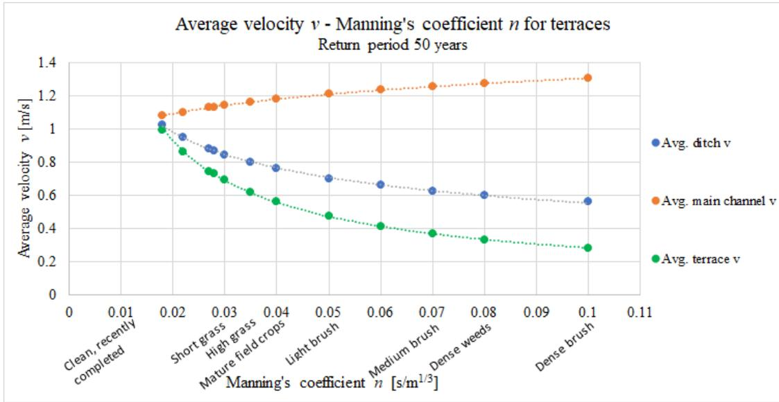
Figure F.4: Average velocity over Manning's coefficient varied on terraces in the theoretical two-stage ditch with a 50 year return period
