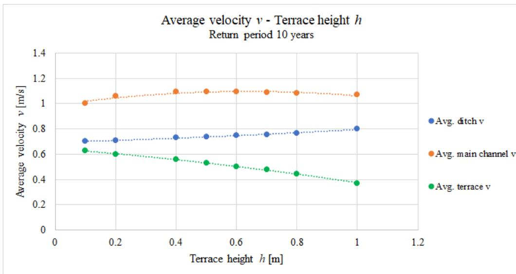
Figure C.2: Average velocity dependent on terrace height. Return period of 10 years in the theoretical two-stage ditch.
