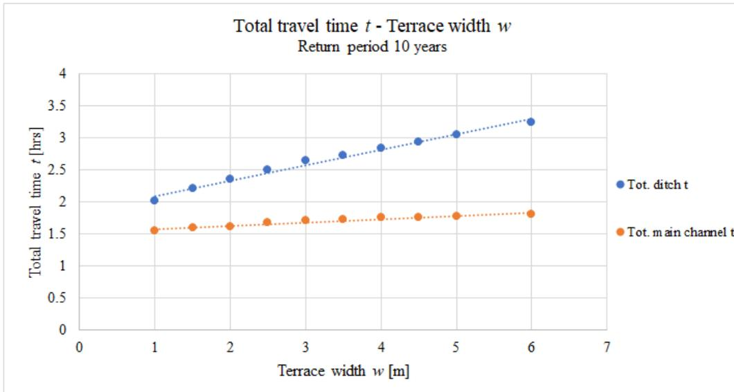
Figure D.1: Total travel time over terrace width, with return period of 10 years. Used was the theoretical two-stage ditch.
