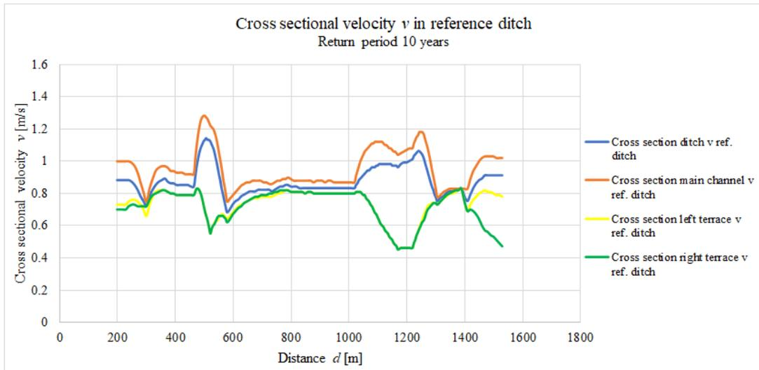
Figure H.2: Velocity for each cross section over the distance of the reference two-stage ditch. A 10 year return period were used.
