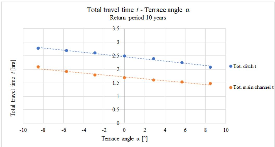
Figure E.1: Total travel time over terrace angle, for 10 year return period while simulating the theoretical two-stage ditch.
