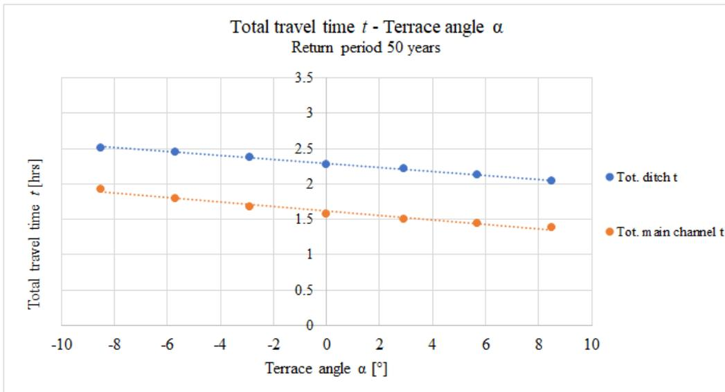
Figure E.3: Total travel time dependent on terrace angle in the theoretical two-stage ditch with a return period of 50 years.
