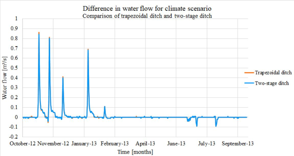
Figure 18: Difference in water flow, calculated between modified (future storm events) and original (current storm events) hydrological year of 2012-2013 over time for a theoretical two-stage ditch with standard design and a theoretical trapezoidal ditch. Light blue line is for the two-stage ditch, hidden behind the light blue line is the orange line for the trapezoidal ditch.
