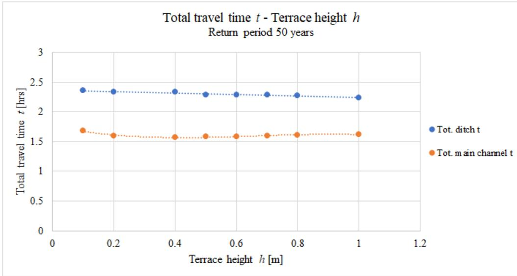
Figure C.3: Total travel time over terrace height with return period of 50 years, in the theoretical two-stage ditch.
