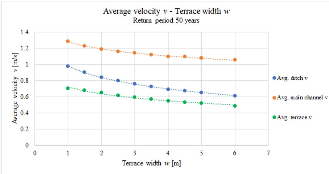
Figure D.4: Average velocity over terrace width, for a 50 year return period in the theoretical two-stage ditch.
