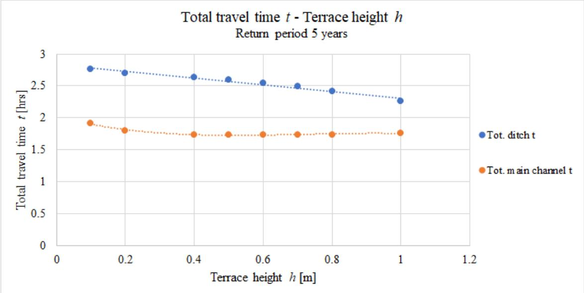
Figure 7: Total travel time  $t$  against terrace height  $h$  for a return period of 5 years in the theoretical two-stage ditch. Blue line is total ditch travel time  $t$ , orange line is total travel time  $t$  in the main channel. Manning’s coefficients used were  $n_1 = 0.035 \text{ s m}^{-1/3}$  on terraces and  $n_2 = 0.027 \text{ s m}^{-1/3}$  in the main channel.
