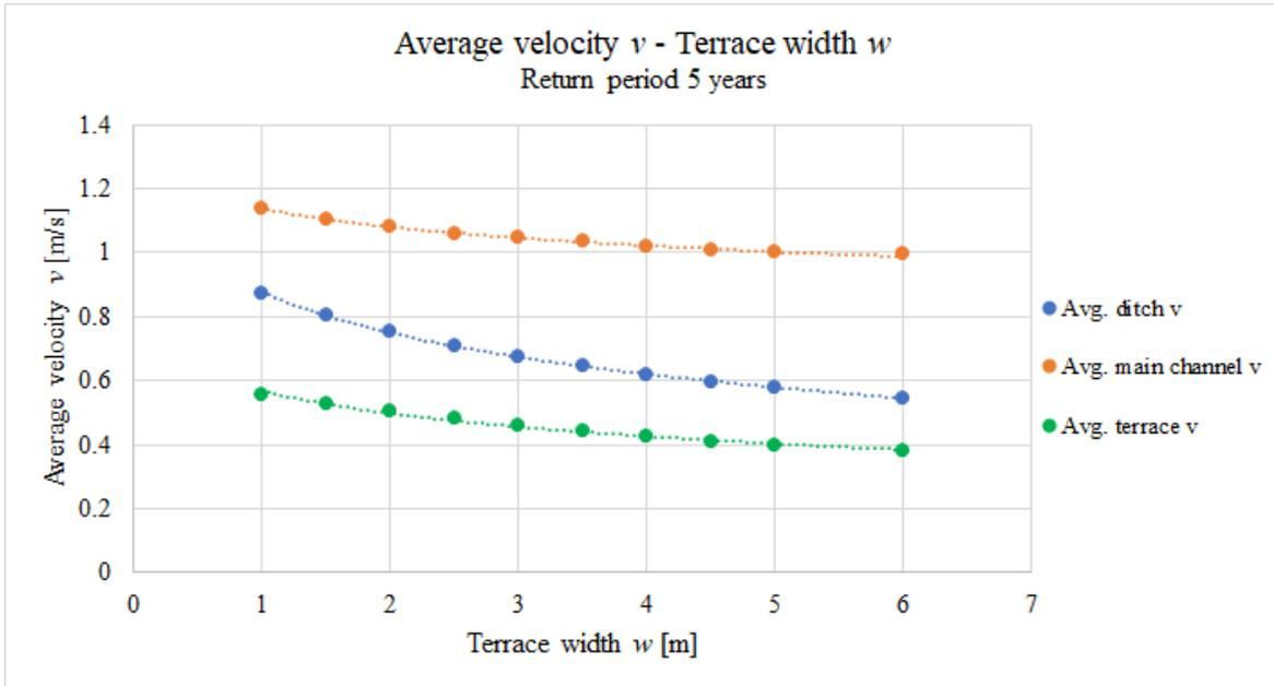
Figure 10: Average velocity  $v$  over terrace width  $w$  for return period of 5 years. Simulations were made in the theoretical two-stage ditch. Blue line represents average ditch velocity  $v$ , orange line is average velocity  $v$  in main channel, and green line is average velocity  $v$  on terraces. Manning's coefficients used in the design were  $n_1 = 0.035 \text{ s m}^{-1/3}$  on terraces and  $n_2 = 0.027 \text{ s m}^{-1/3}$  in main channel.
