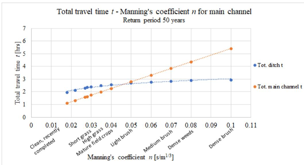
Figure G.3: Total travel time dependent on Manning's coefficient varied in the main channel for a 50 year return period, in the theoretical two-stage ditch.
