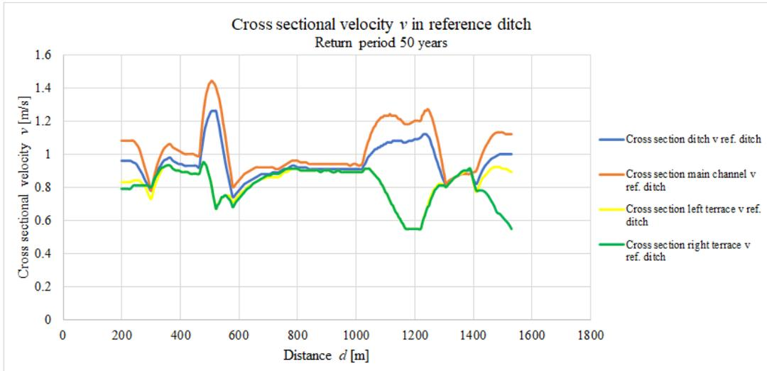
Figure H.4: Velocity for each cross section over the distance of the reference two-stage ditch. Return period 50 years were used.
