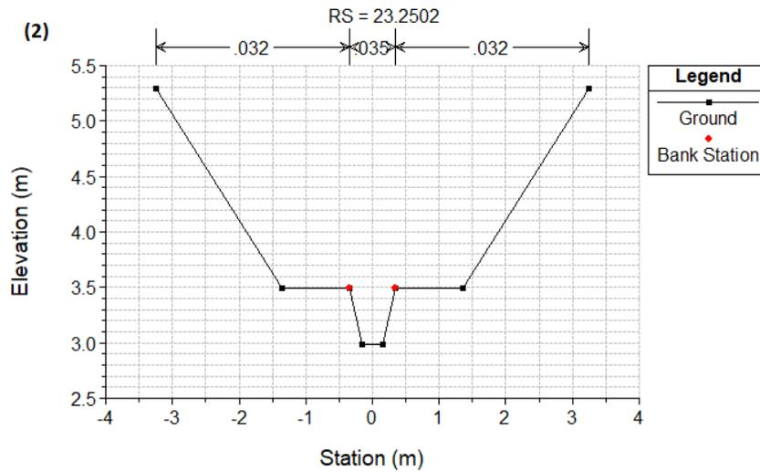
Figure 22: Cross section (2) showing a two-stage ditch shape at river station 23.2502 in the reference two-stage ditch. Defines the cross section shape occurring at (2) in Figure 20. Elevation above sea level over width by station. Values defining vegetation are observed values  $n_3 = 0.032 \text{ s m}^{-1/3}$  on terraces, and  $n_4 = 0.035 \text{ s m}^{-1/3}$  in the main channel.
