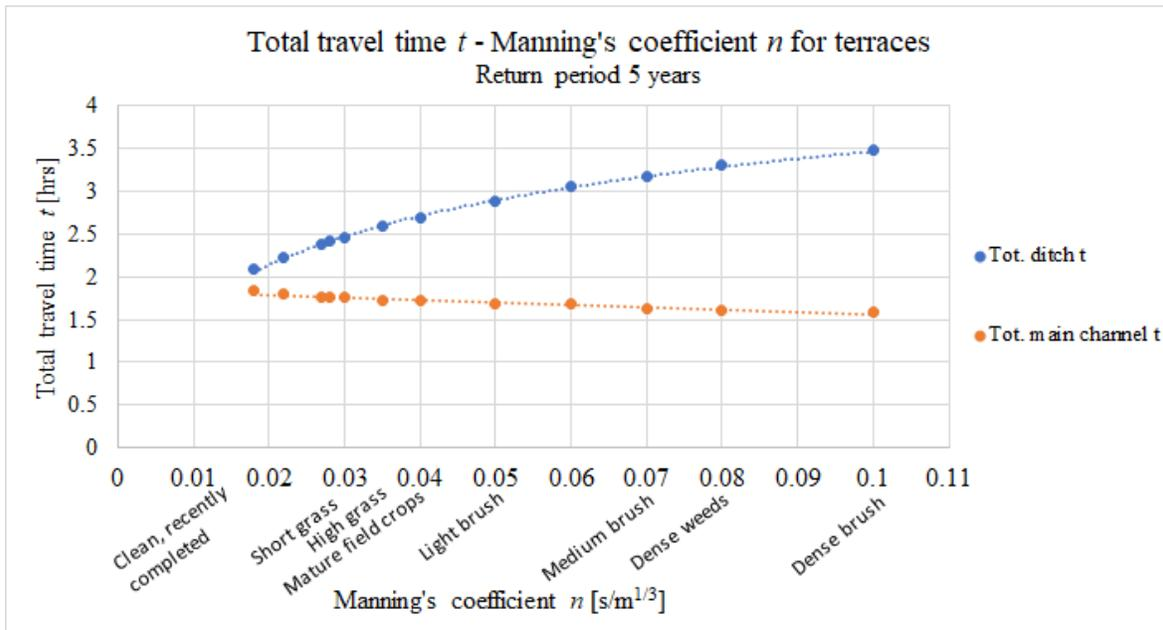
Figure 13: Total travel time  $t$  over Manning’s coefficient  $n$  varied on terraces. For return period of 5 years in the theoretical two-stage ditch. Manning’s coefficient in the main channel was  $n_2 = 0.027 \text{ s m}^{-1/3}$ . Explanations for values of Manning’s coefficient  $n$  are included on axis. Blue line represents total ditch travel time  $t$ , orange line is total main channel travel time  $t$ .
