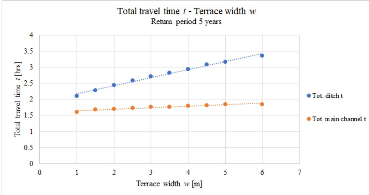
Figure 9: Total travel time  $t$  over terrace width  $w$  for return period of 5 years, for the theoretical two-stage ditch. Blue line is total ditch travel time  $t$ , orange line is total main channel travel time  $t$ . Manning's coefficients defined were  $n_1 = 0.035 \text{ s m}^{-1/3}$  on terraces and  $n_2 = 0.027 \text{ s m}^{-1/3}$  in the main channel.
