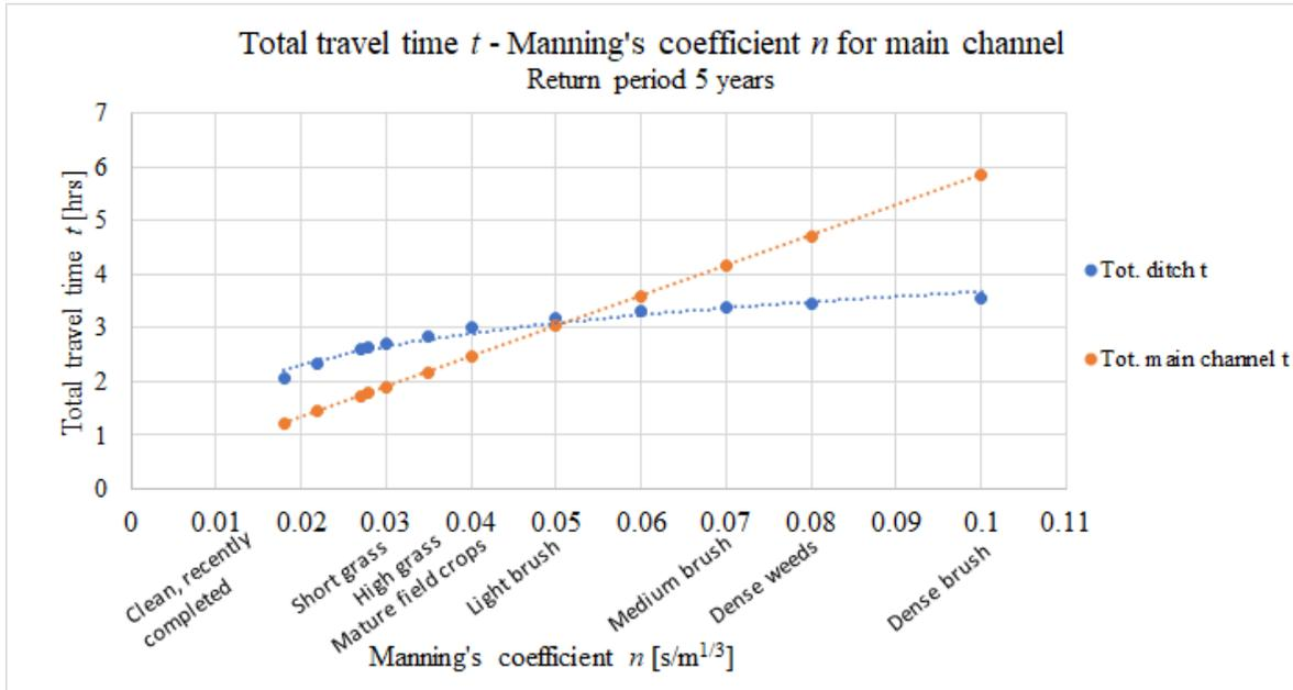
Figure 15: Total travel time  $t$  over Manning's coefficient  $n$  varied in the main channel in the theoretical two-stage ditch for 5 year return period. Manning's coefficient on terraces was kept at  $n_1 = 0.035 s m^{-1/3}$ . Explanations for Manning's coefficient  $n$  are included on axis. Blue line is total ditch travel time  $t$ , orange line is total main channel travel time  $t$ .
