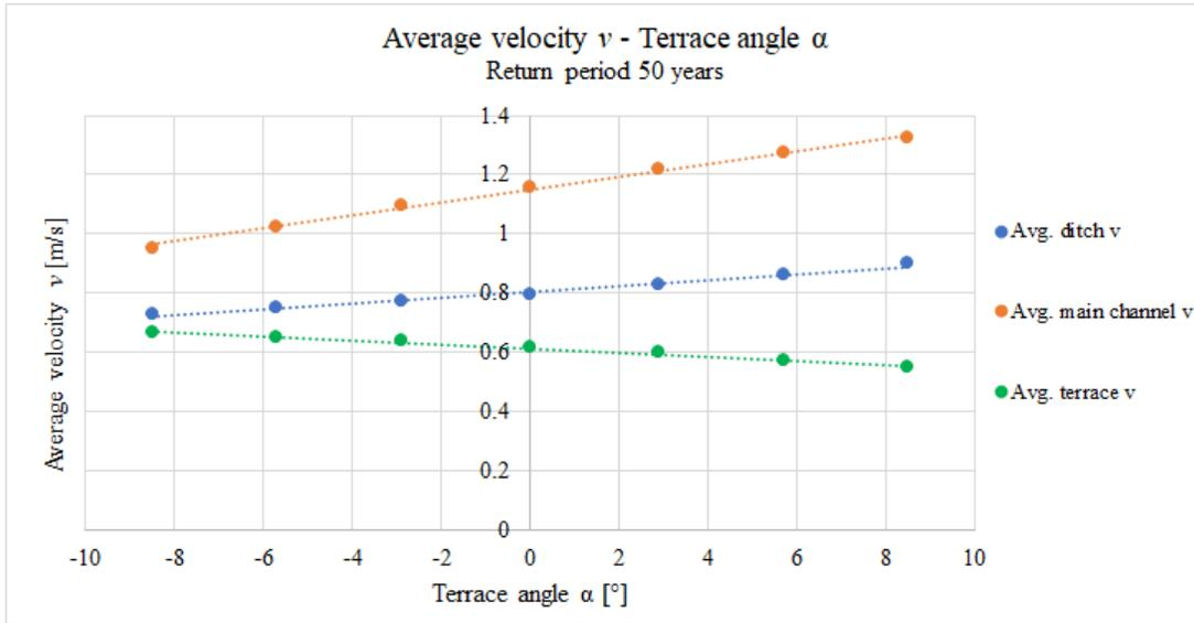
Figure E.4: Average velocity over terrace angle with a 50 year return period. Used ditch shape was the theoretical two-stage ditch.
