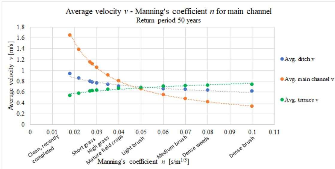
Figure G.4: Average velocity over Manning's coefficient in main channel in the theoretical two-stage ditch with a return period of 50 years.
