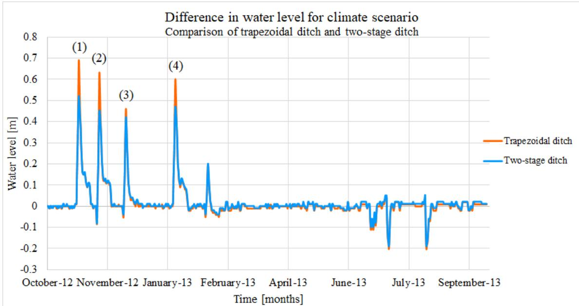
Figure 17: Difference in water level between modified (future storm events) and original (current storm events) hydrological year of 2012-2013 over time. Orange line is for the theoretical trapezoidal ditch shape, and light blue line is for the theoretical two-stage ditch shape of standard design. Marked by numbers (1)-(4) are peak water levels during winter months, with differences between ditch designs presented in Table 9.
