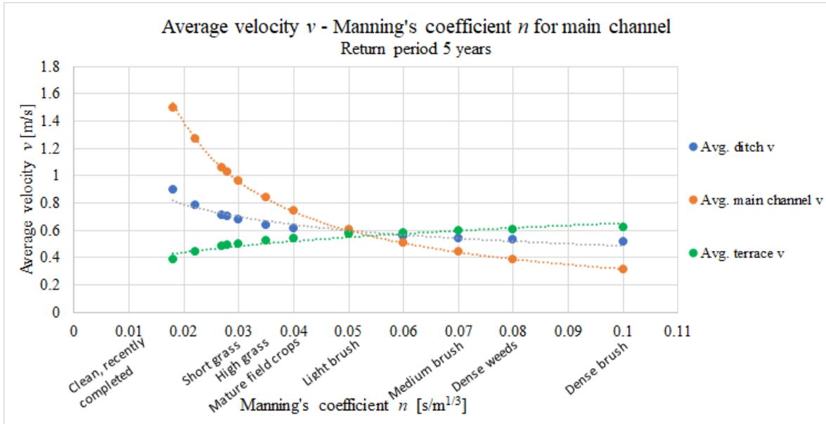
Figure 16: Average velocity  $v$  over Manning's coefficient  $n$  in the main channel, in the theoretical two-stage ditch. Used was a 5 year return period. Manning's coefficient on terraces were  $n_1 = 0.035 \text{ s m}^{-1/3}$ . Explanations are included on axis for values of Manning's coefficient  $n$ . Blue line represents average ditch velocity  $v$ , orange line represents average main channel velocity  $v$ , green line represents average terrace velocity  $v$ .
