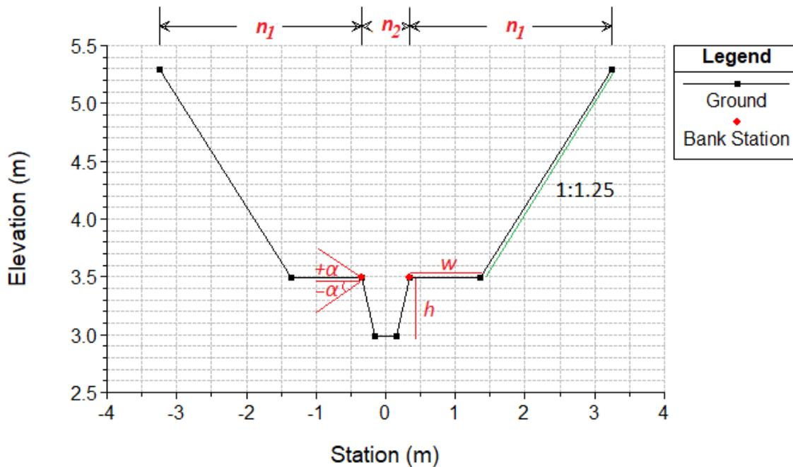
Figure 2: Schematic view of cross section design used in HEC-RAS for modeling a theoretical two-stage ditch, as elevation above sea level over width by station. Red colour represents variable parameters terrace height  $h$ , terrace width  $w$ , terrace angle  $\alpha$  for positive and negative values, and Manning's coefficient  $n_1$  for terraces and  $n_2$  for the main channel. The bank slope is 1:1.25, marked in green.
