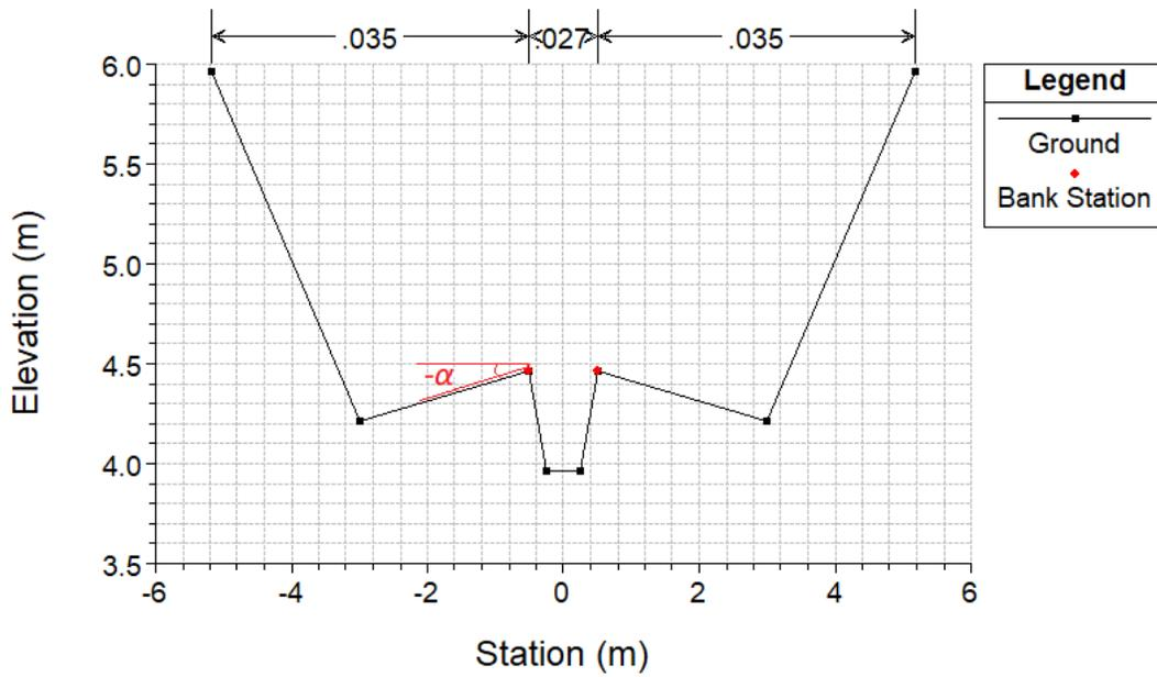
Figure 3: Example of cross section with terraces angled away from the main channel. Presented as elevation above sea level over width by station. Corresponds to a negative value of terrace angle  $\alpha$ . Manning's coefficient is defined as  $n_1 = 0.035 \text{ s m}^{-1/3}$  on terraces and  $n_2 = 0.027 \text{ s m}^{-1/3}$  in the main channel.
