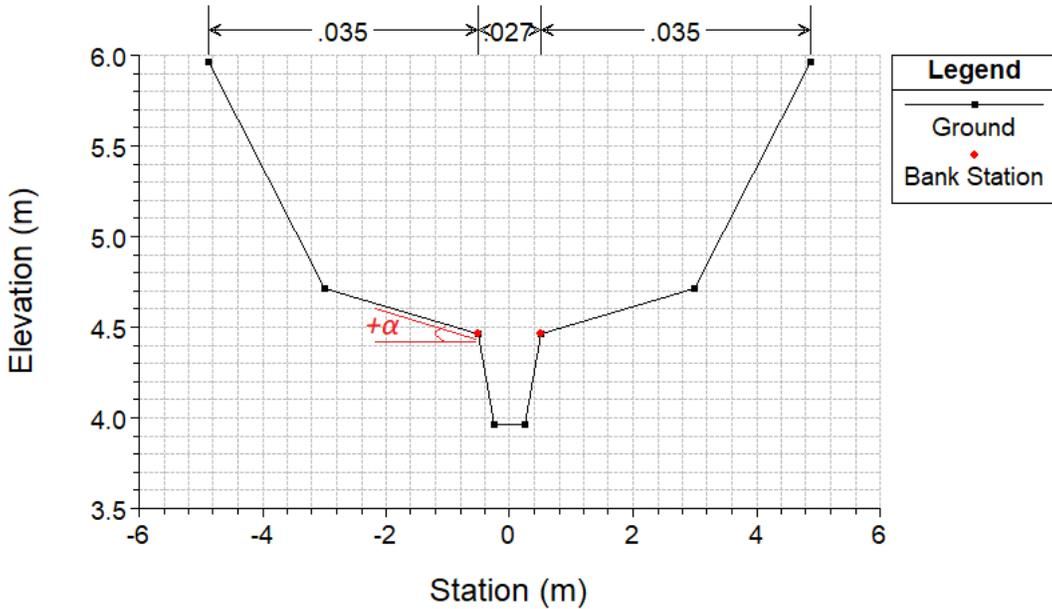
Figure 4: Example of cross section with terraces angled toward the main channel. Presented as elevation above sea level over width by station. Corresponds to a positive value of terrace angle  $\alpha$ . Manning's coefficient is defined as  $n_1 = 0.035 \text{ s m}^{-1/3}$  on terraces and  $n_2 = 0.027 \text{ s m}^{-1/3}$  in the main channel.
