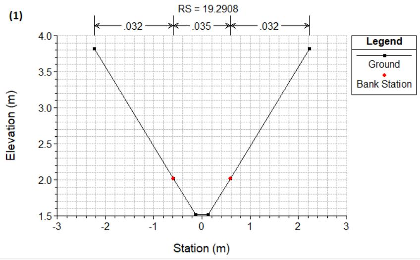
Figure 21: Cross section (1) showing a trapezoidal ditch shape at river station 19.2809 for the reference two-stage ditch. Defines the cross section shape occurring at (1) in Figure 20. Elevation above sea level over width by station. Values defining vegetation are observed values  $n_3 = 0.032 \text{ s m}^{-1/3}$  on bank slopes, and  $n_4 = 0.035 \text{ s m}^{-1/3}$  in the main channel.
