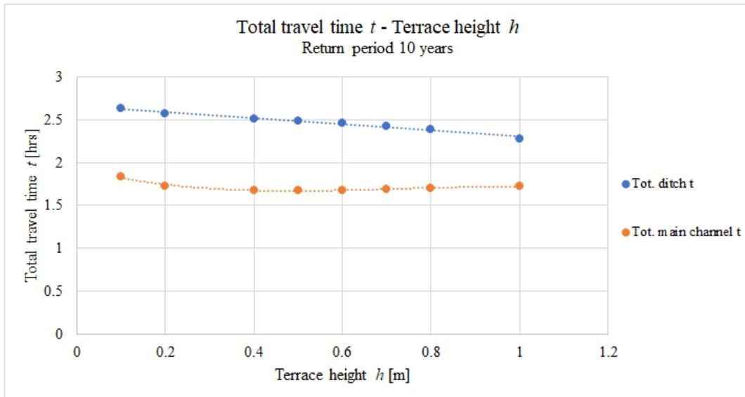
Figure C.1: Total travel time over terrace height, for return period of 10 years in the theoretical two-stage ditch.
