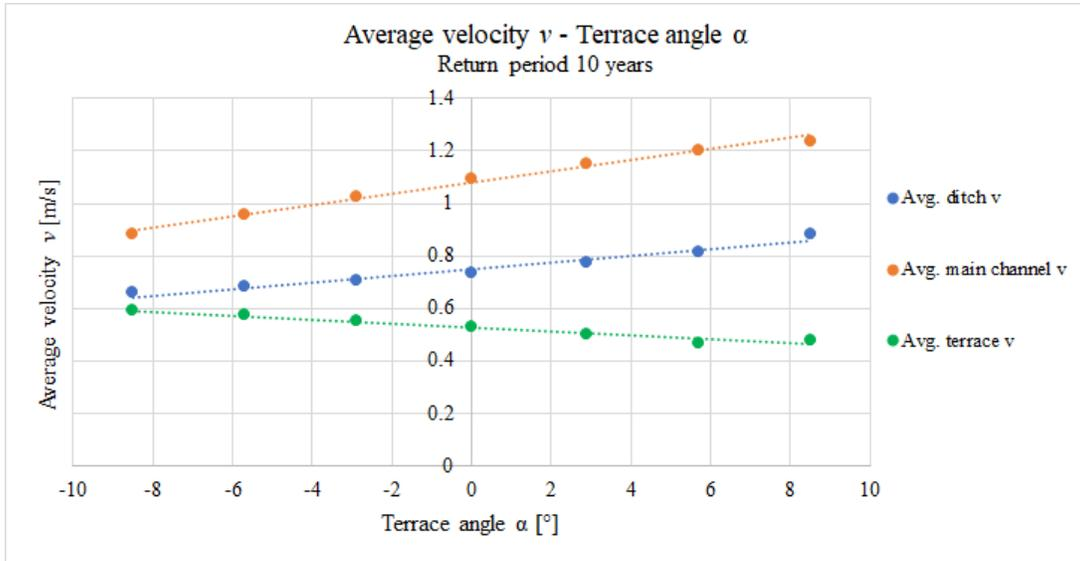
Figure E.2: Average velocity dependent on terrace angle with a 10 year return period in the theoretical two-stage ditch.
