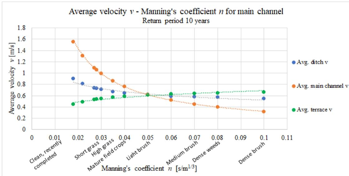
Figure G.2: Average velocity over Manning's coefficient in main channel, for 10 year return period in the theoretical two-stage ditch.
