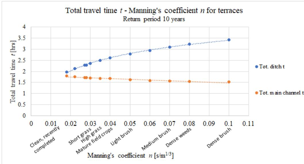
Figure F.1: Total travel time over Manning's coefficient varied on terraces. Used was return period of 10 years and the theoretical two-stage ditch.
