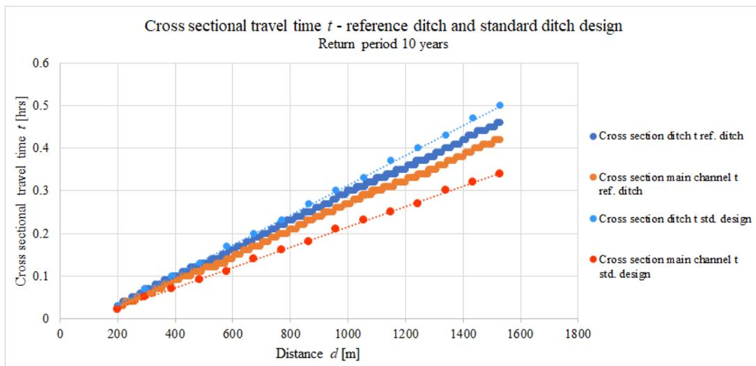
Figure H.1: Cross sectional travel time over distance of ditch, for a 10 year return period. Reference two-stage ditch and theoretical two-stage ditch are included.
