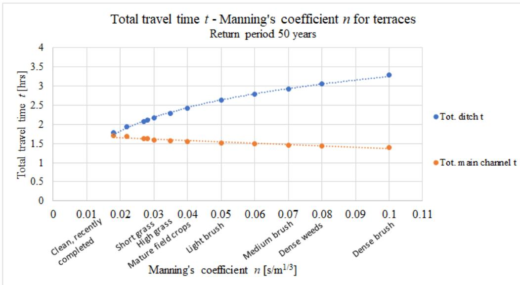
Figure F.3: Total travel time over Manning's coefficient varied on terraces with a 50 year return period in the theoretical two-stage ditch.
