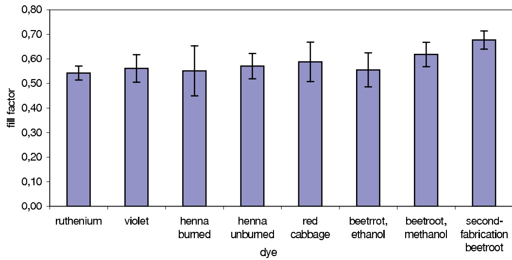
Figure 31: Average fill factor values and distribution ranges for different dyes.
