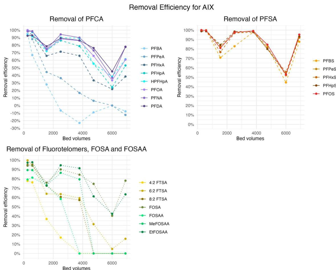
Figure 9. Removal efficiencies for PFAS after AIX during a 22 day long period. For PFCA and PFSA the dashed lines represent short chain and the solid lines represent long chain.
