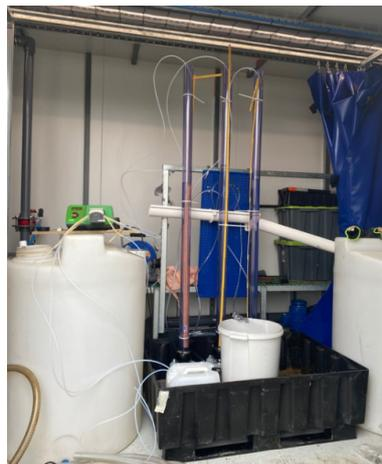
Figure 4. Photo of the set up for the column test with AIX and two stage GAC.
