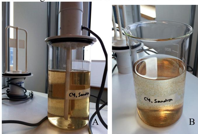
**Figure C1.** Figure A shows FeCl<sub>3</sub> experiment during slowly stirring with flocculator. Figure B shows samples after approximately 30 min of sedimentation.
