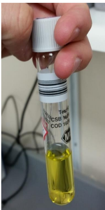
Figure 3. An illustration of the appearances of the small cuvettes used in the method Chloride determination and Chloride Elimination. Photo: Sandra Jonsson
