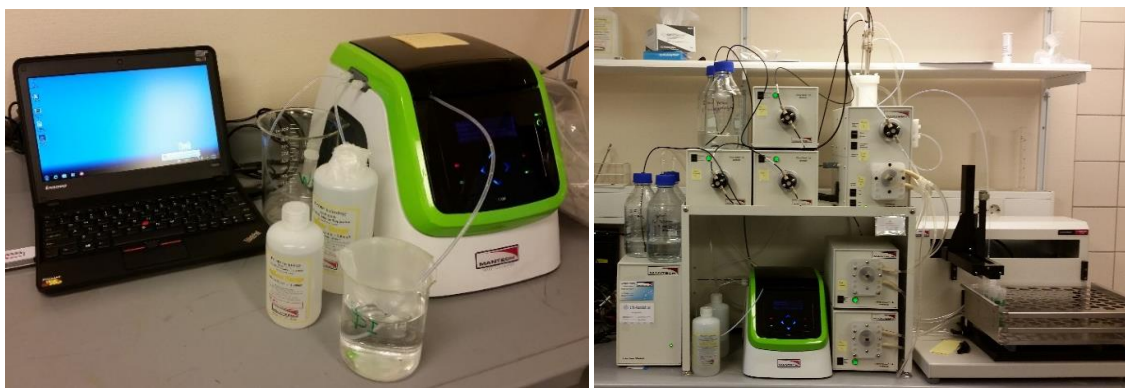
Figure 7. The manual PeCOD unit shown to the left and the automatic PeCOD system to the right, with attached pumps above and to the right of the PeCOD unit. To the right of the automatic PeCOD unit a sample holder is attached along with a sample arm used to transport sample solution from the rack into the vessel. Photo: Sandra Jonsson
