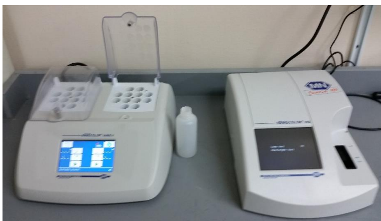
Figure 4. Instruments corresponding to both of the Macherey-Nagel methods, COD Chloride Determination and COD Chloride Elimination. The heating block used for digesting of the samples cuvettes on the left and the spectrophotometer used for measuring the final COD concentration in the sample to the right. Photo: Sandra Jonsson.
