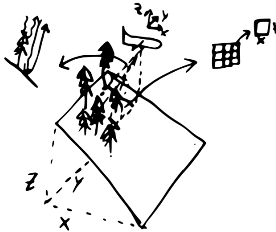
Figure 9. Sketch showing the airborne Lidar procedure. From the airplane, laser signals are sent toward the ground. The first returning signals represent the vegetation and the last the ground surface. The spatial position is corrected with a GPS station somewhere on the ground. The obtained data can then be interpolated and gridded to a DEM.
