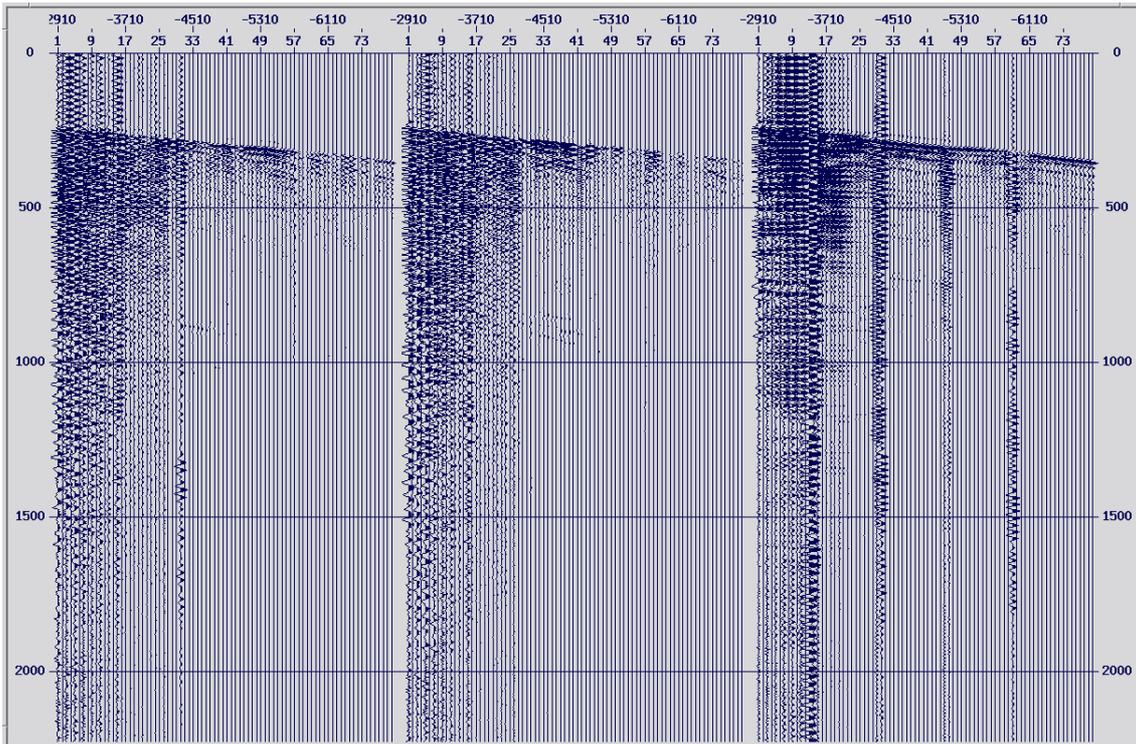
**Figure 16** Raw data from shot 4010 (offset=281,4 meters). H1, H2 and V component from left to right.
