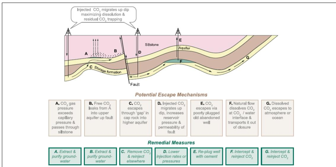
**Figure 6** Some potential escape routes for CO<sub>2</sub> injected into saline formations (IPCC, 2005).
