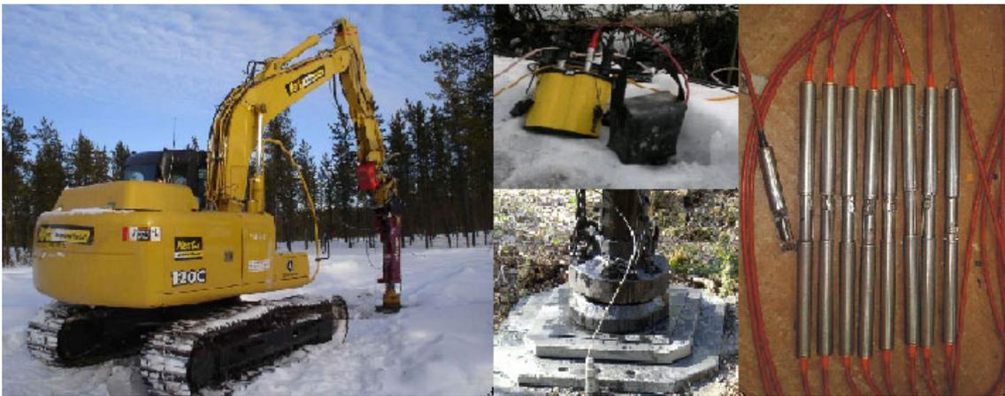
**Figure 14** VIBSIST 1000, channel DMT Summit II 24 bit distributed acquisition system and a 3 component R8XYZ-cg geophone chain from left to right (Surface Geophysics (WP 6.3): VSP/MSP Baseline, 2008).
