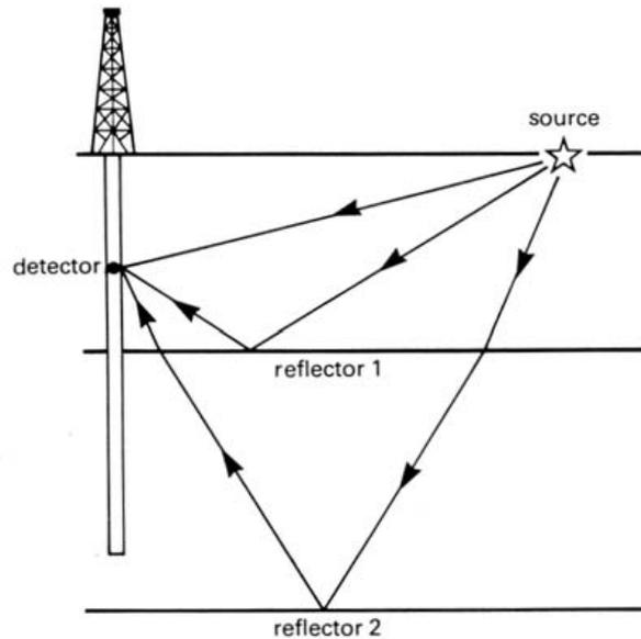
**Figure 2** Typical offset VSP measurement (Kruk, 2005).
