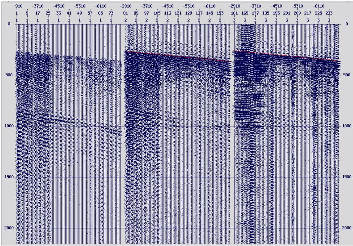
Figure A3 Shot 7033 after rotation. H1, H2 and V component from left to right.
