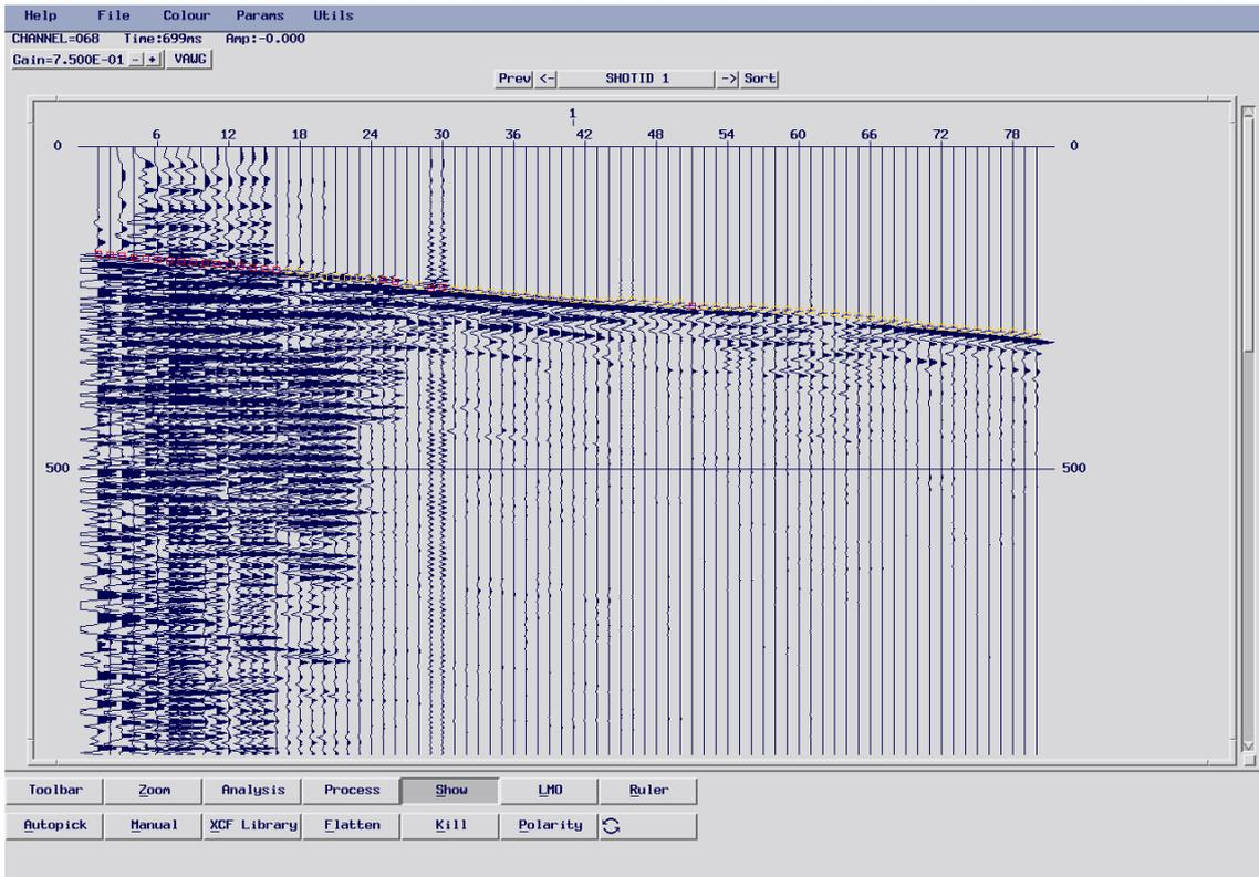
**Figure A9** The pick first break tool in Claritas. Yellow picks represents automatically picks while red picks are manual picks.
