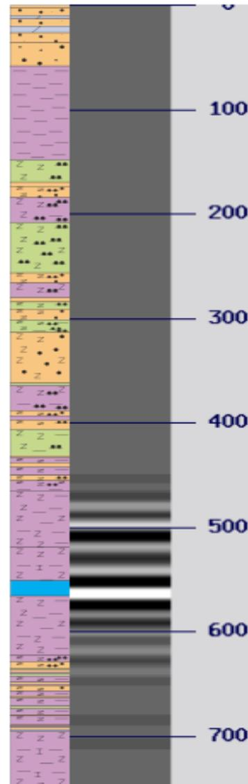
**Figure 19** Correlation between borehole stratigraphy and depth converted zero-offset VSP (see Figure 9 for more detailed explanation).
