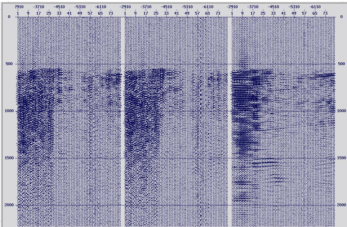
**Figure 17** Raw data from shot 6084 (offset=1144,3 meters). H1, H2 and V component from left to right.
