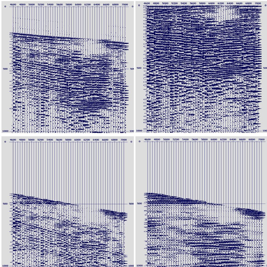
**Figure 18** Seismogram of zero-offset shot. Top left: Before shift of first arrival. Top right: After align coherent downgoing energy horizontal, using shift of first arrival. Bottom left: After horizontal velocity filter of downgoing events plus opposite shift of first arrival. Bottom right: Upgoing events after positive velocity filtering of horizontal events.
