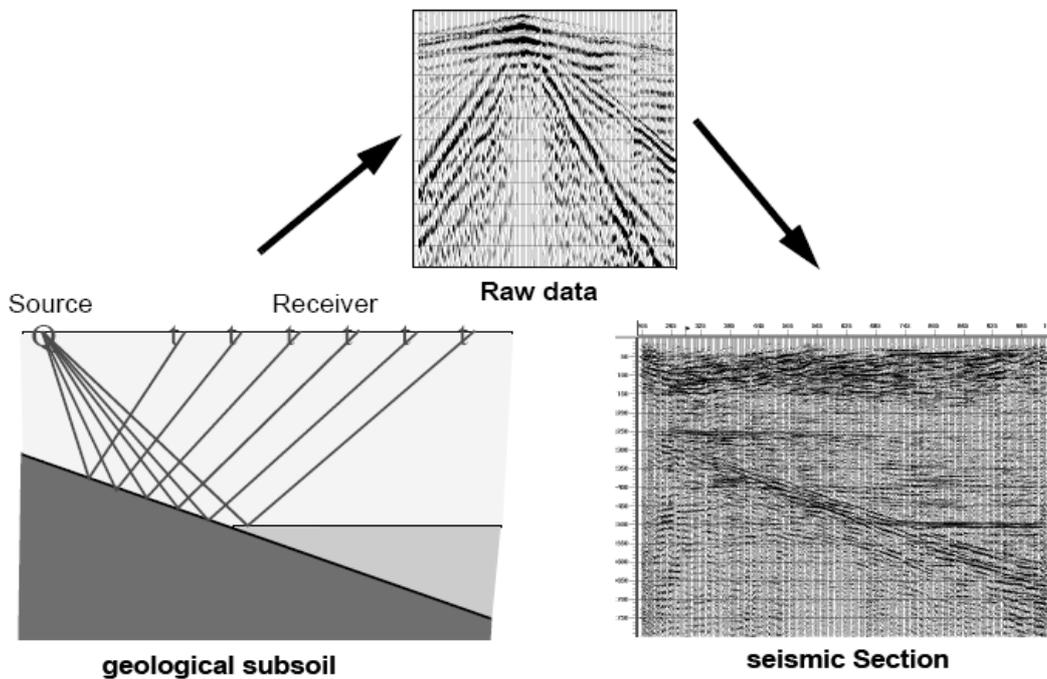
**Figure 1** Schematic picture over the seismic methodology (Kruk, 2005).
