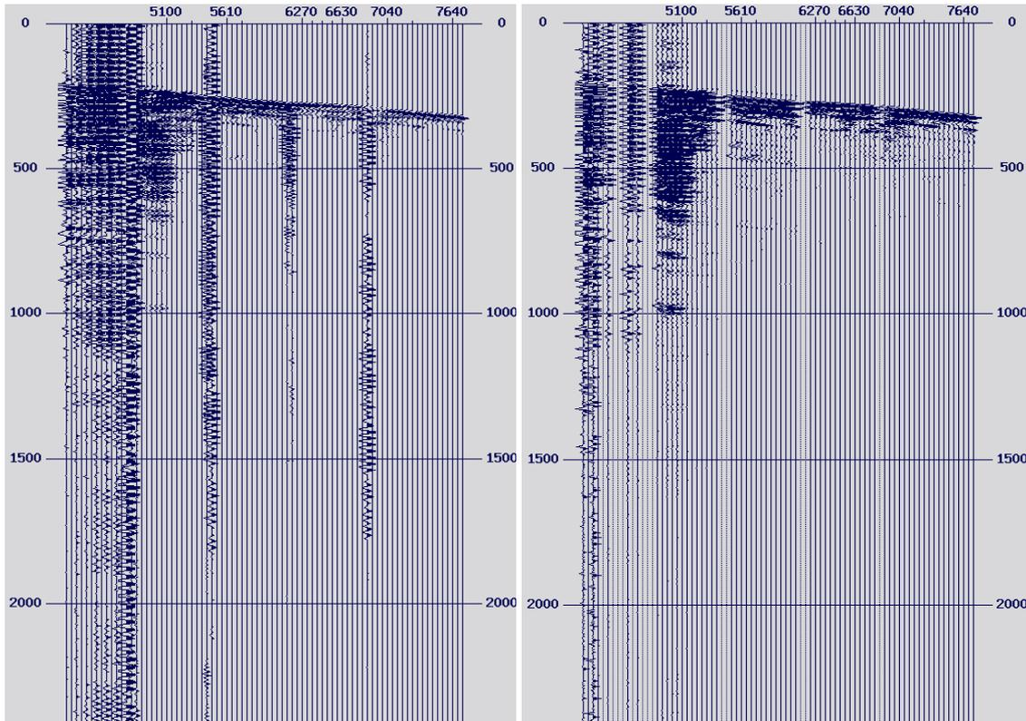
**Figure A5** V component of shot 4010 after bulk static shift and refraction static.
