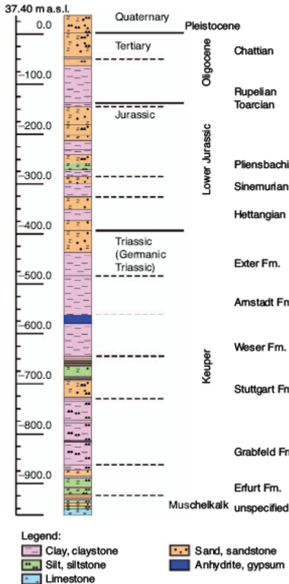
**Figure 9** Stratigraphy of the Ketzin area based on drilling of the Ktzi 169/63 borehole (Juhlin et al., 2007).
