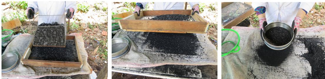
Figure 5: Sieves used to separating charcoal: 13 mm basket (left), 4 mm (middle) and 1,7 mm (right). Authors' pictures.
