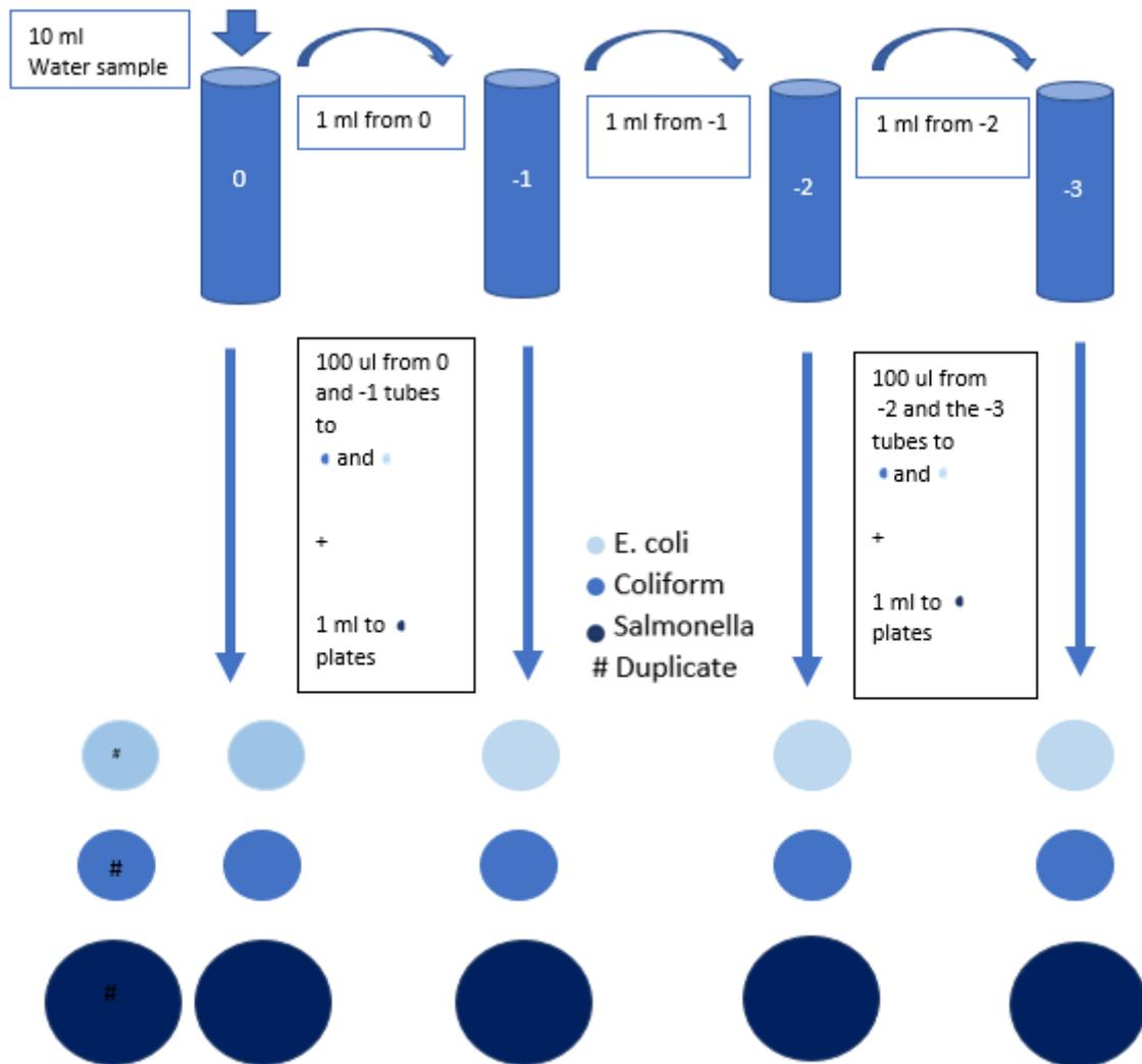
Figure 10: Dilution example procedure
