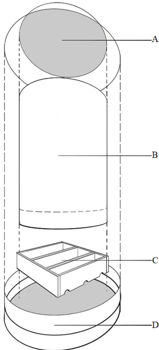
Figure 4: Sketch of the vertical garden. A= Top basin, B=The charcoal filled sack, C= Wooden drainage construct, D= Bottom basin with effluent tap. Authors figure.
