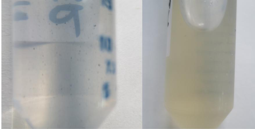
Figure 22: Visual difference between effluent water (left) and influent water (right). The presence of charcoal is visible in the effluent water samples.
