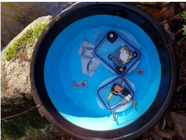
**Figure 4:** Inside of the chamber at site 7. The white and gold device is the CO<sub>2</sub> sensor. It is connected to a 9 V battery and a cable to collect data. When the chamber was in use, the sensor, battery and cable were protected with plastic casings. The diameter of the chamber was 30 cm.
