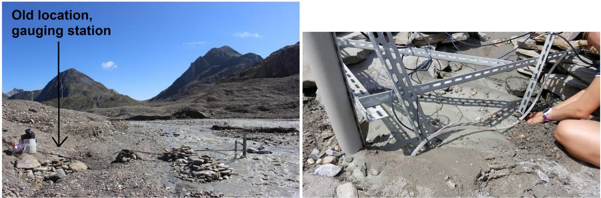
**Figure 15:** To the left, picture taken on 15.08.2017 showing the old placement of the gauging station and the new location of Stream 1. To the right, the sensors were completely covered by sediments and rocks after the flood event. Photograph: Marie Selenius.
