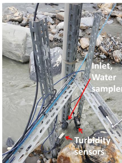
**Figure 7:** Picture taken during extremely low flow on 07.09.2017 showing the locations of the sensors. Picture by Marie Selenius.
