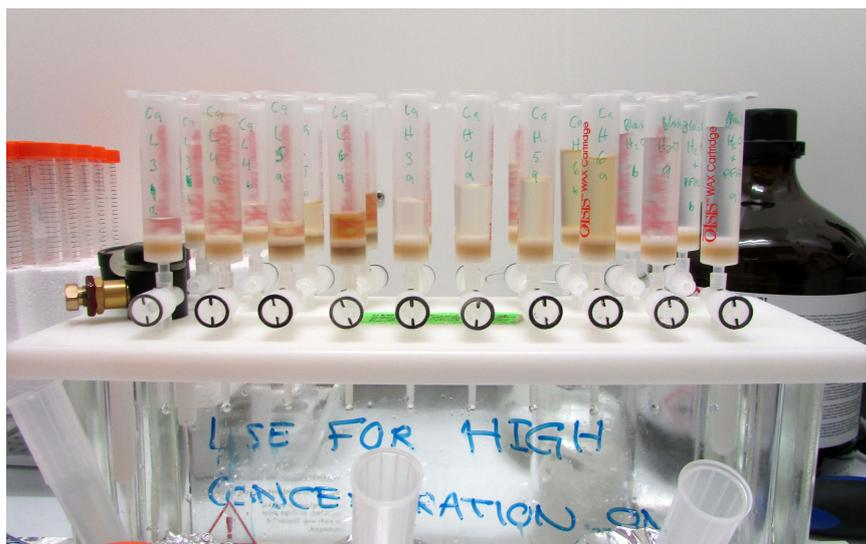
Figure 1. Samples loaded into SPE cartridges mounted to a manifold.
