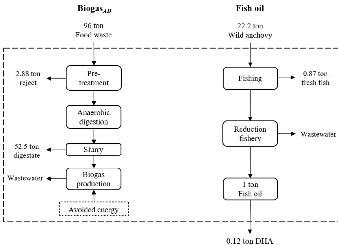
Figure 10: The Fish scenario includes production of fish oil and biogas. Additional energy and water is needed but excluded in this illustration.
