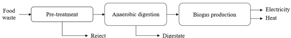
Figure 1: Simplified process for biogas production from food waste, when used to produce electricity and heat. Additional energy, water, transports and processing units are excluded in this illustration.
