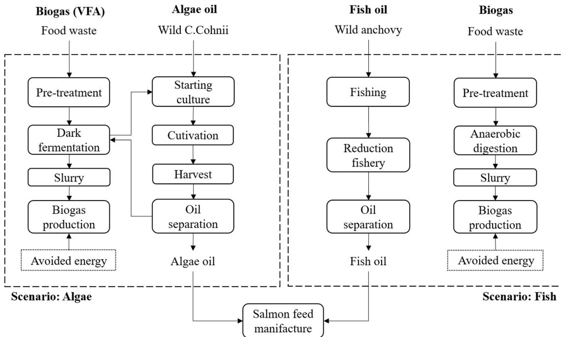
Figure 8: A process overview of assessed DHA production, illustrating the comparison between the Algae scenario and Fish scenario. The system boundary is illustrated as a dashed line and the dotted lines surround by-products included via system expansion.
