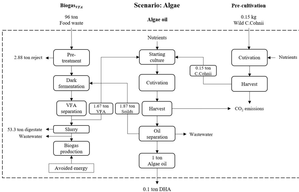
Figure 9: The Algae scenario includes production of algae oil and biogas with VFA extraction. Additional dark energy and water is needed but excluded in this illustration.
