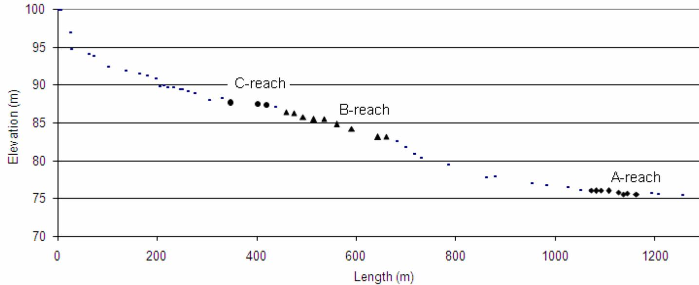
**Figure 1** Longitudinal profile of the river reach between the foot of the dam at Ljusnaren and the confluence with the diverted water downstream the hydropower station. The location and elevation of the three modelled reaches are marked. The foot of the dam is assigned the elevation 100 m, which corresponds to about 160 m above sea level.
