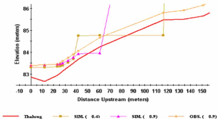
**Figure 13** Water surface elevation simulated for B-reach with WSP. Thalweg elevation, observed water surface elevation, and simulated water surface elevations.
