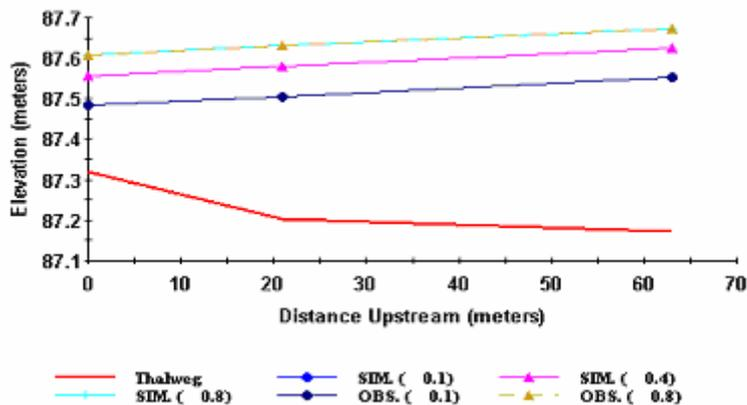
**Figure 12** Water surface elevation profile simulated for C-reach with STGQ.
