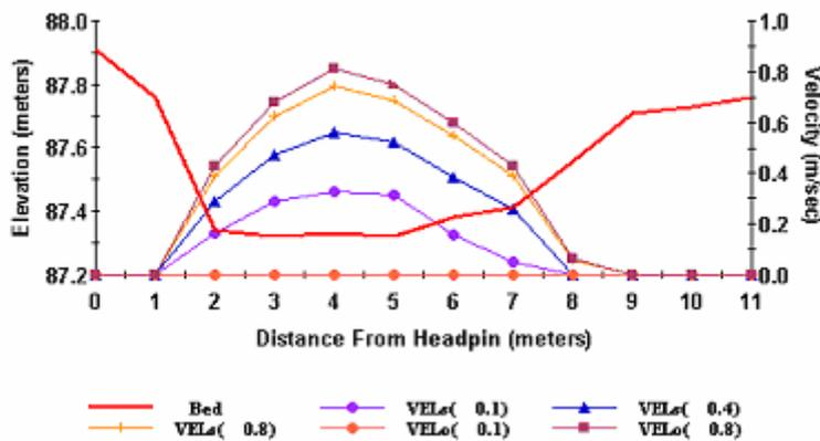
**Figure 14** Measured and simulated velocity profiles and river bed geometry at the C-transect furthest downstream.
