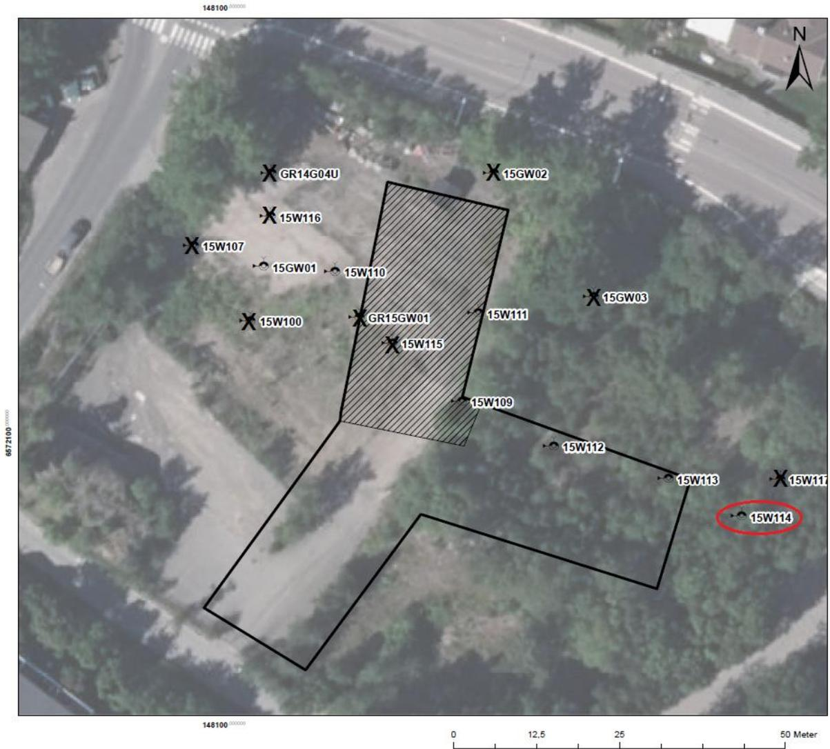
Figure 42. The groundwater pipe 15W114 is marked in red, and the groundwater pipes not part of the observations are marked with a cross. The figure is based on WSP:s figure of the area.
