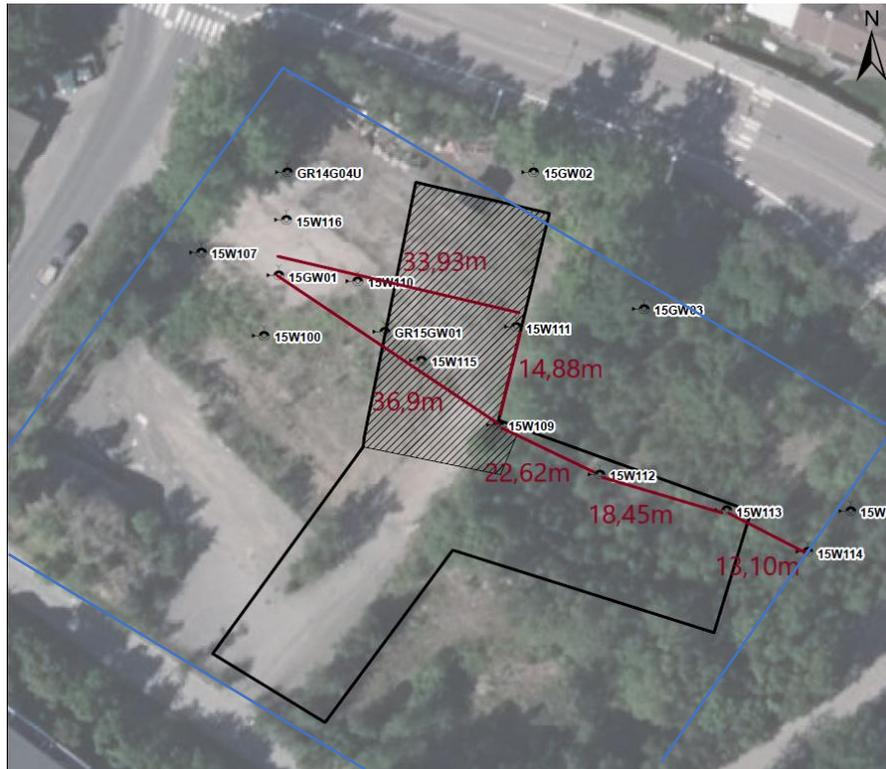
Figure 20. Distances between the different groundwater pipes. Based on a picture by WSP, 2016a.
