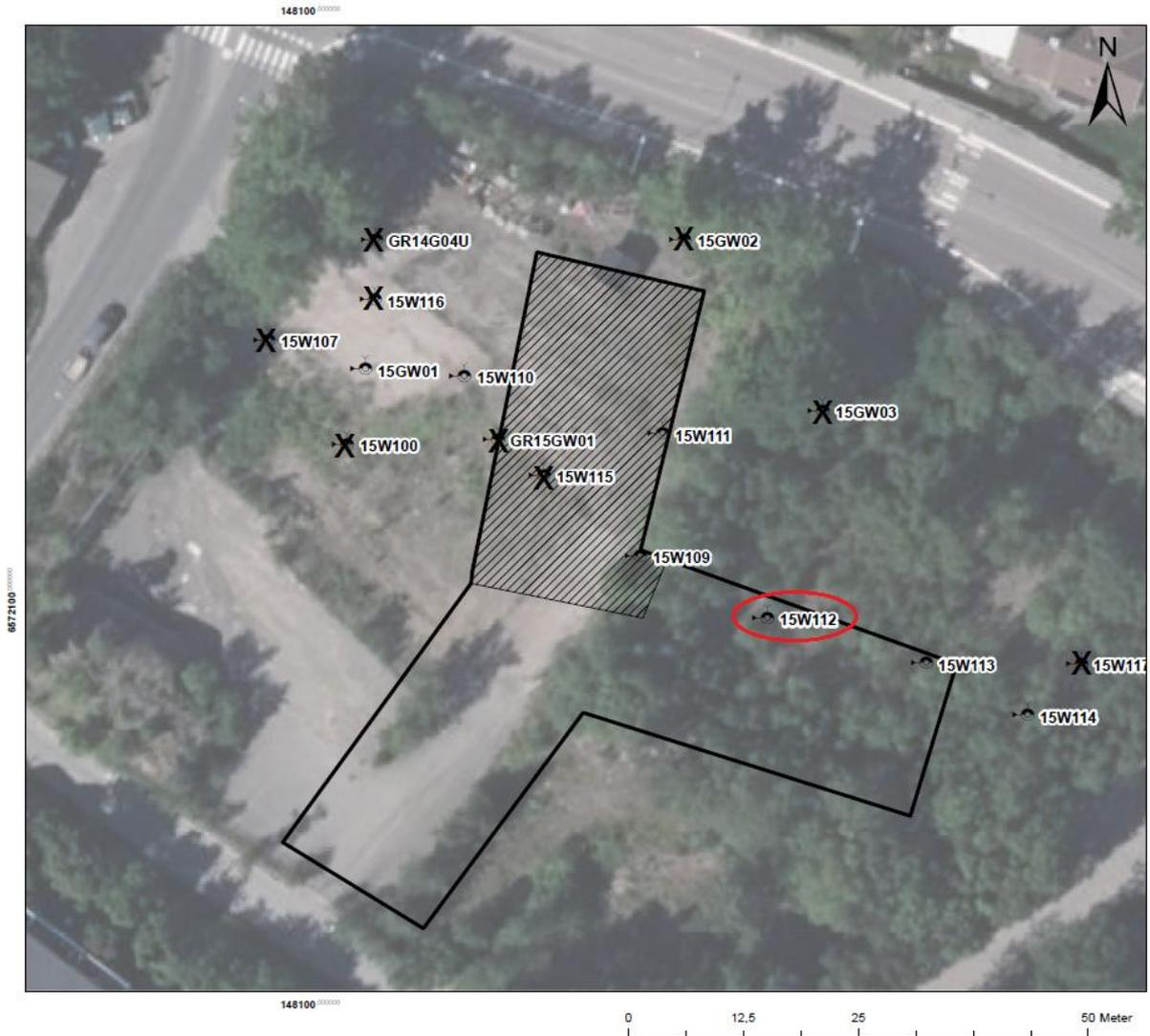
Figure 38. The groundwater pipe 15W112 is marked in red, and the groundwater pipes not part of the observations are marked with a cross. The figure is based on WSP:s figure of the area.
