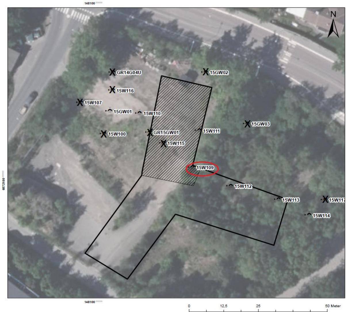
Figure 36. The groundwater pipe 15W109 is marked in red, and the groundwater pipes not part of the observations are marked with a cross. The figure is based on WSP:s figure of the area.
