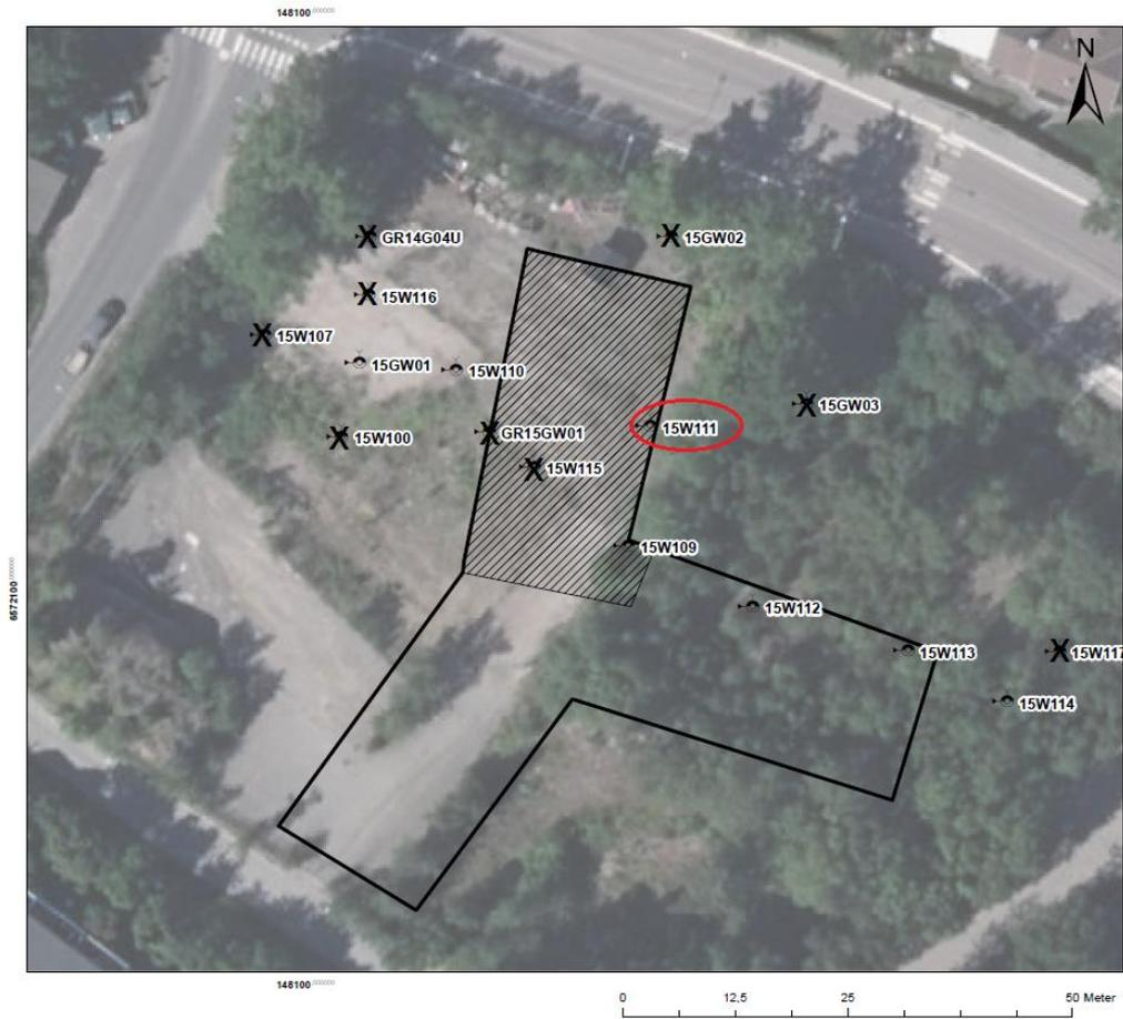
Figure 34. The groundwater pipe 15W111 is marked in red, and the groundwater pipes not part of the observations are crossed over. The figure is based on WSP:s figure of the area.
