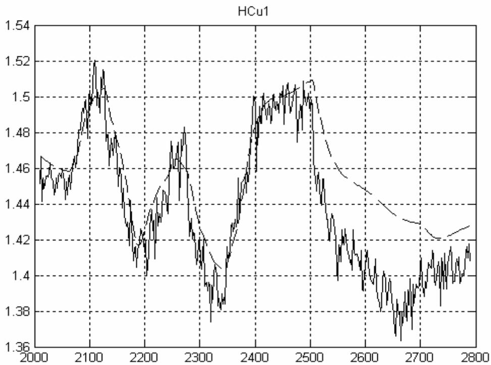
**Figure 5.6** The simulated output (dashed) from the model HCu1 compared with the measured output from the validation data set, BS2 (solid). The estimated parameters of model HCu1 was rounded off to three significant digits.
