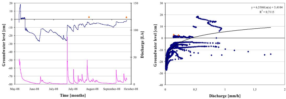
Figure F: Hydrological data evaluation for site 8.
