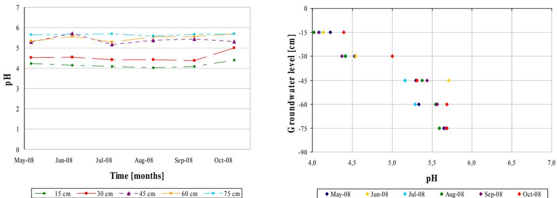
Figure III: pH value variations at the different sampling depths for site 7.
