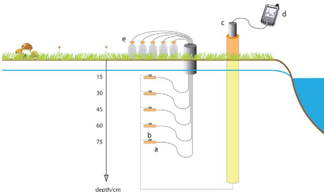
**Figure 4:** Principle sketch of the measurement equipment and its placement in the field, a – suction lysimeter, b – temperature probe, c – groundwater capacitance probe, d – recording instrument, e – sampling bottle.
