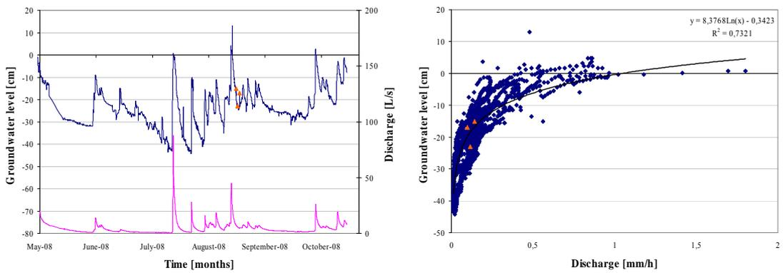
Figure G: Hydrological data evaluation for site 10.
