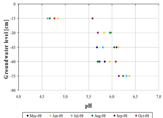
Figure X: pH value variations at the different sampling depths for site 9.
