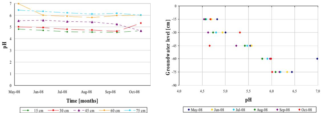
Figure II: pH value variations at the different sampling depths for site 6.
