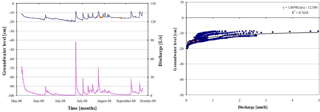
**Figure C:** Hydrological data evaluation for site 6.
