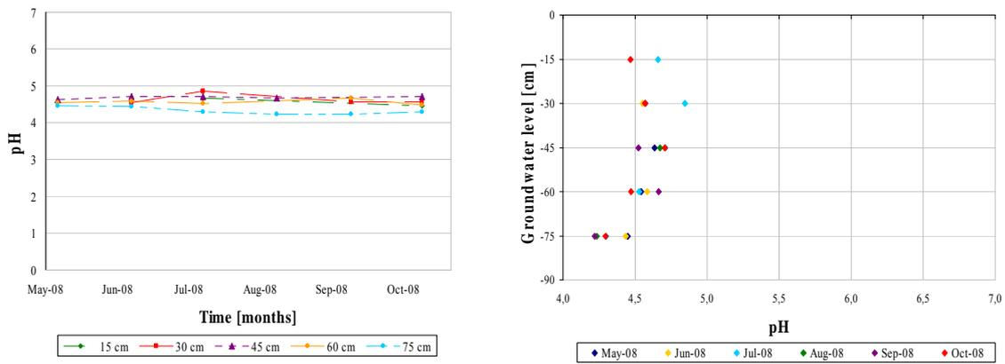
**Figure V:** pH value variations at the different sampling depths for site 8.
