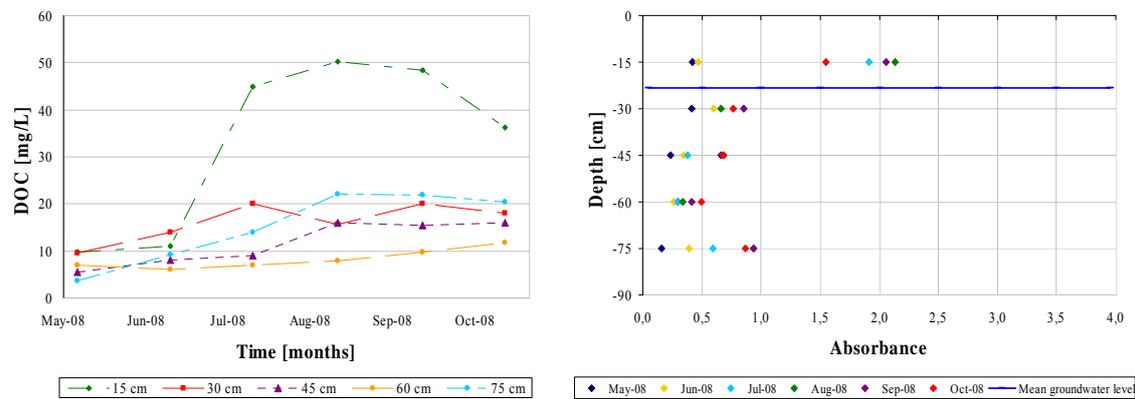
**Figure vi:** Variations in DOC (left) and absorbance (right) at the different sampling depths for site 10.
