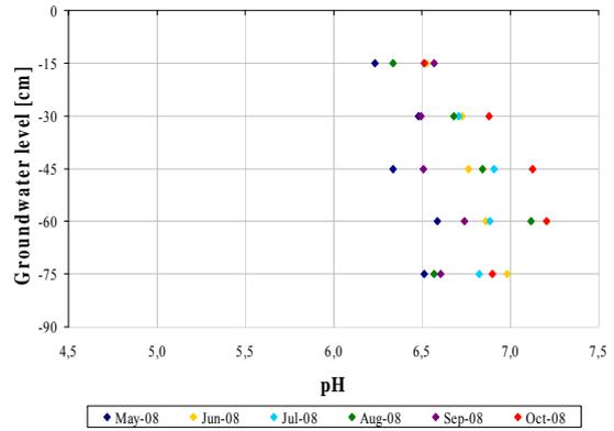
Figure VII: pH value variations at the different sampling depths for site 11.
