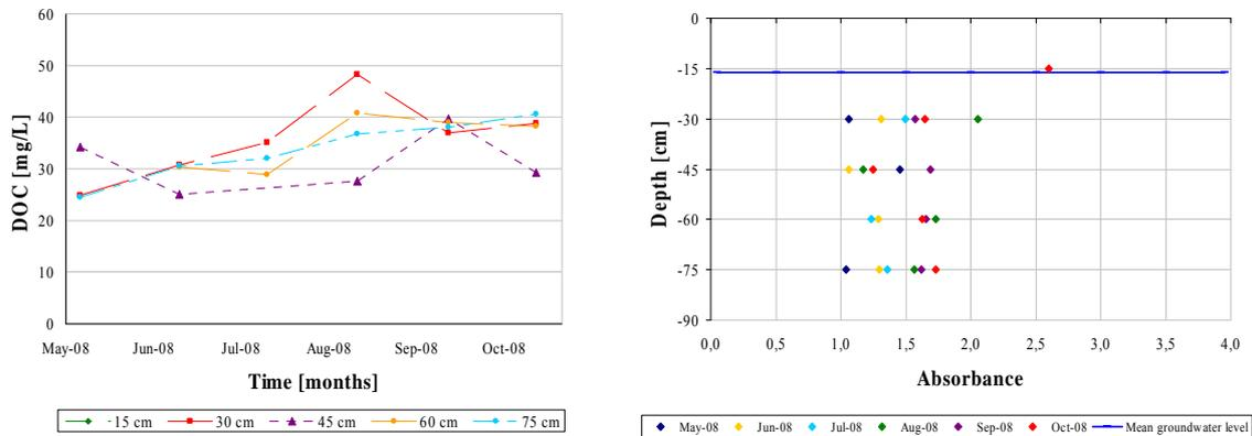
**Figure iv:** Variations in DOC (left) and absorbance (right) at the different sampling depths for site 2.
