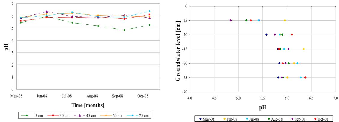
**Figure VI:** pH value variations at the different sampling depths for site 10.
