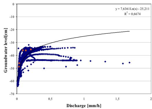
**Figure J:** Hydrological data evaluation for site 9.
