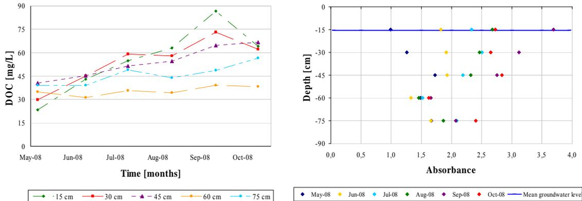
**Figure 15:** An example of the DOC and absorbance profiles representative of group *forest*, based on site 6, showing DOC variations throughout the sampling period (left) and a vertical absorbance profile (right).
