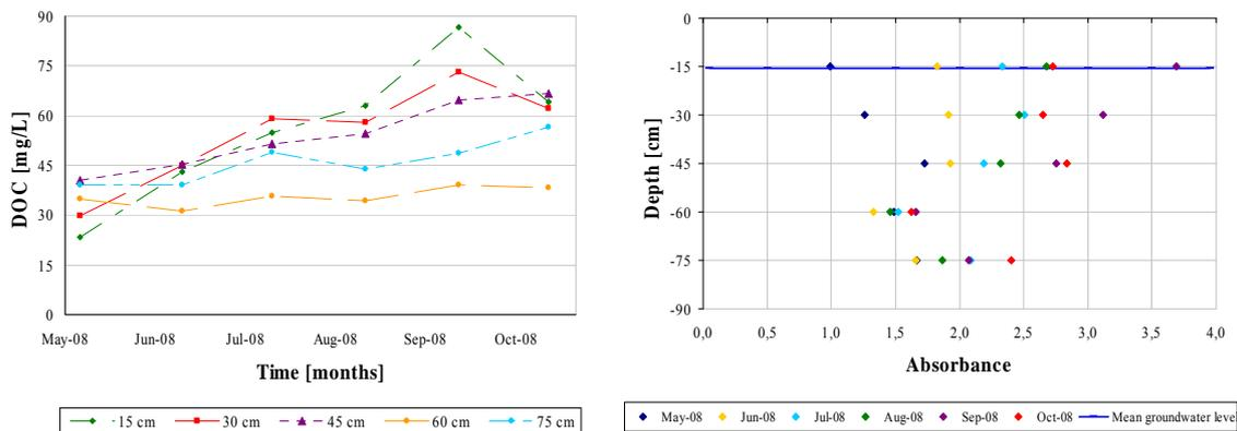
Figure ii: Variations in DOC (left) and absorbance (right) at the different sampling depths for site 6.
