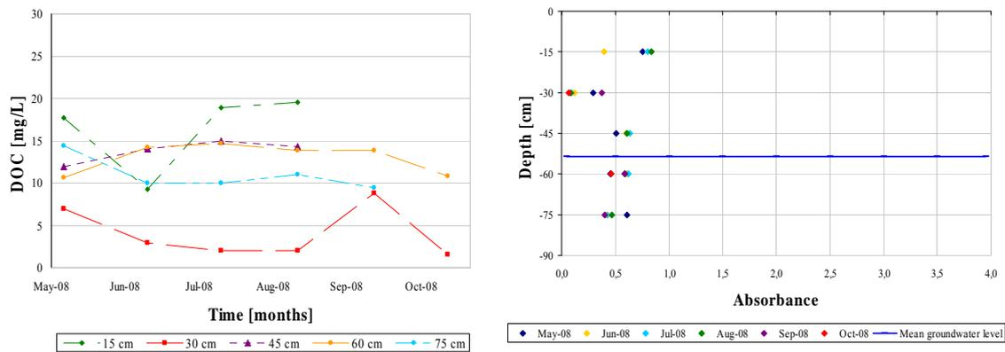
Figure viii: Variations in DOC (left) and absorbance (right) at the different sampling depths for site 1.
