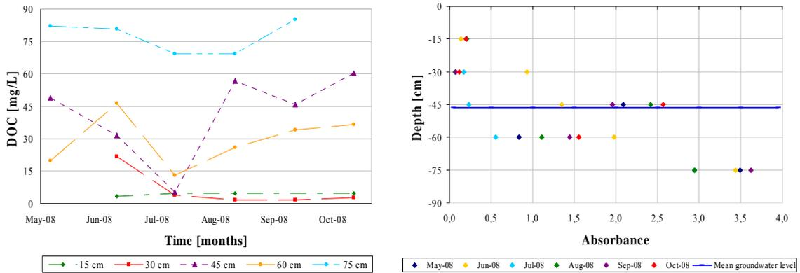
Figure x: Variations in DOC (left) and absorbance (right) at the different sampling depths for site 9.
