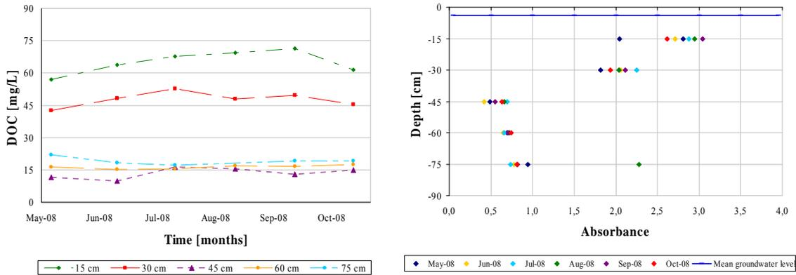
Figure vii: Variations in DOC (left) and absorbance (right) at the different sampling depths for site 11.
