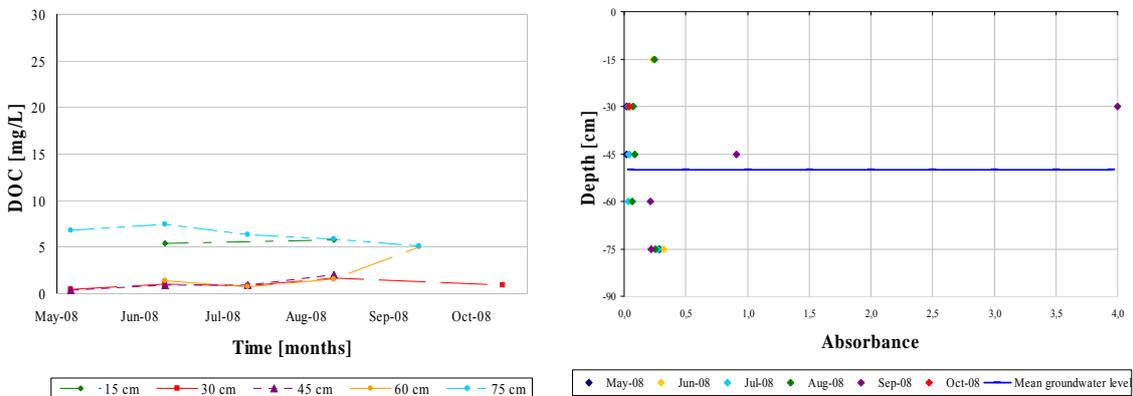
Figure ix: Variations in DOC (left) and absorbance (right) at the different sampling depths for site 4.
