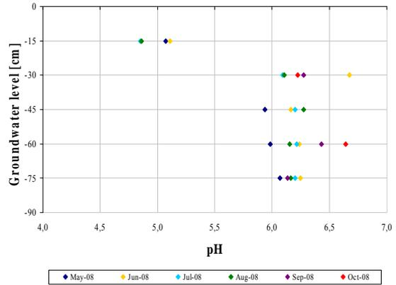
Figure VIII: pH value variations at the different sampling depths for site 1.
