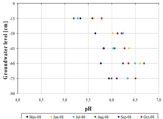
Figure XI: pH value variations at the different sampling depths for site 12.
