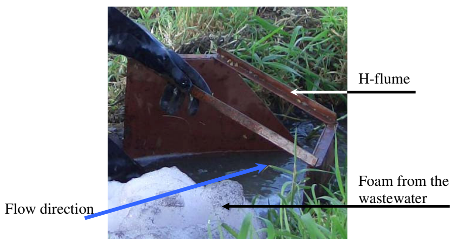
Figure 4. A H-flume measuring the flow in a small irrigation canal at a basin irrigated farm. Photographer Charlotta Hofstedt, 2004.
