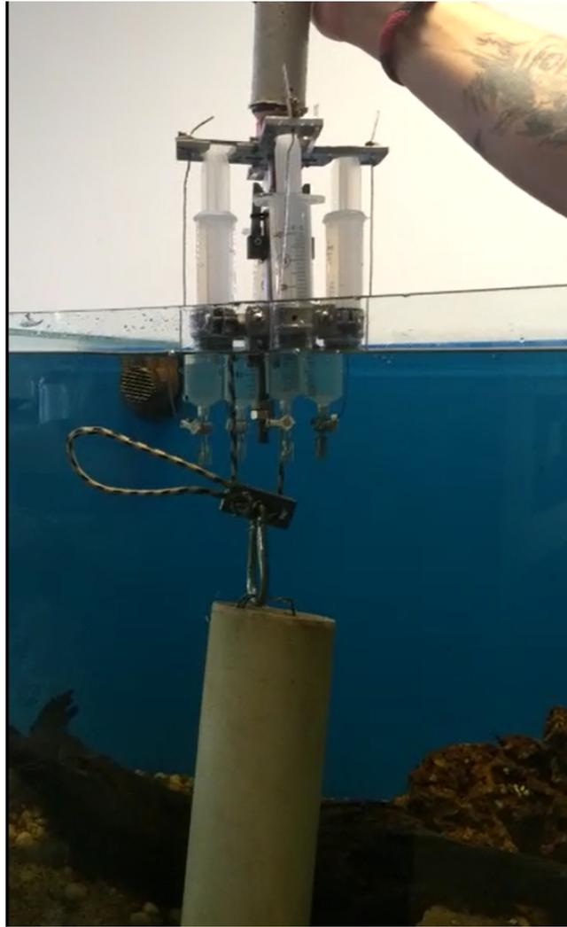
Figure 5. Deep-water sampler being tested in aquarium
