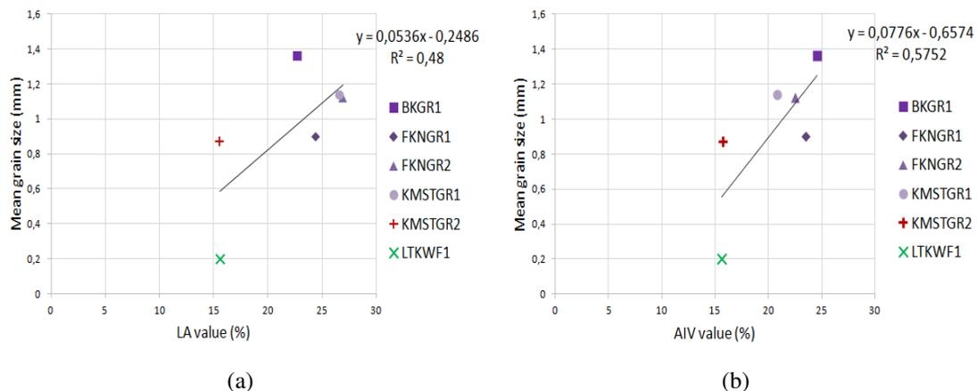
Figure 25: a) The LA value tend to correlate with mean grain size. Low mean grain size seems to give low LA value. b) AIV value tend to correlate with mean grain size. Low mean grain size seems to give low AIV value.
