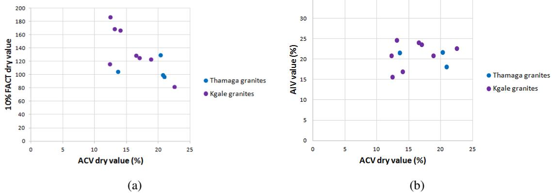
Figure 18: a) The 10 % FACT and ACV values tend to have a significant negative correlation, this according to closely related test methods. b) AIV and ACV values tend to have a weak correlation.
