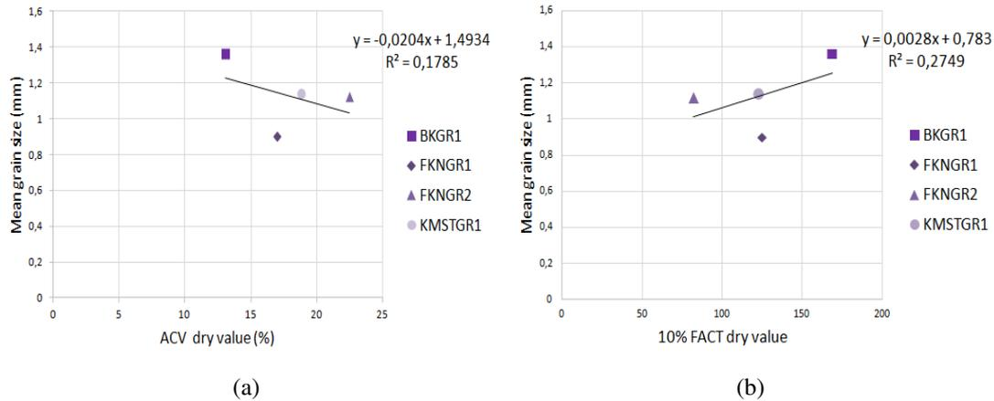
Figure 24: a) The ACV tend to have a weak correlation with the mean grain size. A low mean grain size seem to give high a ACV. b) The mean grain size tend to have a weak correlation with the 10 % FACT value. A low mean grain size seem to give a low 10 % FACT value.
