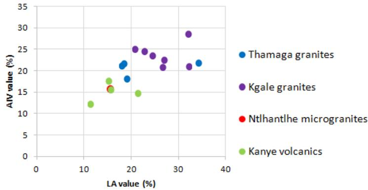
Figure 14: The aggregate impact values and Los Angeles values tend to have a positive correlation.
