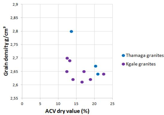
Figure 31: Grain density and ACV value for Thamaga and Kgale granites.
