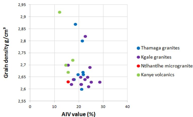
Figure 17: Figure show grain density and AIV value for all granite types. Higher density tend to give lower AIV value.
