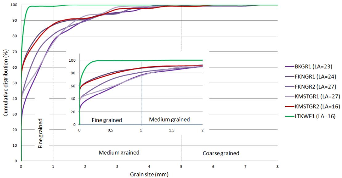
Figure 28: Grain size distribution curve with LA value in parenthesis next to each sample
