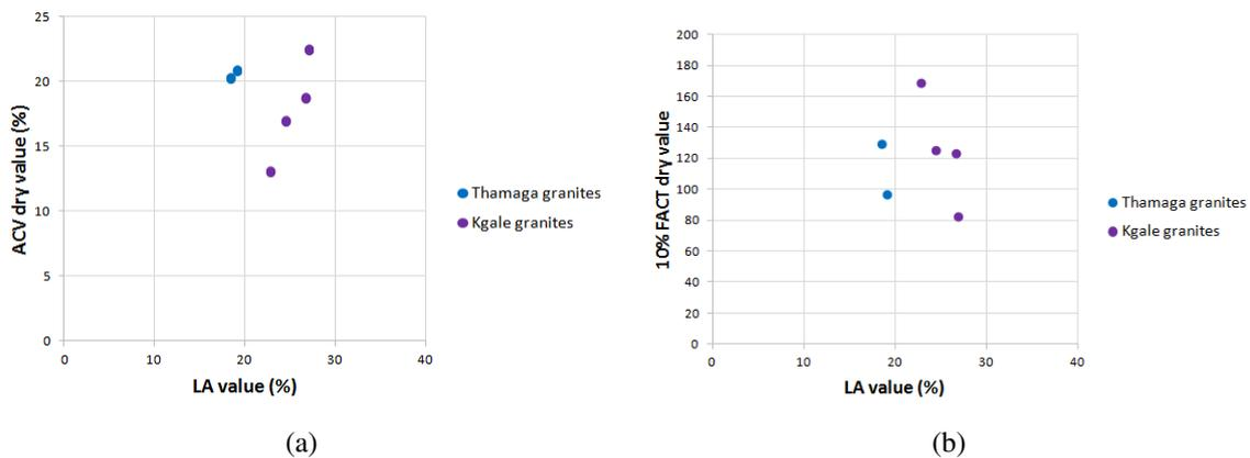
Figure 15: a) The aggregate crushing values and Los Angeles values tend to have a positive correlation, similar to[?]. b) Figure shows 10 % FACT and LA value for Thamaga and Kgale granites. No obvious correlation.
