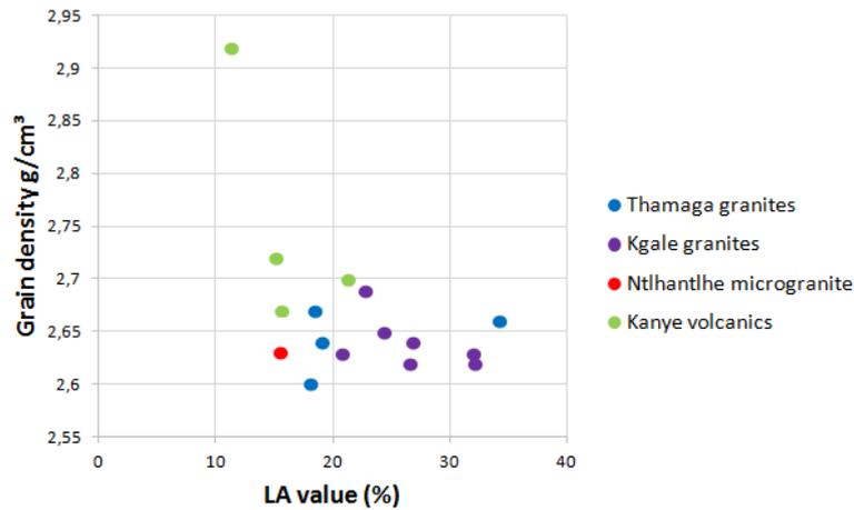
Figure 16: Figure show grain density and LA value for all granite types. Higher density tend to give lower LA value.
