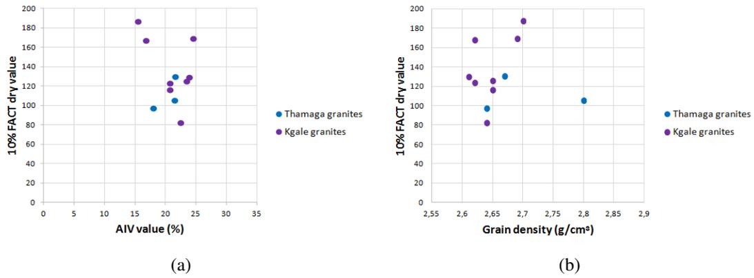
Figure 30: a) 10 % FACT value and AIV value for Thamaga and Kgale granites. b) 10 % FACT value and grain density for Thamaga and Kgale granites.
