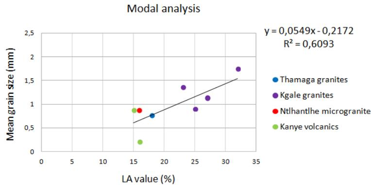
Figure 26: The LA value from the modal analysis tend to correlate well with mean grain size,  $R^2 = 0.61$ . Low mean grain size seems to give low LA value.
