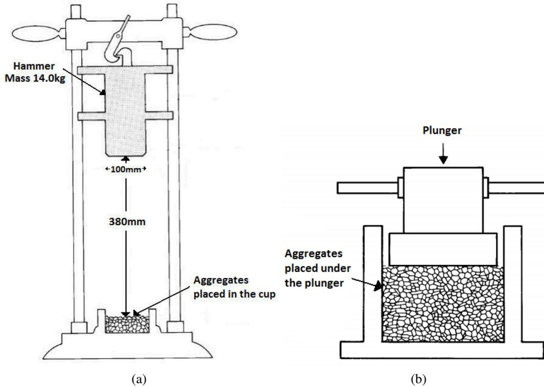
Figure 8: a) Apparatus for the aggregate impact value test, Modified from Millard (1993).
