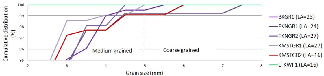
Figure 29: Grain size distribution curve which only show the upper limits (95 %-100 % cumulative distribution). The Fikeng FKNGR1 contain the largest grains.
