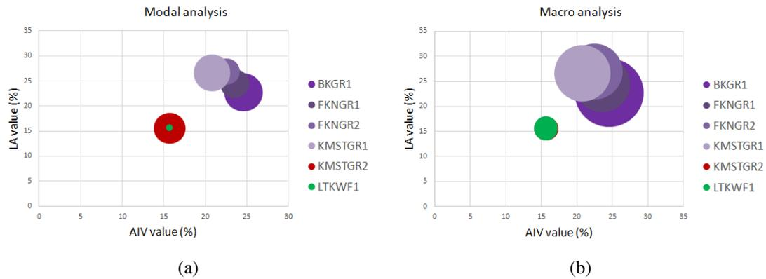
Figure 32: a) The LA value correlates with the AIV and mean grain size of the modal analysis. b) The LA value correlates with the AIV and mean grain size of the macro analysis. The mean grain size corresponds to the size of the circles, larger circle diameter correlates to larger mean grain size.
