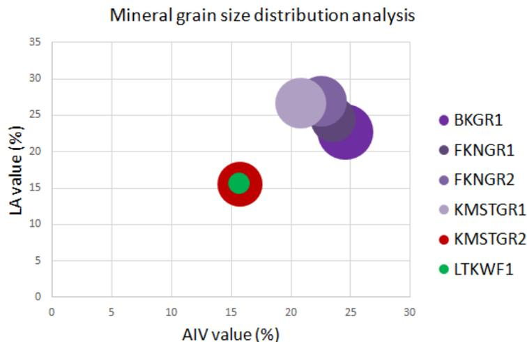
Figure 27: The LA value correlates with the AIV and mean grain size of mineral grain size distribution. The mean grain size corresponds to the size of the circles, larger circle diameter correlates to larger mean grain size.
