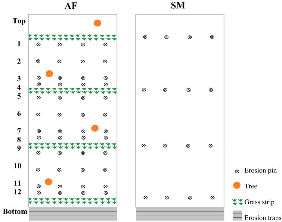
Figure 9. Illustration of the plot design in the Son La trial. The AF plot was designed with four grass strips and twelve rows of erosion pins with four pins in each row. The AF plots also had four trees, placed above each grass strip. The species were Longan and Mango, alternating between the rows with Longan placed in the top of the plot. The SM plot was designed with four rows of erosion pins, located in the height of the grass strips in the AF plot.
