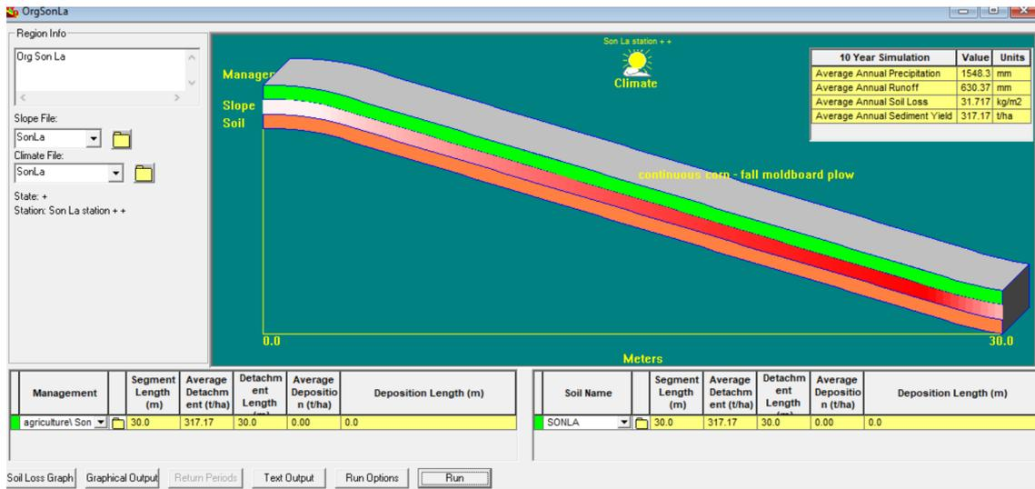
Figure 27. The result screen in WEPP for a simulation of a SM plot in Son La over a period of 10 years. Total soil loss is 317 t ha<sup>-1</sup>.
