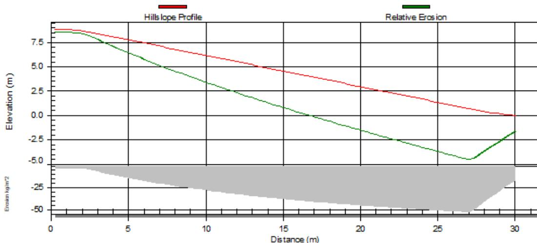
Figure 28. Output graph from WEPP showing the actual slope surface (red), the soil detachment (green) and the actual erosion [kg m<sup>2</sup>] (grey area). A 10 year-simulation with the WEPP model gave a total soil loss of 317 t ha<sup>-1</sup>.
