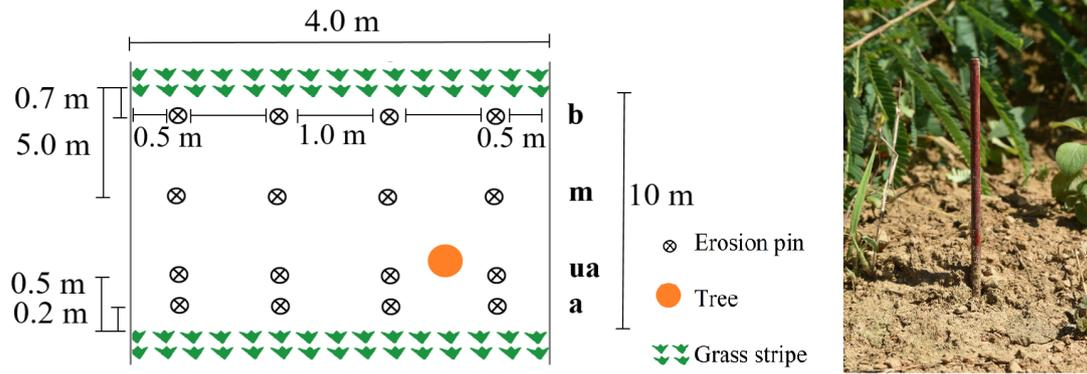
Figure 8. Figure (to the left) illustrating the positions of the erosion pins in one section in the AF experimental plots in both sites. The four positions in one section are below the grass strip (b), in the middle of two grass strips (m), upper above the grass strip (ua) and above the grass strip (a). Photo of an erosion pin (to the right).
