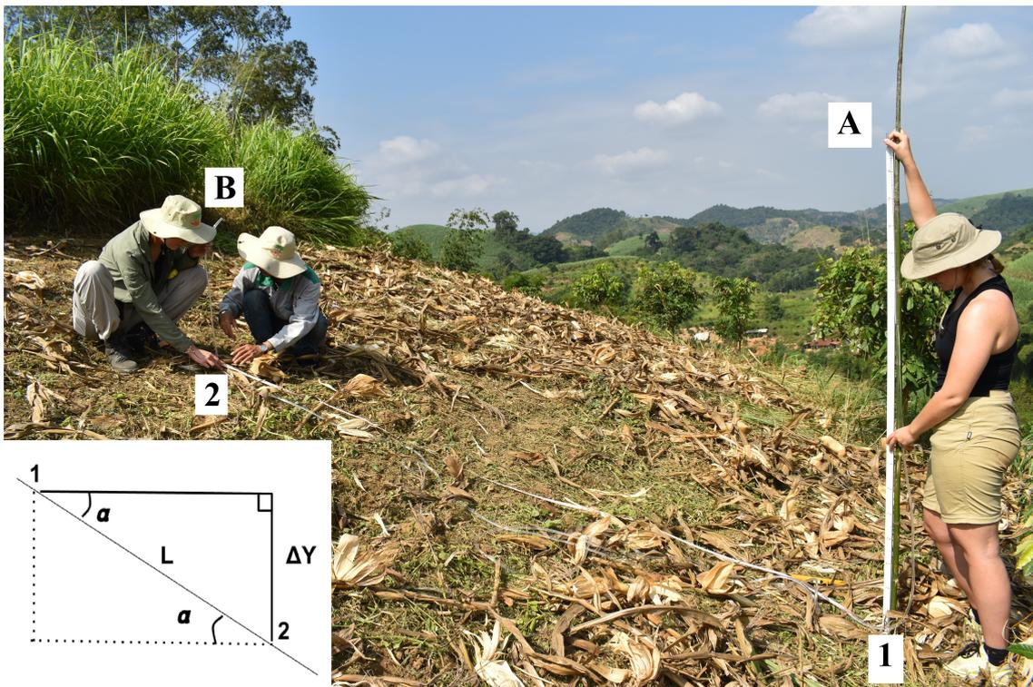
Figure 7. Demonstration of the method set up to evaluate the slope gradient.
