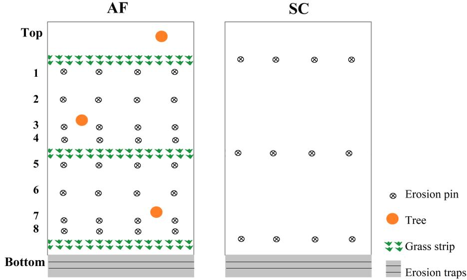
Figure 10. Illustration of the plot design in the Dien Bien trial. The AF plot was designed with three rows of grass strips and eight rows of erosion pins, with four pins in each row. There were also three Son tra trees, one above each grass strip. The SC plot was designed with three rows of erosion pins, located in the height of the grass strips in the AF plots.
