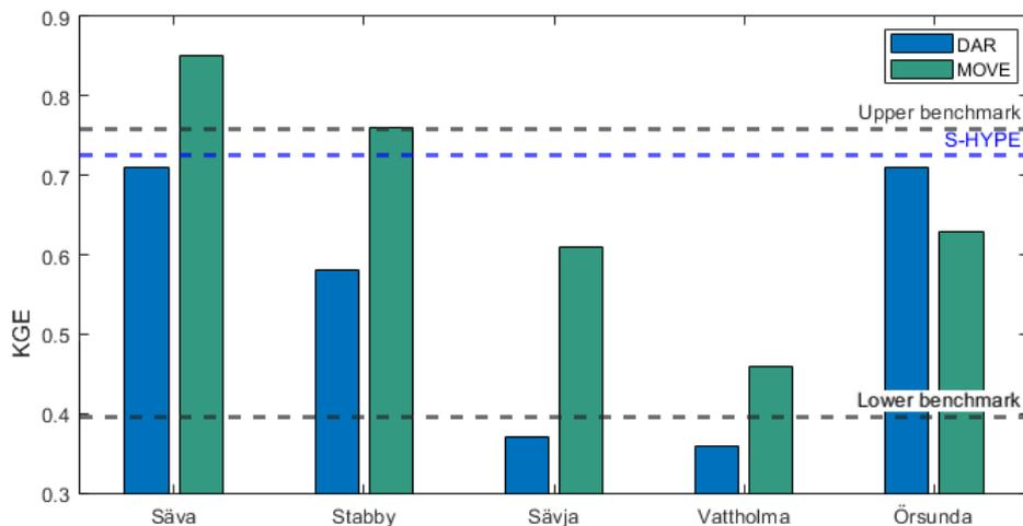
**Figure 5.** The performance of the two index methods measured in KGE. The blue bar shows the performance of the DAR method, while the green bar shows the MOVE method. The lines represents different benchmarks used in the project.
