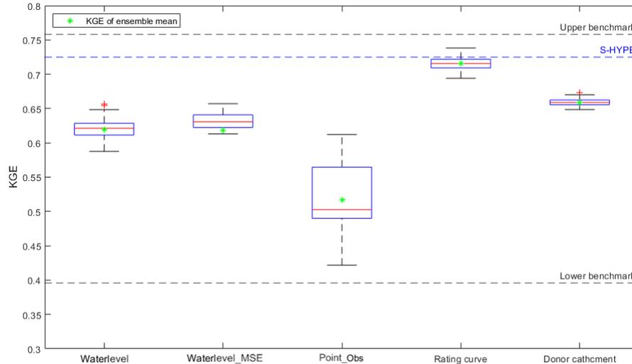
**Figure 8.** *The distribution of performance (measured in KGE) for the different HBV calibration-methods. All boxes are based on 100 simulations (100 values) except for `Waterlevel_MSE`, which is based on 10 simulations. The lines represents different benchmarks used in the project.*
