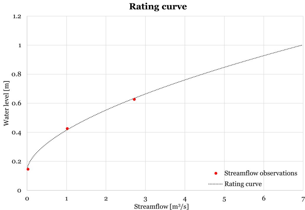
**Figure 14.** *The rating curve for Håga catchment created for this project.*
