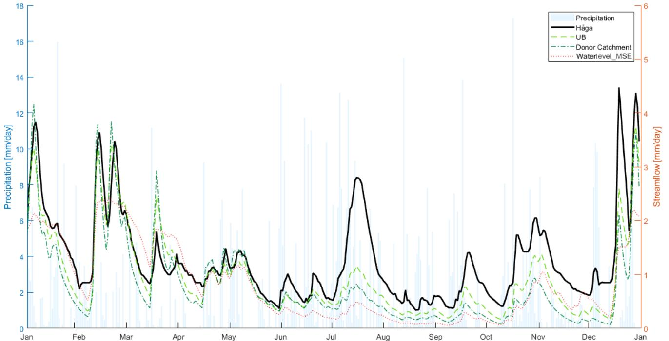
**Figure 10.** Hydrographs for the year 1998 for some of the HBV-calibration-methods.
