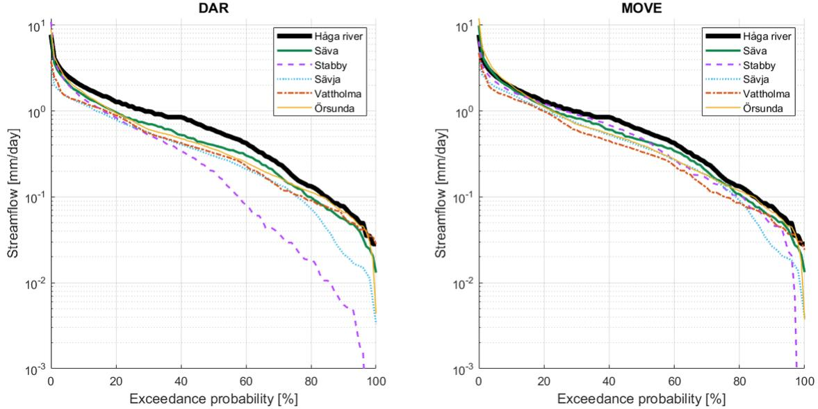
**Figure 6.** Flow duration curves for the two index-methods. The thick black line is the actual FDC of Håga river for the evaluation period.
