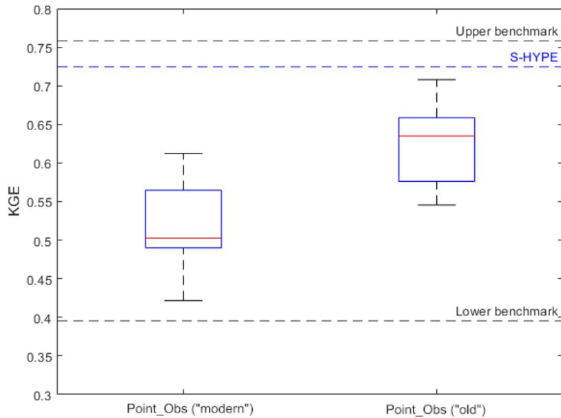
**Figure 12.** *The distribution of KGE-values for HBV-calibrations using either more recent point observations of streamflow or "synthetic" observations from the evaluation period. Both boxes are based on 100 values*
