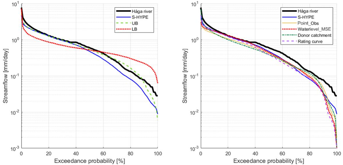
**Figure 9.** Flow duration curves for HBV-simulations. To the left the FDC of UB and LB is shown together with Håga and S-HYPE as reference. To the right the references are shown together with all calibration-methods except Waterlevel as it is essentially the same as Waterlevel\_MSE.
