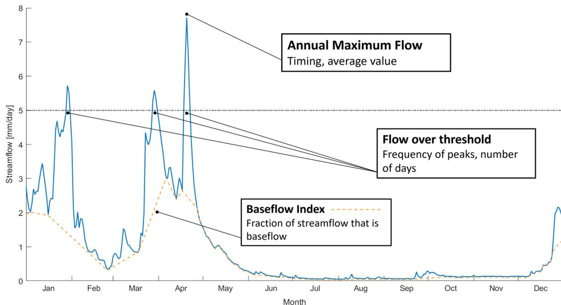
**Figure 1.** *Some examples of hydrological signatures that can be calculated from different types of data*
