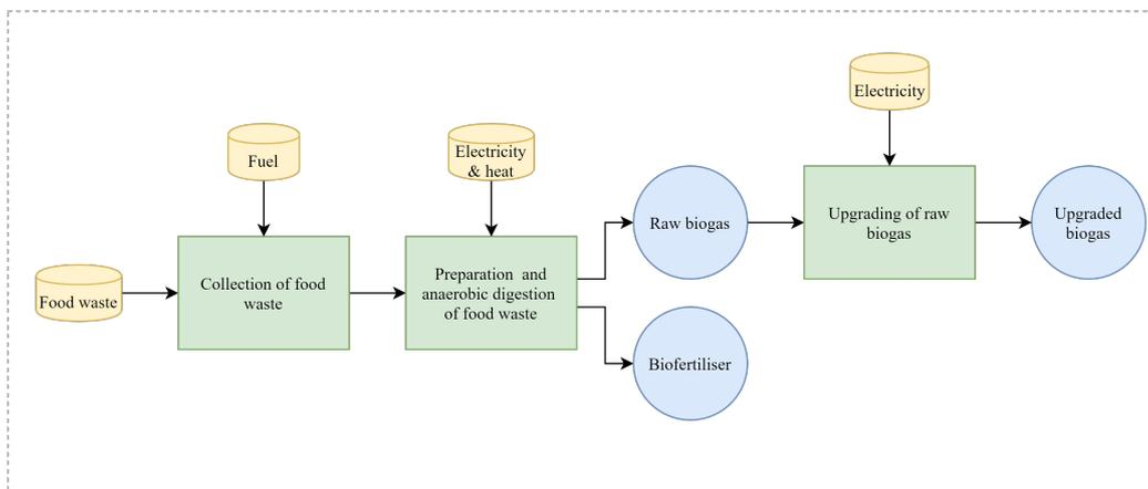
**Figure 5:** Process chart illustrating the treatment of food waste where yellow cylinders depict consumed resources, green boxes represent greenhouse gas emitting processes, blue circles represent produced resources and the dotted line show the system boundaries
