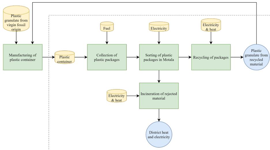
**Figure 6:** Process chart illustrating the treatment of plastic containers where yellow cylinders depict consumed resources, green boxes represent greenhouse gas emitting processes, blue circles represent produced resources and the dotted line show the system boundaries
