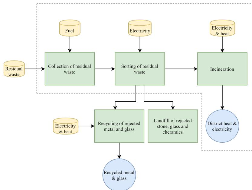
**Figure 7:** Process chart illustrating the incineration process where yellow cylinders depict consumed resources, green boxes represent greenhouse gas emitting processes, blue circles represent produced resources and the dotted line show the system boundaries
