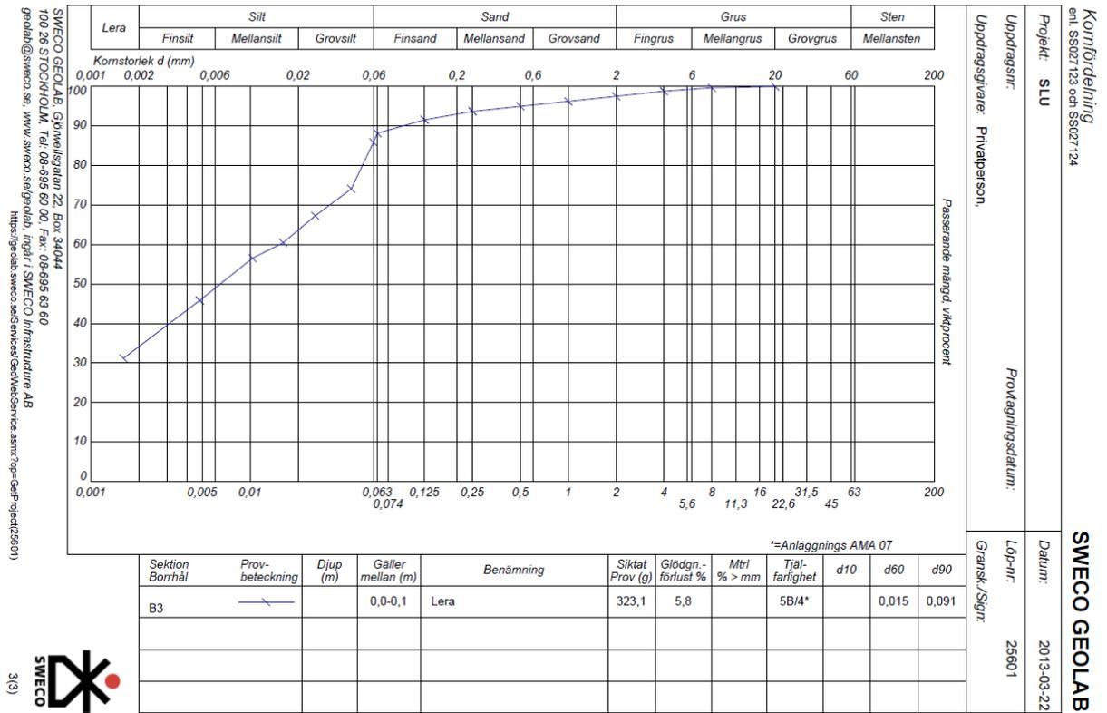
Figure A4. Sieving curve for soil B3 0.0-0.1. The soil went under the alias soil C3 in the report.
