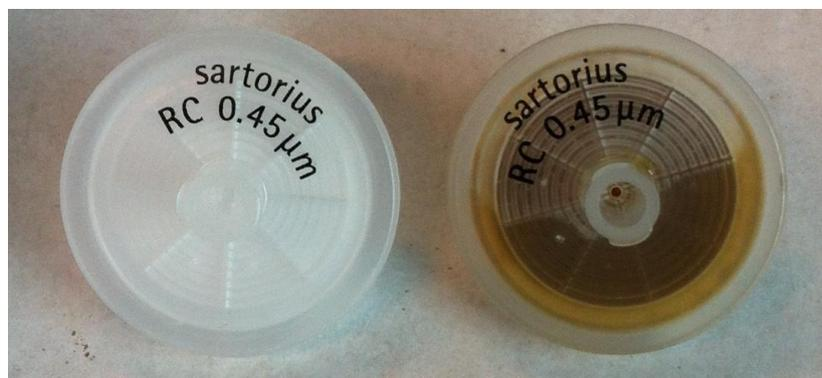
**Figure 14.** Syringe filters before (left) and after (right) filtration of one sample. Some suspended solids were stuck in the syringe filters. This might have act as a source for PFASs losses in the experiment method. These potential losses were however not measured.
