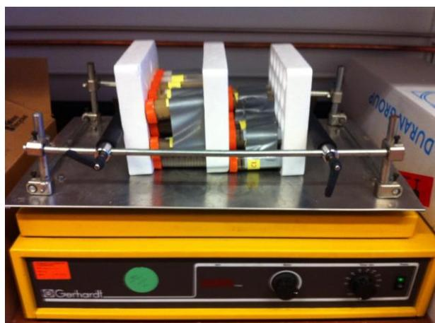
**Figure 2.** The samples were shaken on a 2D shaker at 200 rpm. The samples were removed from the shaker after 8, 24, 48, and 72 hours (spiked samples) and 48, 196, 240 and 360 hours (contaminated samples).
