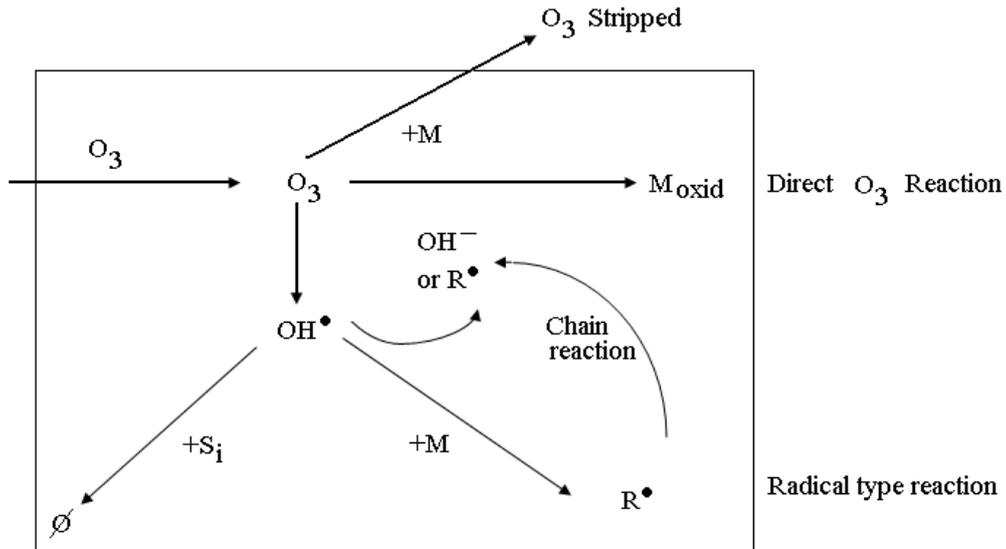
*Figure 6.* Scheme of reaction of ozone added to an aqueous solution. M=solute, M<sub>oxid</sub>=oxidized solute, S<sub>i</sub>=free radical scavenger i, Ø=products which do not catalyze the ozone decomposition, R=free radicals which catalyze the ozone decomposition (Hoigné and Bader, 1979).
