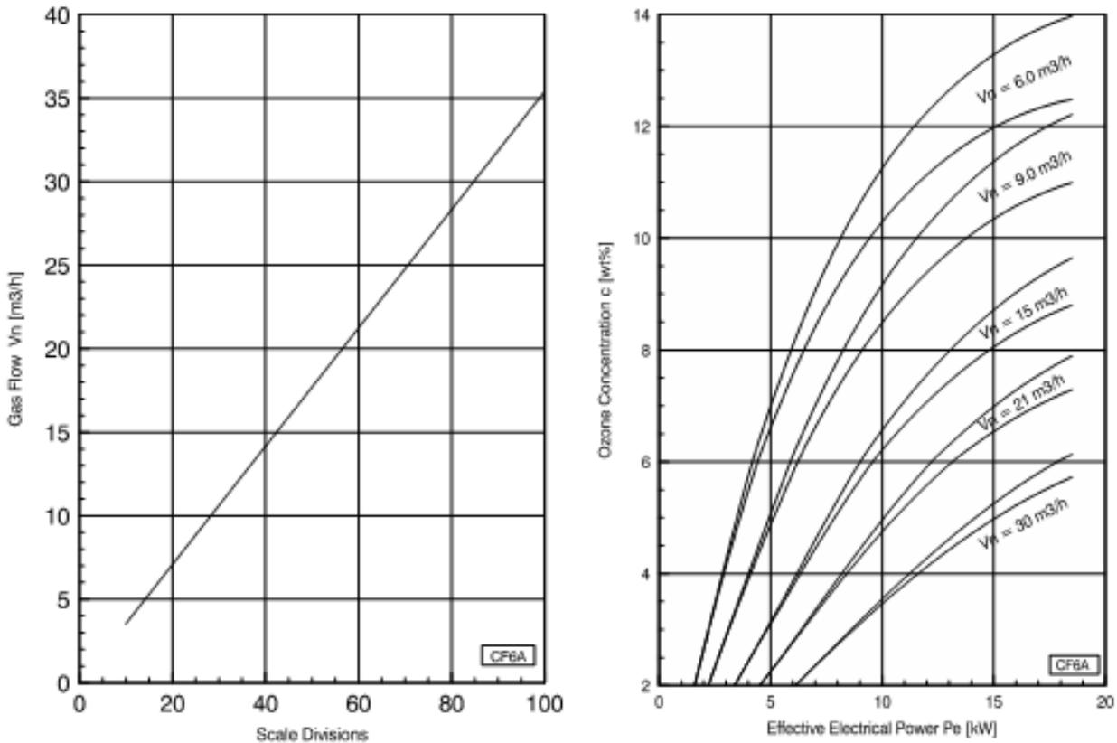
Figure 8 . Gas flow and electrical effect diagram examples for the OZAT<sup>®</sup> OZONGENERATOR TYP CF-6A.
