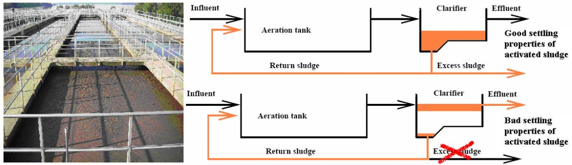
Figure 2. Bulking sludge in the clarifier, Himmerfjärden WWTP 2006.
