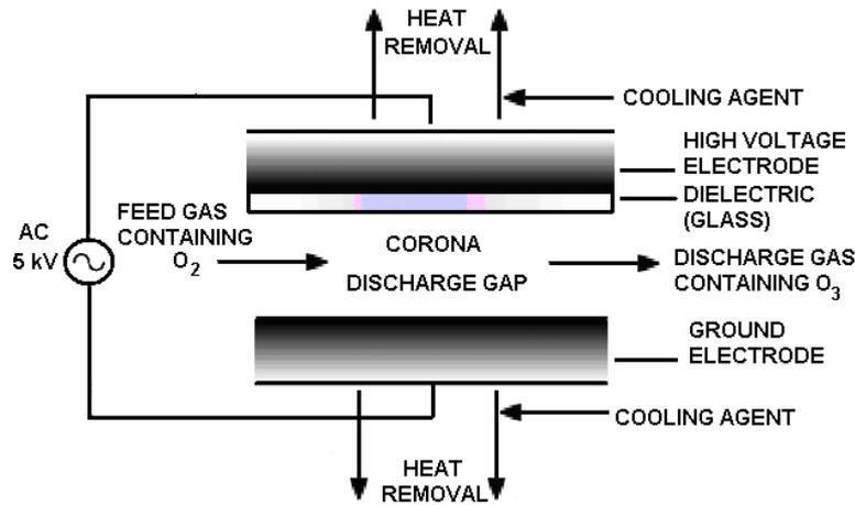
Figure 7. Principle of a basic electrical discharge cell
