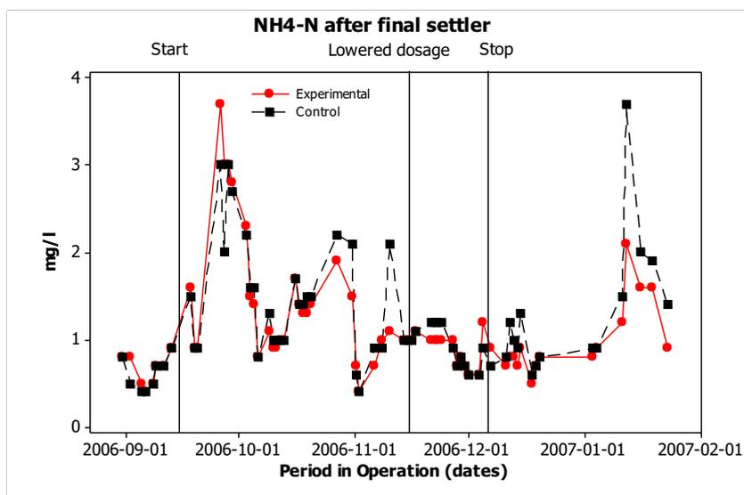
Figure 30. Ammonia in effluent of the tertiary treatment for the control and experimental line.
