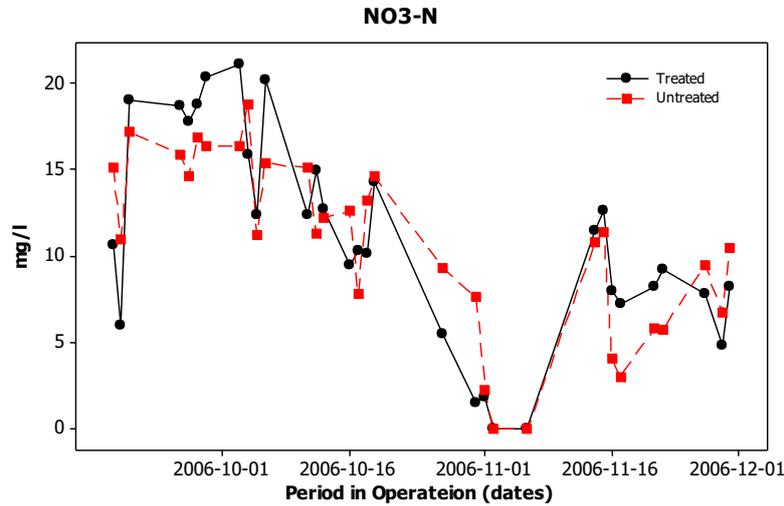
Figure 27. Nitrate ( $\text{NO}_3\text{-N}$ ) in the treated and untreated RAS in experimental line.
