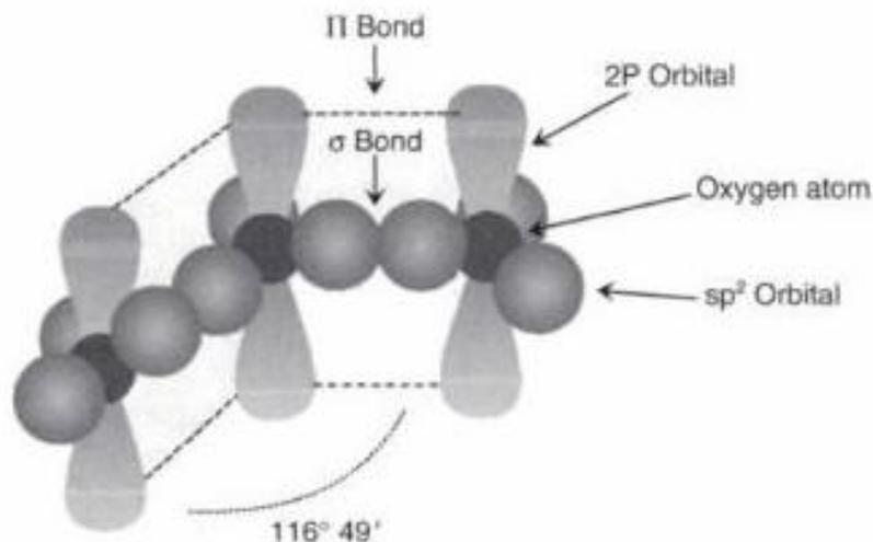
Figure 5. Structure of an ozone molecule. Figure copied from Beltran (2003)
