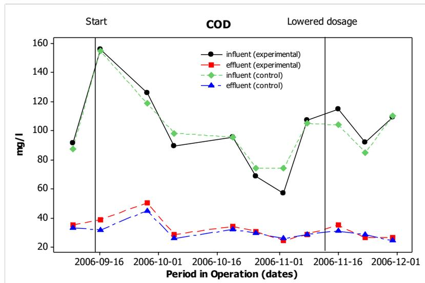
Figure 28 Influent and effluent COD values for the control and experimental lines.
