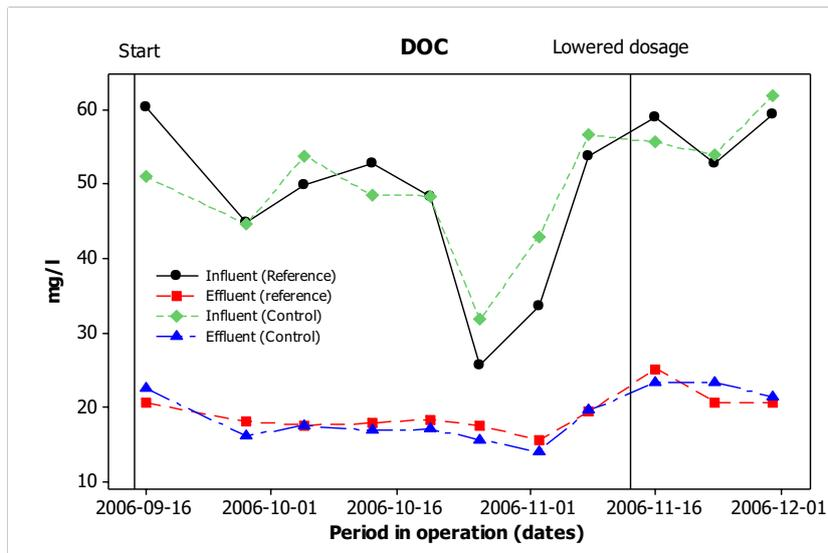
Figure 29 Influent and effluent DOC values for the control and experimental lines.
