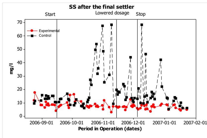
Figure 14. Suspended solids in effluent of the final settler for the control and experimental line.
