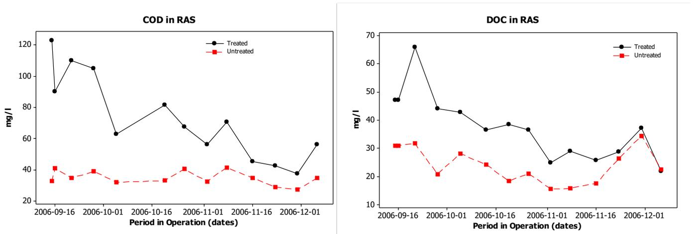
Figure 25. COD and DOC in the treated and untreated RAS in experimental line.
