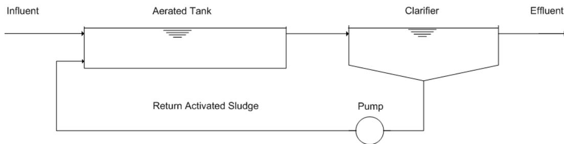
Figure 1. The activated sludge process, the waste water flow in to the aerated tank and out from the clarifier.
