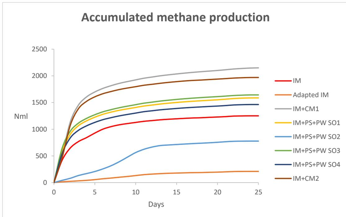
**Figure 23** The total accumulated methane production for each triplicate with the inoculum included. SO is short for scenario and describes the ratio between PS and PW. The ratios are 10.72 for SO1 and SO2, 12.45 for SO3 and 8.93 for SO4. The ratios are calculated with the VS value. Other abbreviations
