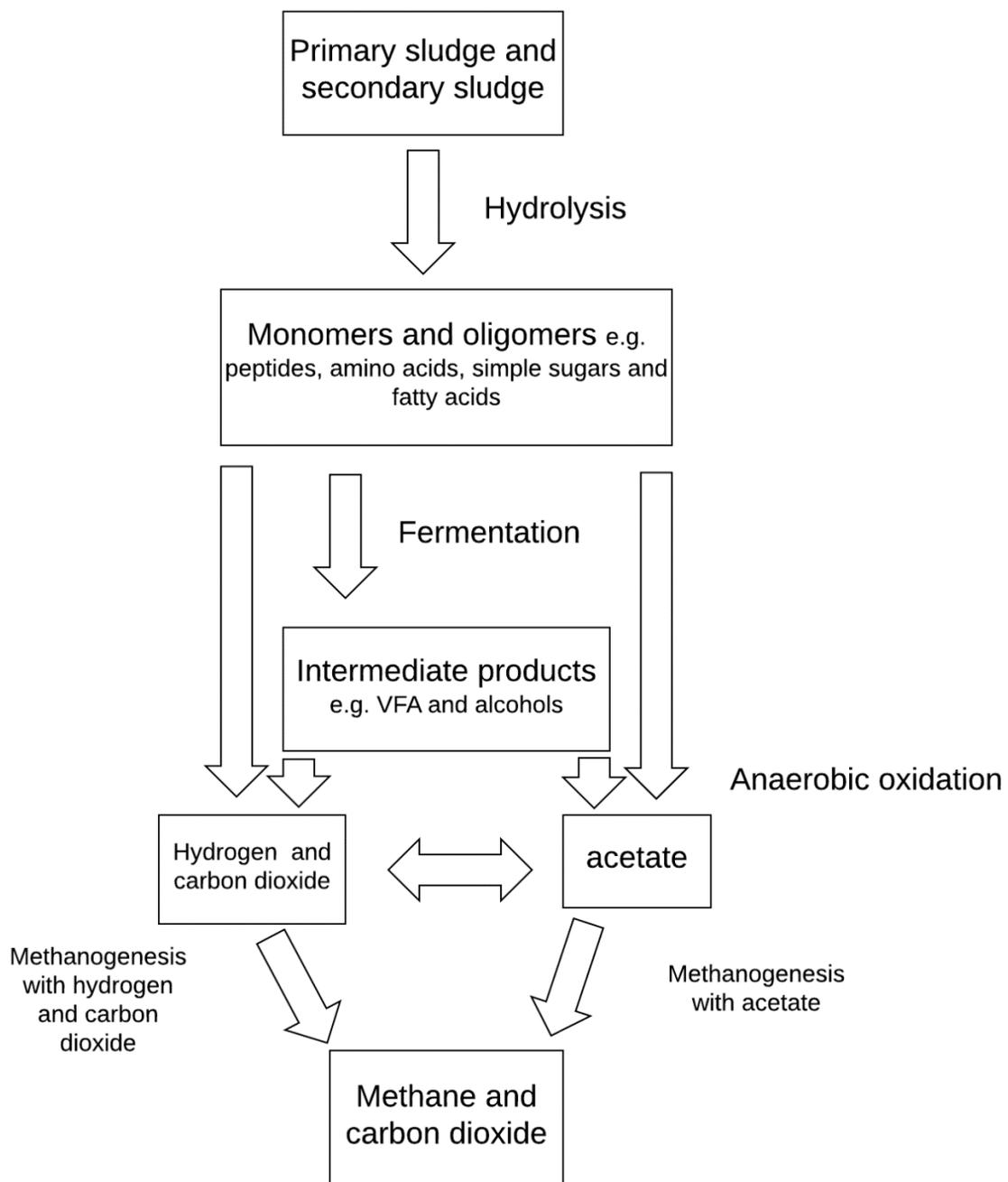
**Figure 6** Flow chart over the four degradation steps from sludge to methane in an anaerobic digester.
