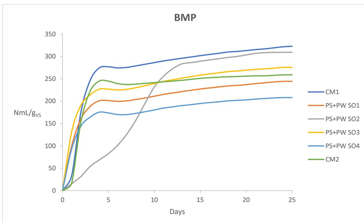
**Figure 25** The methane production for each substrate triplicate. The inoculum is excluded and added VS is considered.
