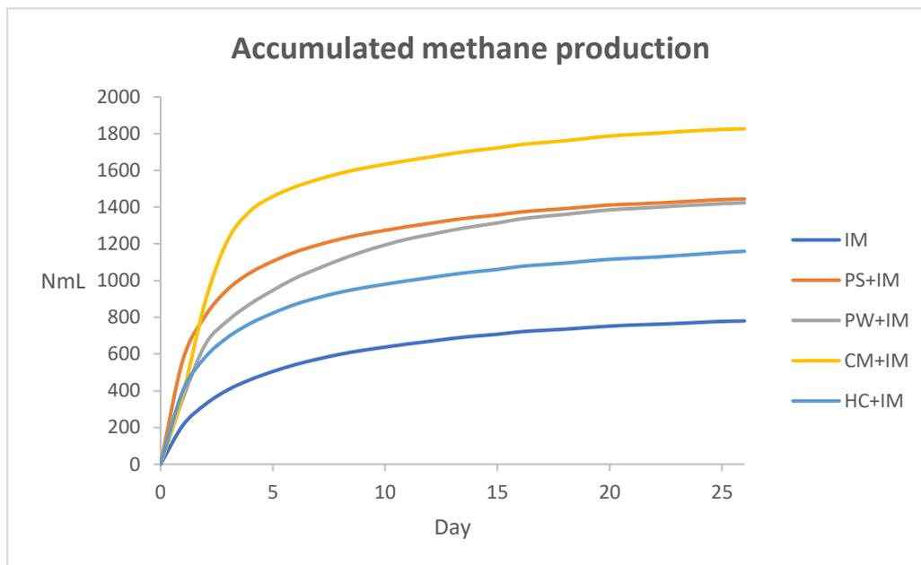
**Figure 19** Total accumulated methane production for the substrates in trial 1 together with the inoculum. IM: Inoculum, PS: Primary sludge, PW: Process water, CM: Microcrystalline cellulose, and HC: Hydrochar.
