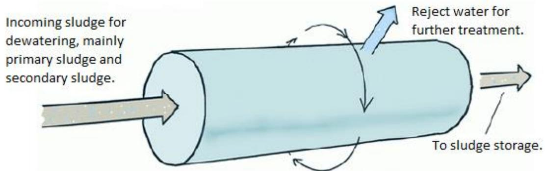
**Figure 4** Simple sketch over how a centrifuge works. The primary sludge and secondary sludge are coming in. Since the reject water and the dewatered sludge have different densities, they can be separated from each other (Kävlinge kommun, 2014).
