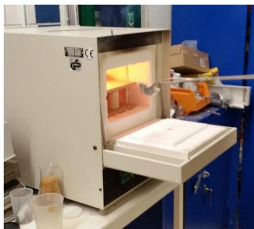
**Figure 13** Left: The samples after 2 h in 550 °C and Right: One sample on its way into the 550 °C oven.
