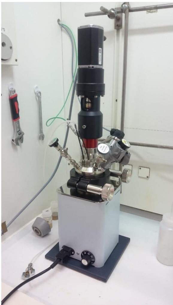
**Figure 12** The laboratory scale HTC batch reactor (Åkerlund & Sirén Ehrnström, 2017).
