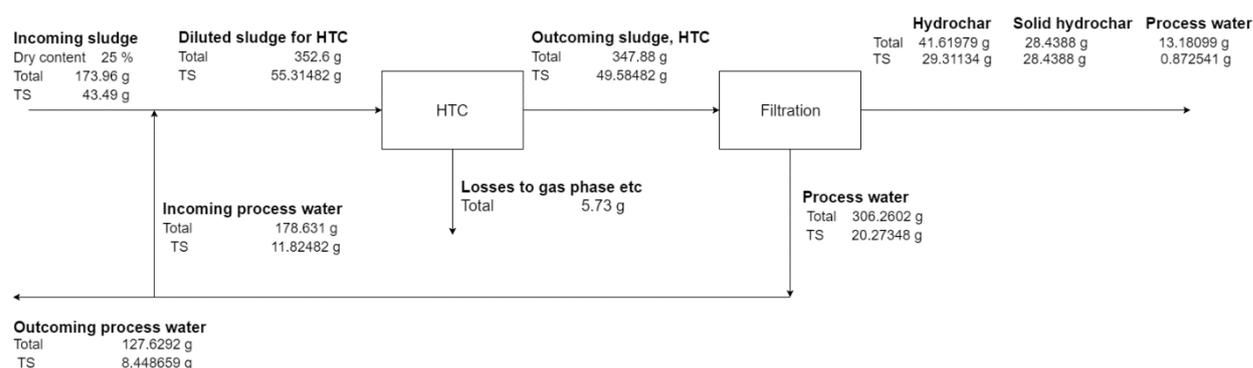
**Figure 17** Mass balance for a realistic design of the HTC process in full-scale. All values are present as total weight and as the TS amount of the total weight.
