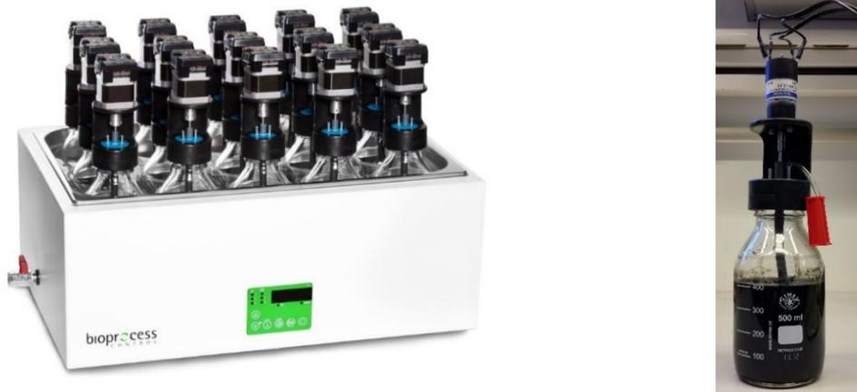
**Figure 16** Left: The sample incubation unit consisting of the water bath and the 15 vials. Right: A close-up of one vial with sample within. The red little plastic piece is a gas stop i.e. it prevent gas from leaking out (Bioprocess Control Sweden AB, 2017).
