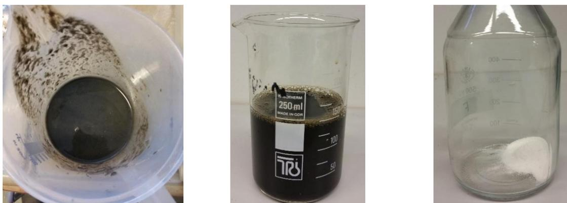
**Figure 10** Three image of three different substrates. The image to the left is primary sludge, middle image is process water and the image to the right is microcrystalline cellulose.
