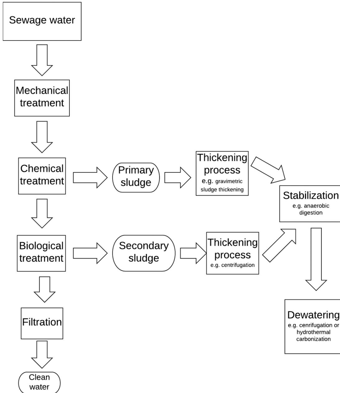
**Figure 2** Flow chart over the treatment steps in a wastewater treatment plant and what types of sludge are formed in which step. Moreover, the dewatering process of primary and secondary sludge.
