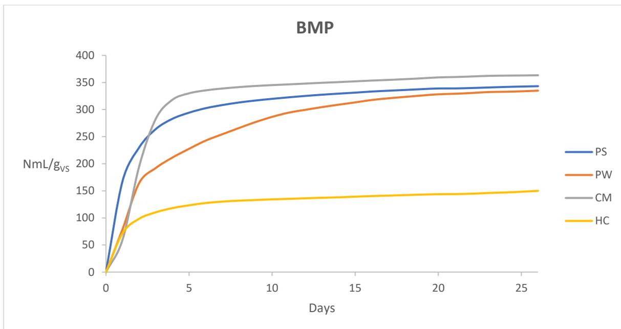
**Figure 21** Methane production for each substrate divided with the substrates' VS weight. (Methane production from the inoculum excluded).
