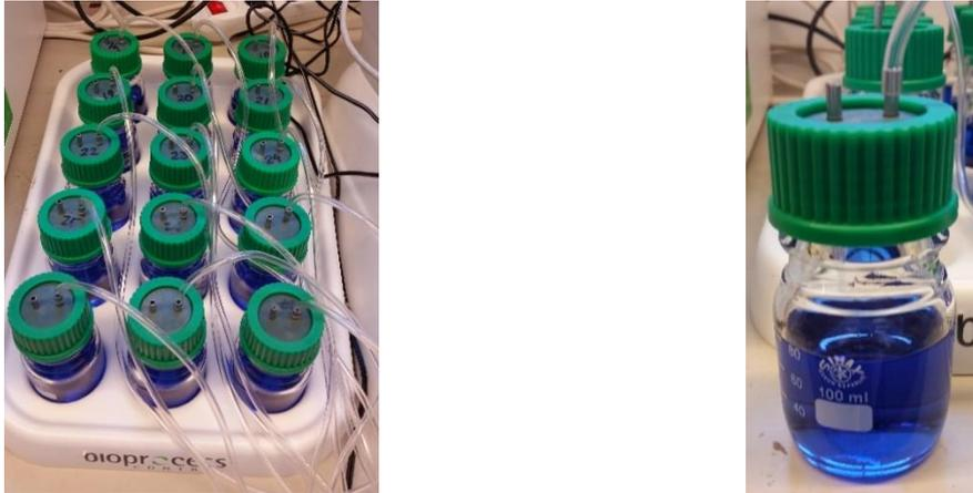
**Figure 15** Left: 15 CO<sub>2</sub>-fixation bottles placed in the bottle holder. Right: Close-up of a CO<sub>2</sub>-fixation bottle and the alkaline solution.
