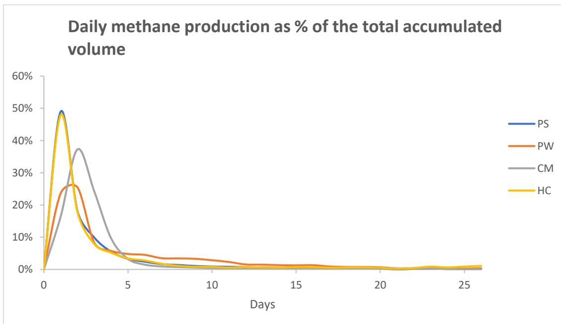
**Figure 22** Daily methane production as percent of the total accumulated volume. The graph for primary sludge is hard to see but the graph is right behind the hydrochar graph.
