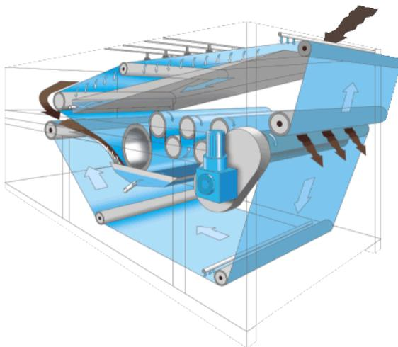
**Figure 5** Illustration of a belt filter press (Huber technology, 2017).
