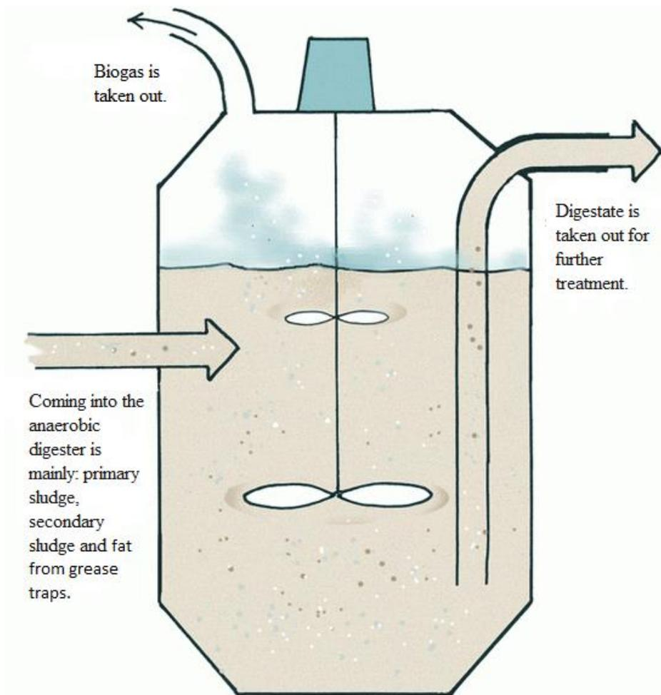
**Figure 7** Simple sketch of a CSTR. Mainly Primary sludge, secondary sludge and grease traps sludge are fed into the CSTR at Henriksdals WWTP. Biogas and digested sludge are discharged at top of the digester. It is also common with a third outlet at the bottom of the CSTR for digested sludge with high density (Kävlinge kommun, 2016).
