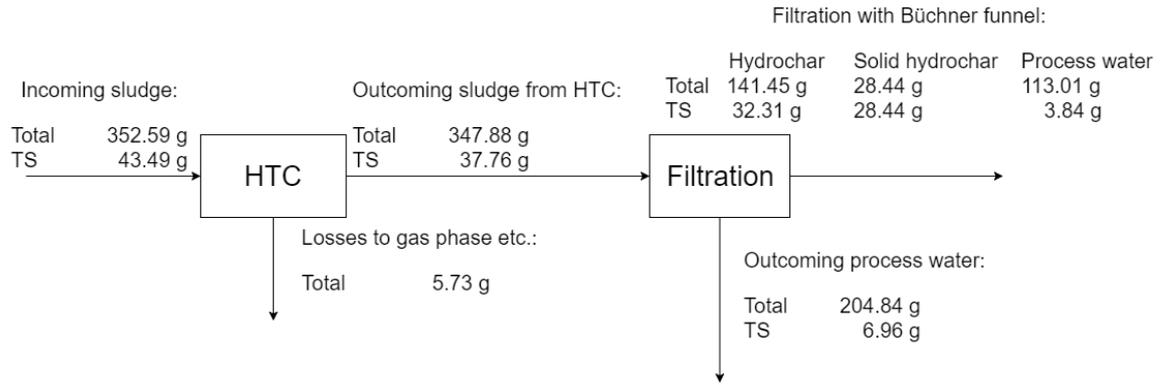
**Figure 18** Modified figure from C-Green (Öhman, 2017b). The dewatering ratio (by weight) between outcoming process water and incoming sludge has been changed from approximately 70 % to approximately 58 % to better replicate the conditions in this master thesis.
