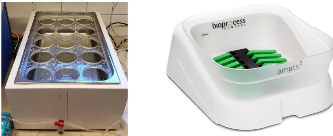
**Figure 14** Left: The water bath. The temperature in the water bath could be regulated, during the trials the temperature was set to 37°C. The water bath was constructed with 15 holes, where the vials could be placed. Right: Gas measuring device, when enough gas has entered under the green flaps, they are lifted and the released volume is registered (Bioprocess Control Sweden AB, 2017).
