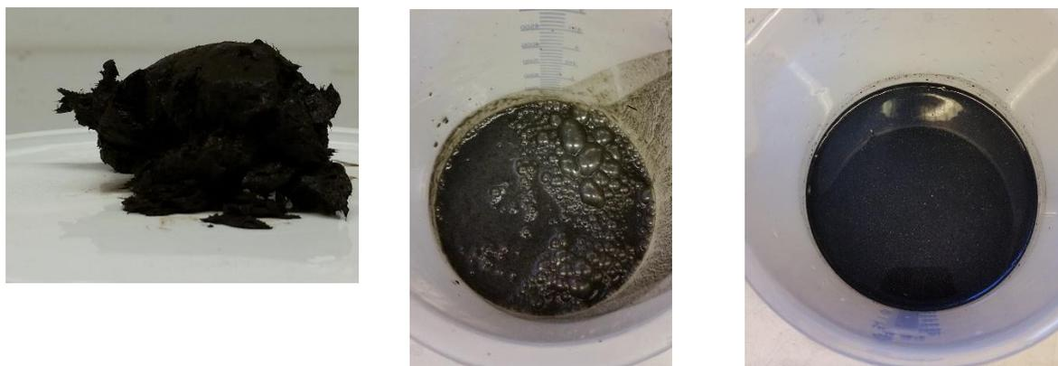
**Figure 11** Two substrates and one inoculum. The image to the left is hydrochar, the middle image is ordinary inoculum from Henriksdals WWTP and the image to the right is adapted inoculum.
