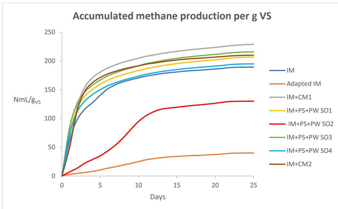
**Figure 24** The total accumulated methane production divided with the added amount VS weight. The inoculum is included.
