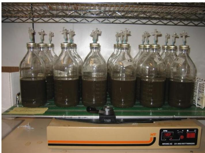
Figure 5 Batch bottles (1 l) on a shake table in a constant temperature room. Photo taken by Erik S. Moglia, 2007.
