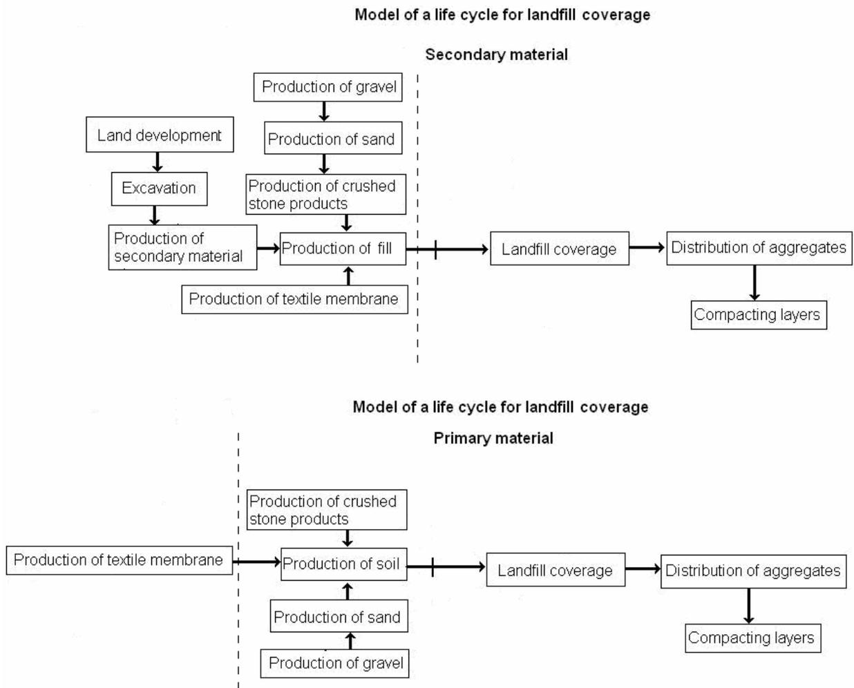
**Figure 4.2** Life cycle model structure for landfill coverage. Upper part represents Case 1, where secondary material was used. Lower section represents Case 2, in which virgin material was produced to function as fill. Intersected arrows indicate transport. Dotted lines show system borders.
