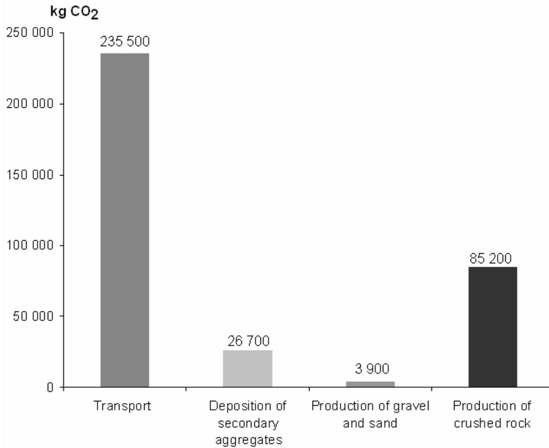
**Figure 4.8** Emissions of CO<sub>2</sub> from each process in the Case 2, where only virgin materials were used.
