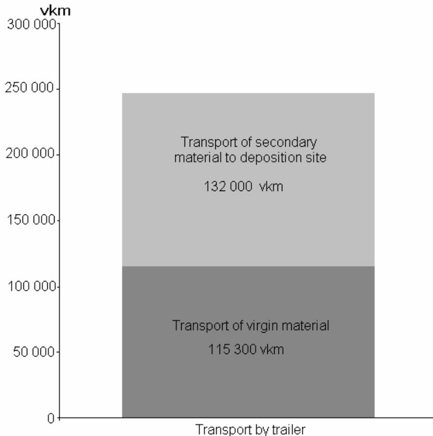
**Figure 4.6** Contribution to total amount of vehicle kilometers from transport of discarded aggregates and virgin material, respectively, in *Case 2*.
