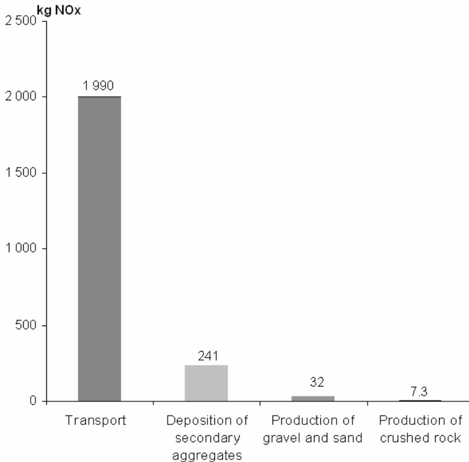
**Figure 4.11** Emissions of NO<sub>x</sub> as contributed by each process in Case 2.
