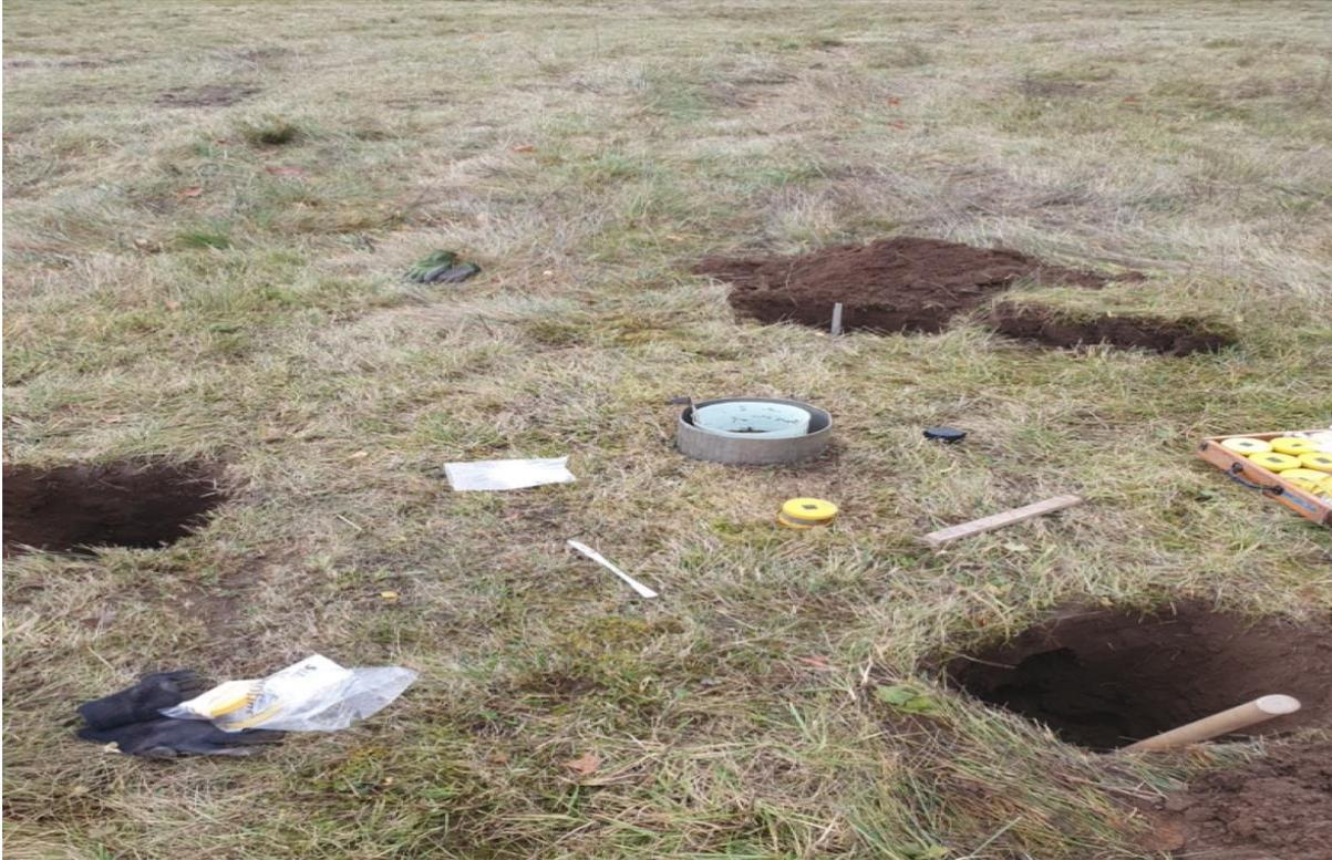
FIGURE 5: EXPERIMENTAL SETUP ON SITE 2, DOUBLE RING INFILTROMETER CAN BE SEEN IN THE CENTRE OF THE PHOTO, THE YELLOW CYLINDER BELOW WAS USED TO TAKE SOIL SAMPLES
