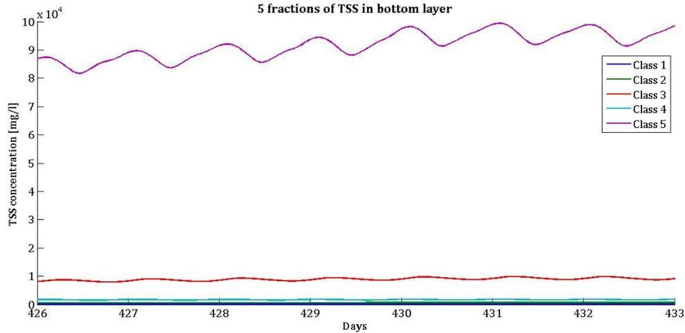
Figure 20. The five fractions of TSS in the bottom layer, evaluating simulation results from the first week of July.
