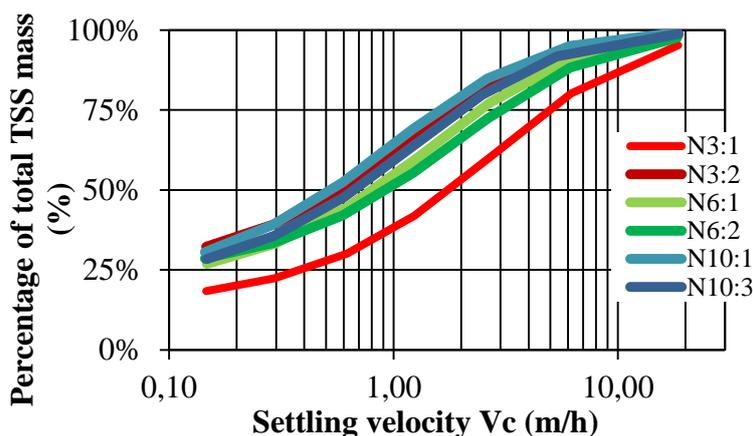
Figure 9. The resulting ViCA's curves in three cases when the dilution was made the same in Column 1 and Column 2 in order to evaluate the effect of storage time.
