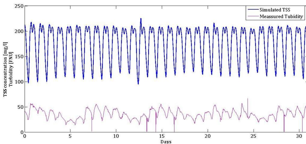
Figure 19. Online measurements of turbidity and simulated concentrations of TSS in the primary effluent during the month of July.
