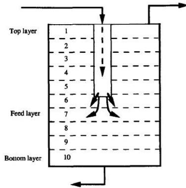
Figure 3. Layered settling model of 10 layers (after Takács et. al., 2001).
