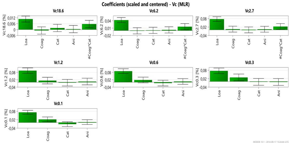
Figure 14. The coefficient plot of the factors describing each settling velocity, terms are scaled and centered to enable comparison of the impact by each term.
