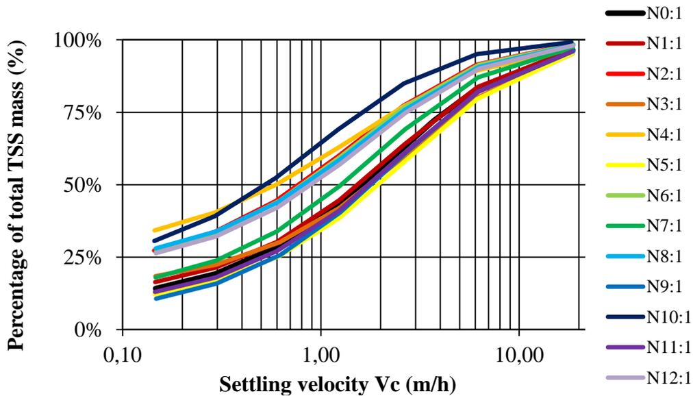
Figure 11. The settling velocity distribution, ViCA's curves, attained from Column 1. The top cluster of curves represent the afternoon samples and the bottom cluster of curves the morning samples.
