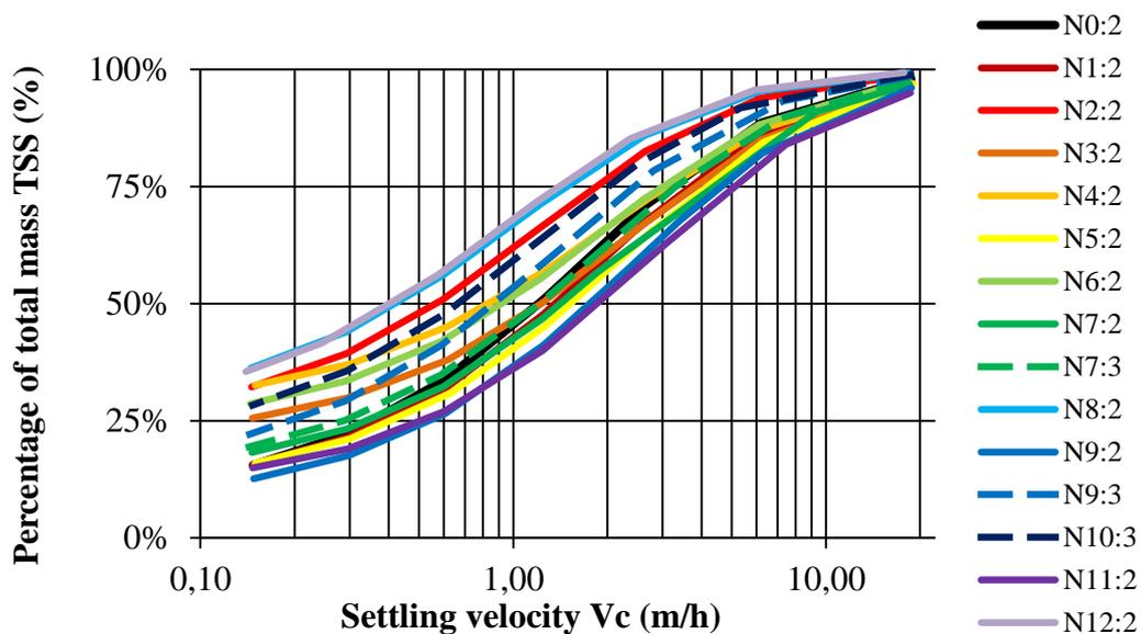
Figure 10. The settling velocity distribution, ViCA's curves, attained from Column 2. The top cluster of curves represent the afternoon samples and the bottom cluster of curves the morning samples.
