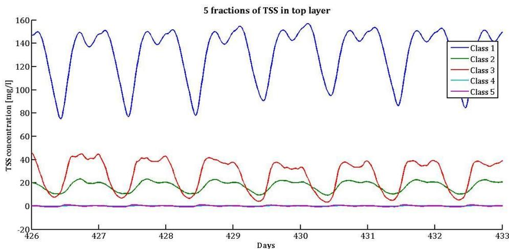
Figure 21. The five fractions of TSS in the effluent, evaluating simulation results from the first week of July.
