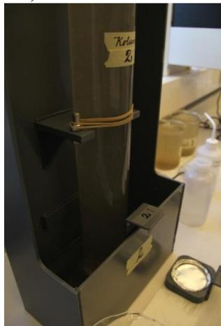
Figure 5. A cup was placed under the column, collecting the settled particles. *Photo: Emma Lundin*
