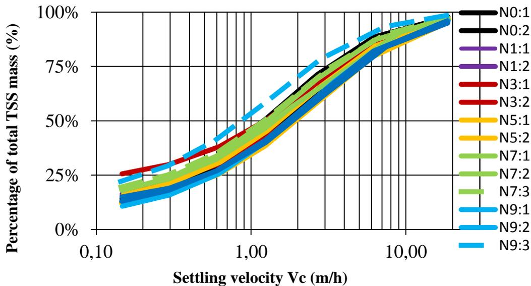
Figure 7. The ViCA's curves,  $F(v_s)$ , gathered from the morning samples with altering dosage of chemicals, compare with These criteria meet the recommendations for screening purposes (Umetrics. 2001). Therefore. a test chart was developed after  $2^{4-1}$  FFD with four
