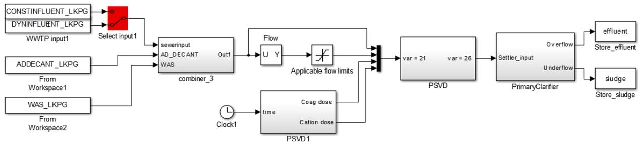
Figure 17. The model of the primary clarifier based on particle settling velocity distribution, presented in Simulink.
