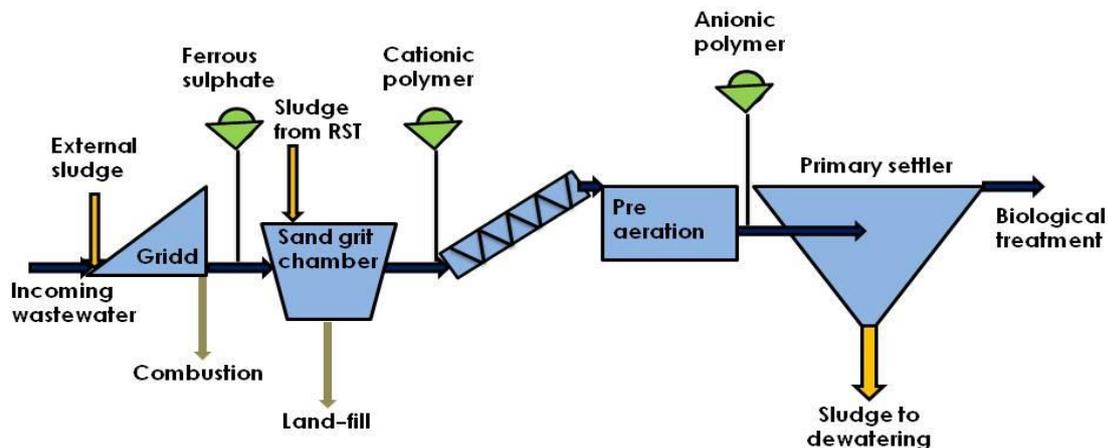
Figure 1. The mechanical treatment step at Nykvarn WWTP. (Tekniska Verken, 2013).
