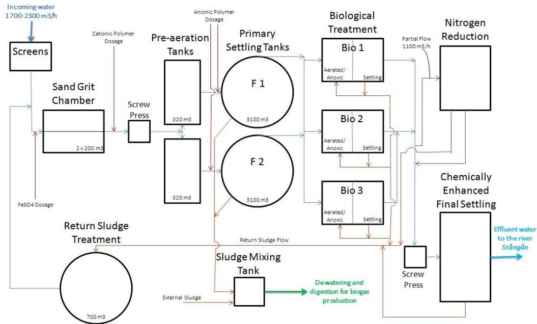
Figure 2. Nykvarn's WWTP has two primary clarifiers. Here seen as the round tanks of 3100 m<sup>2</sup> each. The figure does not display the sludge treatment steps including the Sharon tank.
