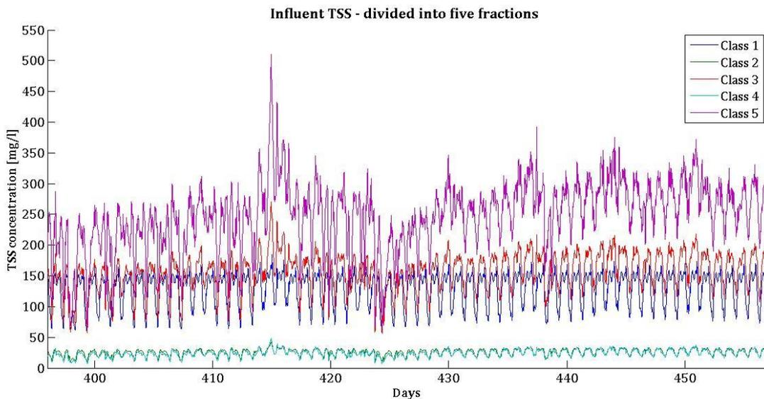
Figure 16. Simulated influent data for June and July, after TSS division in the PSVD function.
