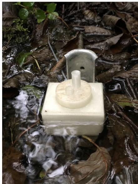
*Figure 11: An EC-trap installed in a stream.*
