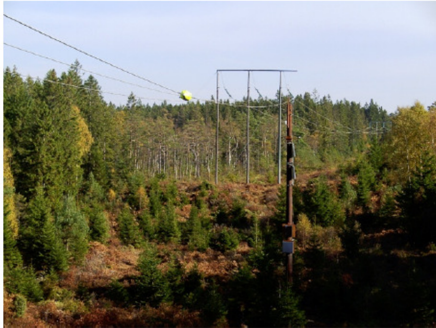
Figure 3.1: The measurement system Cordinas installed on the line and the weather station on a pole beside the line
