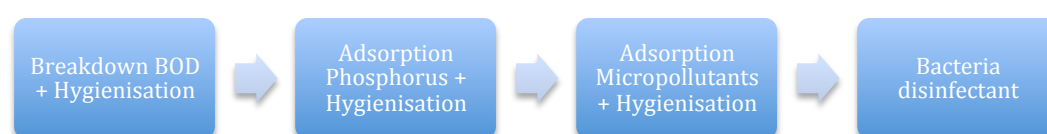
Figure 3. The functional flow of the sandbed filter with Polonite and GAC add-on filters, as well as disinfection of bacteria with a UV lamp.
