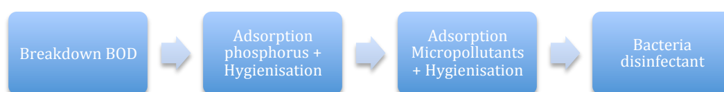
Figure 5. The functional flow of the package treatment system with Polonite and GAC, which is called BIOP. Package treatment systems often contain disinfection of bacteria with a UV lamp.
