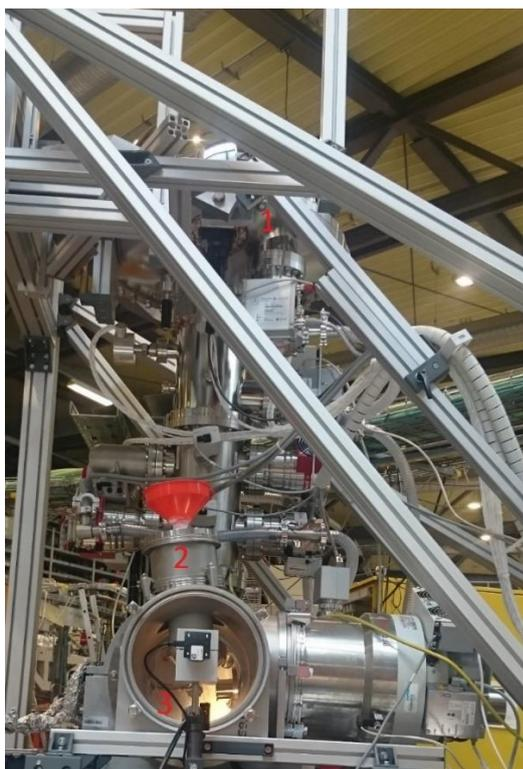
Figure 4. The experimentation station. 1 is the analyzer, 2 is one of the three cold traps, 3 is the chamber with the water jet
