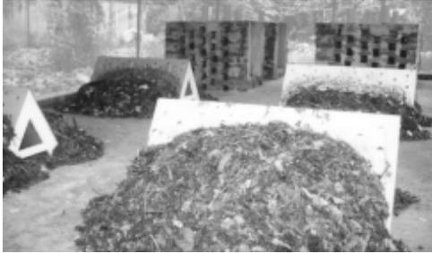
**Figure 3** Waste piled onto and around triangular aerators as it can look in Bangladesh (Rothenberger & Enayetullah, 2006).
