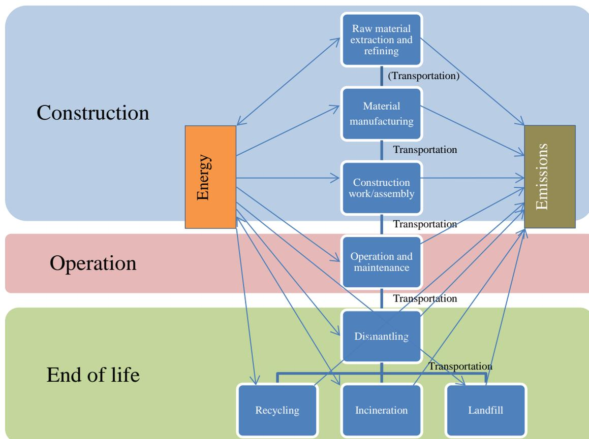
**Figure 5.** Flow chart of sub model illustrating the different steps and phases of the life cycle. This example is for the track sub model.
